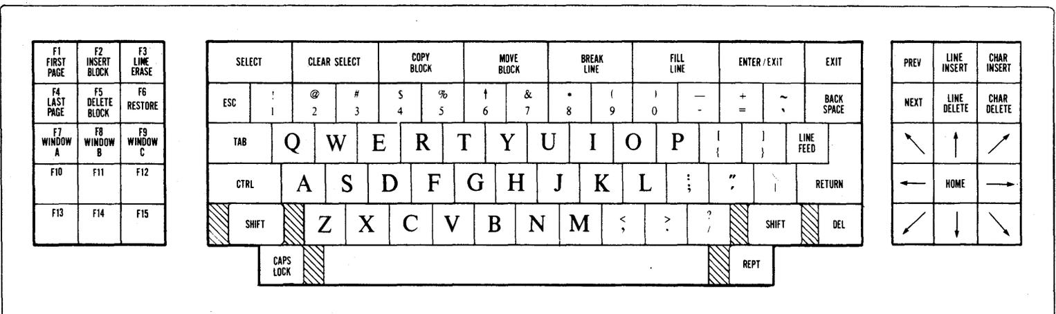
Figure 5. Monochrome Display Keyboard
