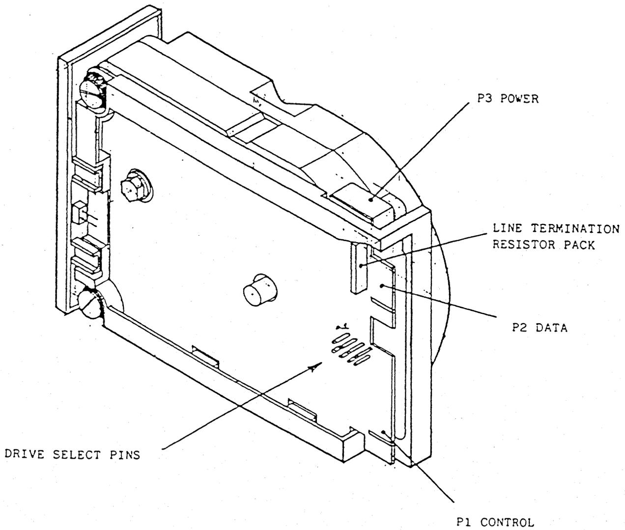
FIGURE 2 : CONNECTOR AND DRIVE SELECT PIN POSITIONS
