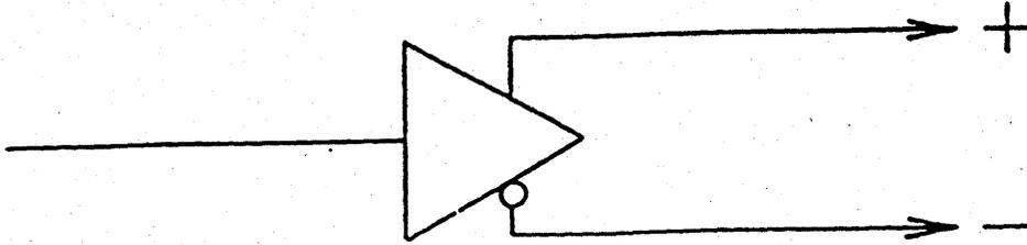
FIGURE 9 : RS 422 DIFFERENTIAL LINE DRIVER
