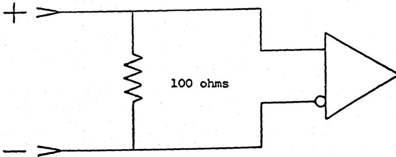
FIGURE 10 : RS 422 DIFFERENTIAL LINE RECEIVER
