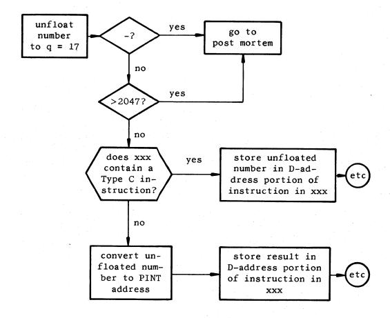
As a result of the structure of PINT memory, some instructions are limited. For example, jCXI may not be used to modify count-type (Type C) instruction. This could have been allowed only by approximately doubling the operation time.
