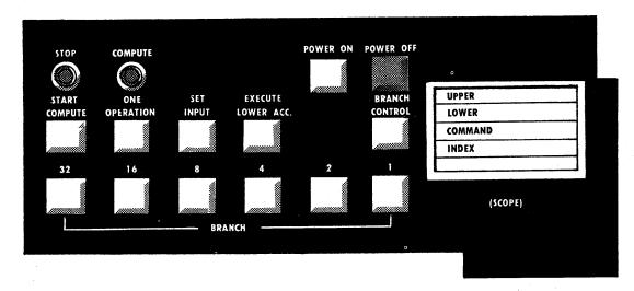
Operational control of the computer is effected through the control panel of the 4010 computer. The location, arrangement, and components of this panel provide operator convenience in system control and supervision.
