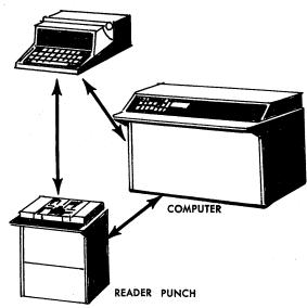
All units switched to OFF-LINE state are automatically interconnected, for example:
