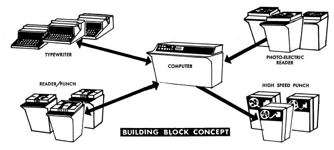
As many as 45 input and output units may be connected on-line simultaneously and, with minor modifications, up to 60 devices may be connected.
