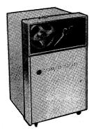
The High Speed Punch is capable of perforating paper tape at the rate of 300 characters per second. It is designed for ON-LINE operation with (and under control of) the 4010 computer.
