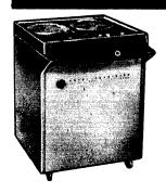
The model 4410 Photo-Electric Reader is a high-speed "input" device for the RPC-4000 computer. Capable of reading punched paper tape at 500 characters per second, this unit is separately packaged in a matching cabinet which provides tape-handling facilities. Tape may be sensed in forward or reverse direction with equal ease. Also, tape may be searched for a special code in either direction while the computer accepts input, emits output, or computes.
