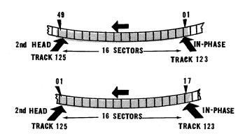
One dual-access track has two read-write heads located 16 sectors apart with each separately addressed. Heads 123 and 125 are on this same track, but head 125 is 16 sectors "behind" 123; that is, a word will pass head 123 first then pass head 125 exactly 16 word-times later. Thus, any word on this track may be retrieved by either head. For example, Word in 12300 = 12516. Word in 12301 = 12517.
