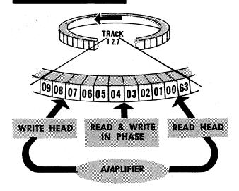
There is one track on the drum devoted to HIGH SPEED (access) storage. This is called an "eightword high speed line," since eight words of information are duplicated eight times, and has a track address of 127. The sector address is modulo 8, thus sector designations 0, 8, 16, 24, ... 56 all apply to the same word.
