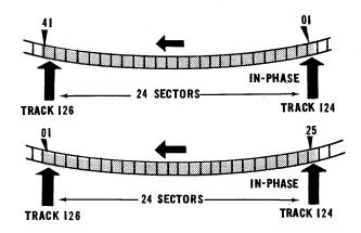
In each case, the lower numbered head is called the "reference" head because it is in phase with main-memory.
