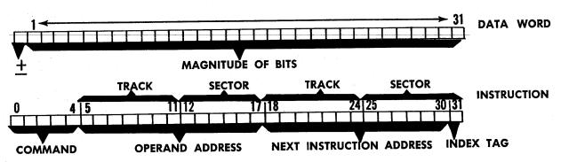
Data transfer is usually accomplished in one-word units. However, part of a word may be extracted and/or operated upon in certain instances at the discretion of the programmer. In addition, multiple words may be transferred in the repeat mode of operation.
