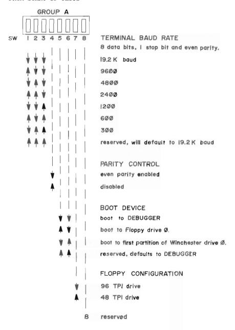
Note: For normal operation, the PROMs require that switch 8 of the Group-A DIP switch be set off (down). Switch 8 is used to cancel the memory test or select various maintenance and debugging options on startup.
