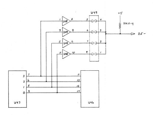
MOD TO ALLOW ADDRESS ING FIRST 128K TO CHUSE BUSS ERROR
