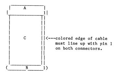
Line up the crimping pins of each connector with the wires in the cable and press fit to the cable.
