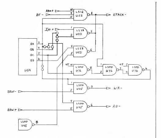
MOD TO ALLOW EXTRA DATA HOLD TIME FOR SLOW PERIPHERAL CHIPS
