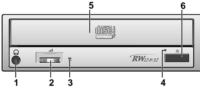
1. Connector for stereo headphones with a 3.6 mm stereo mini-jack
