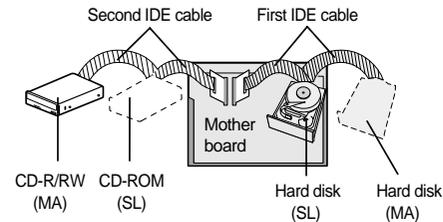
Install the jumper in the MA position (Master).
