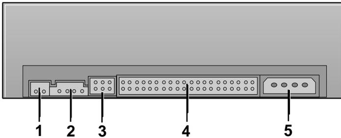
1. Two-pin digital audio output terminal for use with a sound or MPEG card supporting digital audio features
