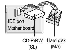
Install the jumper in the SL position (Slave).
