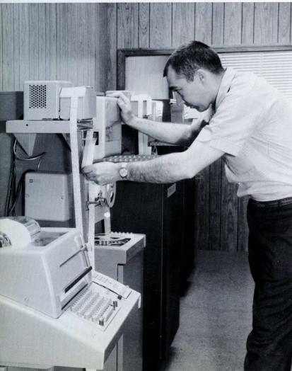
Exceptional simplicity is the key to Sanders 5700 System. Data can be entered via a typewriter-style keyboard in a typical low-noise office environment. Once the displayed data is verified, it is then sent, via the keyboard, to a punch which can be located up to 1000 feet from your office.
