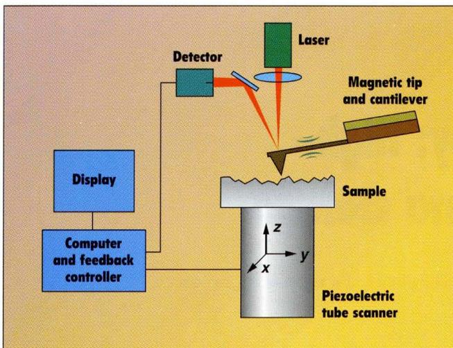
**Figure 2.** Schematic of a scanning probe microscope (MultiMode design). For magnetic imaging, the probe has a magnetic tip. The sample is moved in a raster pattern by the piezoelectric scanner, and the sample's stray fields cause shifts in the resonance of the cantilevered probe that are measured by laser detection.
