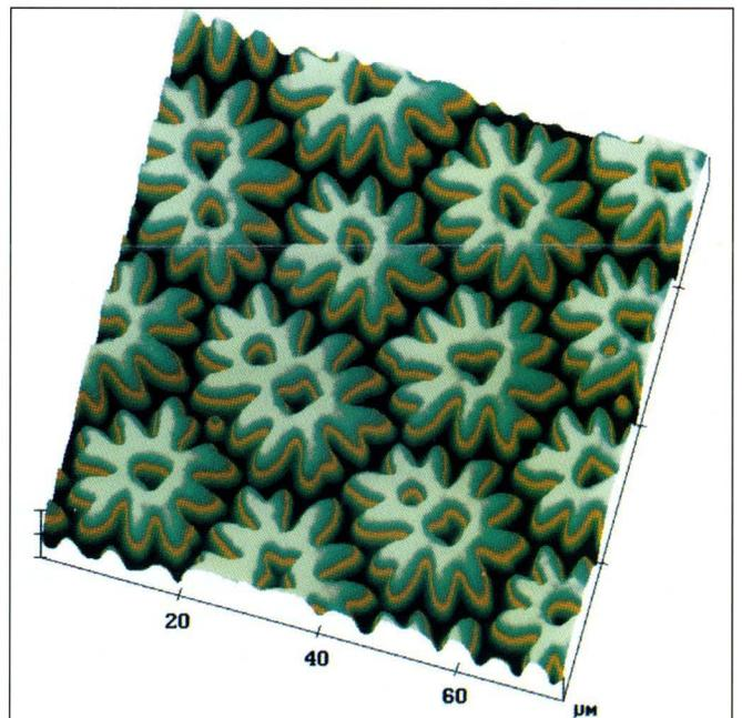
Figure 9. MFM reveals picturesque "flower" domains in a 60- $\mu\text{m}$  garnet film used in magneto-optic isolators. Similar garnet films are also used for magnetic bubble memories and are proposed for data storage devices based on micromagnetic structures (Bloch lines) at the walls of bubble domains. (Sample courtesy of Vincent Fratello and Raymond Wolfe, AT&T Bell Laboratories.)
