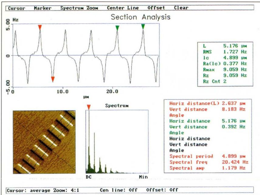
Figure 5. Section analysis of a hard disk track. The magnetic signal (top) is an average across the rectangular box centered on the track (lower left). Also shown are the power spectrum and various statistical measures of the magnetic signal.
