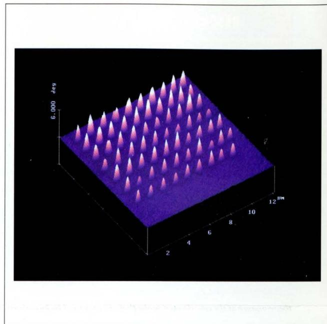
**Figure 11.** Bits written on TbFeCo magneto-optical media with a thin-film MFM probe. The same probe was used for imaging. The total applied field was decreased in successively nearer rows until no bits were written, giving a measure of the media's point coercivity. Sample courtesy of William Challener, 3M Corp.
