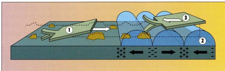
**Figure 4.** Magnetic imaging using LiftMode. For each scanline, the surface topography is first determined with TappingMode, in which the tip lightly taps the sample (1). The tip is then raised to the lift height (2), and a second pass is made to acquire magnetic force data (3) while keeping the tip-to-sample spacing constant.
