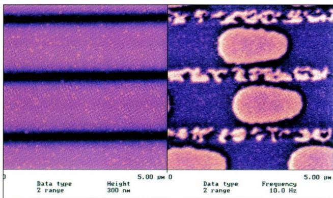
Figure 6. Bits on a magneto-optical disk. The left image shows surface topography with the tracks delineated by grooves. The magnetic force image on the right used LiftMode (lift height 35 nm). Bit edge roughness is visible, as is the virgin domain structure in the grooves (with features as small as 50 nm).
