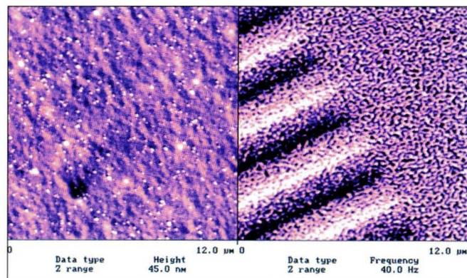
Figure 7. Track edge on metal-evaporated recording tape. Lubrication nodules and surface structure are visible in the topography image (left). The magnetic force image (right) used a lift height of 30 nm, and shows how the bit transitions are related to the virgin magnetic structure.
