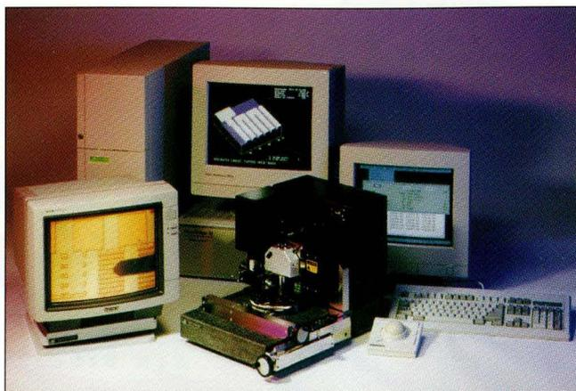
**Figure 3.** The advanced MFM imaging system used to produce the images in this article includes the Digital Instruments NanoScope III SPM controller and a Dimension 3000 atomic-force/magnetic-force microscope. Also shown are the computer and displays used for real-time video, system control, and signal processing.
