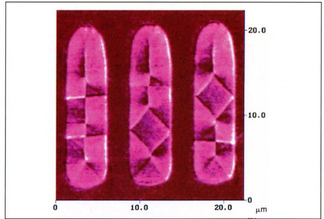
Figure 8. Magnetic domains in three topographically identical regions of 50-nm Permalloy ( $\text{Ni}_{80}\text{Fe}_{20}$ ) film. Magnetically "soft" materials such as Permalloy are widely used in such components as magnetic recording heads.
