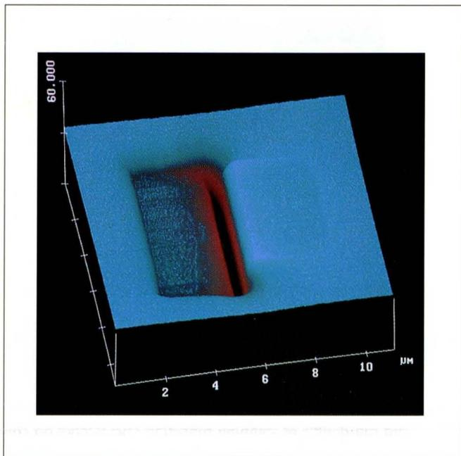
**Figure 10.** Magnetic force gradient map of fields from an active inductive head; lift height 50 nm. The magnetic gap appears as the sharp color change between the pole tips.
