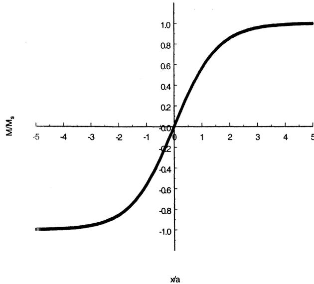
At the transition in a thin film media, magnetization flips directions. In real transitions, the flip in direction of magnetization has some finite width over which the direction of magnetization changes.
