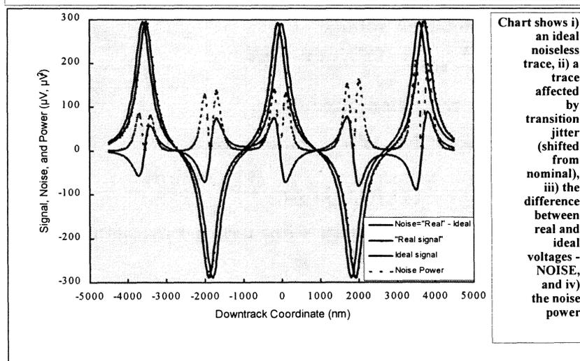
Chart shows i) an ideal noiseless trace, ii) a trace affected by transition jitter (shifted from nominal), iii) the difference between real and ideal voltages - NOISE, and iv) the noise power
