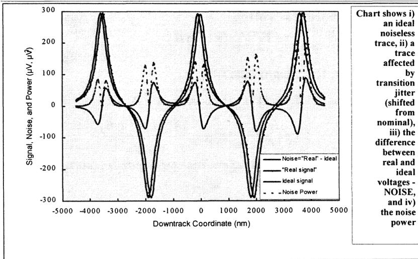
Chart shows i) an ideal noiseless trace, ii) a trace affected by transition jitter (shifted from nominal), iii) the difference between real and ideal voltages - NOISE, and iv) the noise power
