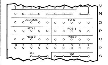
The symbol hubs are wired to the Code Lines to "set up" each code that will be used for a symbol or function. Symbols with common "bits" in their configuration are wired in common.
