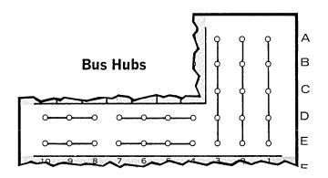
The hubs connected by lines are common terminals used to simplify the wiring of the board. All wires plugged to a given BUS hub series will be common.
