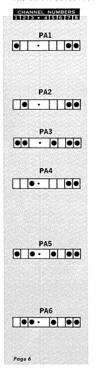
Alerts the Processor for an external entry (an entry from keyboard or reader). Whenever the PA1 code is read (with Code Control "ON") Field Control tracks 7 and 8 will be activated.
