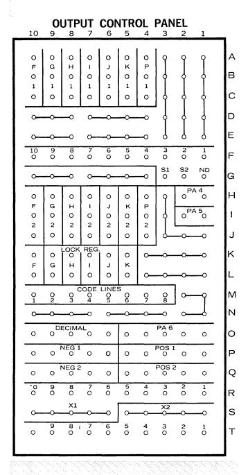
The removable Output Program Panel is recessed behind a door located on the left front side of the Processor. This panel is used for providing output signals and is not related in any manner to Processor input. There are eight primary sections to the output Program Panel. These sections are programmed by interconnecting specific hubs as prescribed by output requirements. The following information describes in detail the programming for each Output Control Panel section.
