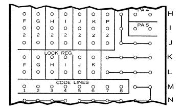
The LOCK REG section is used for *locking* selected registers such that their contents cannot be cleared by the CLEAR STORAGE/RESTORE key operation. When locked, each selected register (F, G, H, I, J and K) will retain the accumulation unless transferred out by a PA3, 4 or 5 sequence.
