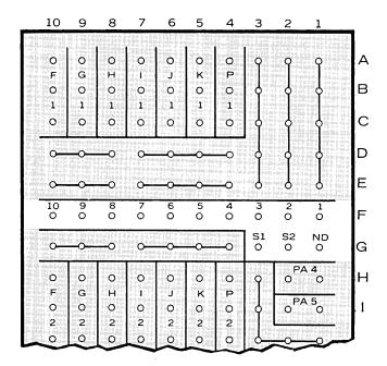
Positions F 1-10 and G 1-3 are used to indicate the order of start, decimal, stop (and when required "no decimal") of each register and register split. Appropriate register hubs are wired to these hubs to indicate the desired field output for each register. The S1 and S2 hubs indicate the first and second symbols available for signs and branching. The ND must be wired when no decimal is used for specified registers. The numbers (10 through 1) correspond with the output orders for the registers.
