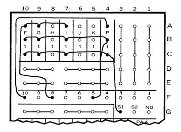
In the example above the F, G, and I Registers are wired to start at order eight, print the decimal at 5 and stop before the first symbol. The Product Register is wired to start at order 10, print the decimal at 5 and stop before the first symbol. Note that "common" hubs are wired together with multiple jumper wires. When desirable, the BUS hubs may be used for connecting hubs in common.
