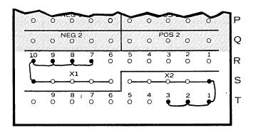
In the example shown, X1 is wired to transfer the first four digits (10-7) of a register as zeros while X2 is wired to transfer the last three (3-1) as zeros. Both X1 and X2 are selected with a PA4 sequence, but the digit 2 must also be included to select the X2 level.
