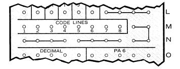
Eight hubs (M 3-10) designate the eight channels of the TYPETRONIC systems code. When the Decimal, PA6, NEG 1 and 2 or POS 1 and 2 are used, these Code Line hubs are wired to the specified code for each function.
