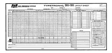
The 7816 layout sheet is provided to "put on paper" the essential requirements for the Program. The sheet is divided into six primary sections: PRINTER LAYOUT, FIELD CONTROL, INPUT ORDER ASSIGNMENTS, REGISTERS, OUTPUT CODE ASSIGNMENTS and OUTPUT CONTROL PANEL.
