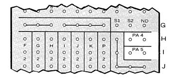
The PA4 and PA5 hubs are wired when either or both functions require *retention* of an output factor in the initiating register. If this connection is not made, the selected register will clear on PA4 or PA5 output.
