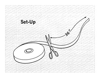
Cut off a strip of fibrous tape about 36" in length. This should be done with scissors, since creasing or folding is to be avoided. Place the tape in the punch and blank feed three or four inches until the feed punching is consistent.
