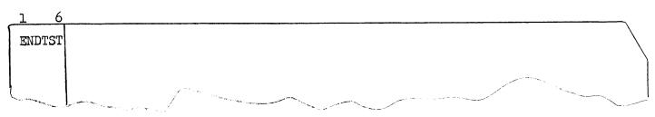
End-of-Tape Card - This end-of-Logical Tape (EOT) Card is used to load an EOT file on the prestored input tape for tape drive A2.
