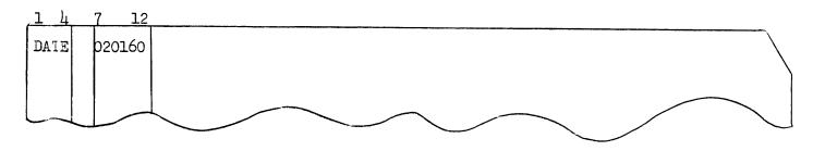
Assemble Compool Control Card - One control card can be used to assemble (Symbolic Prestored) or reassemble (using binary tape from previous incorrect assembly) up to three Compools. The control card carries the Compool idents and Column 25 determines the mode (assembly or reassembly.)
