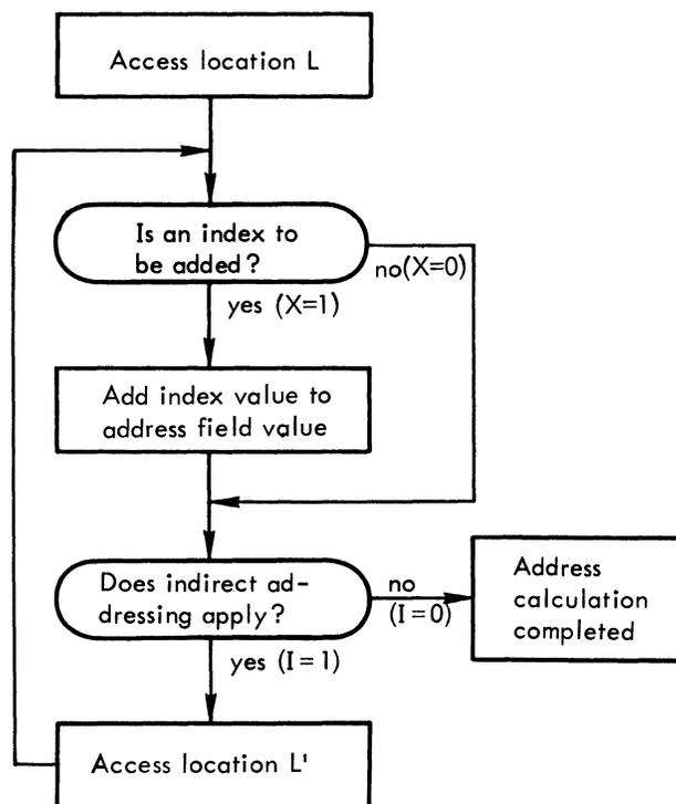
Figure 4. Effective Virtual Address Calculation
