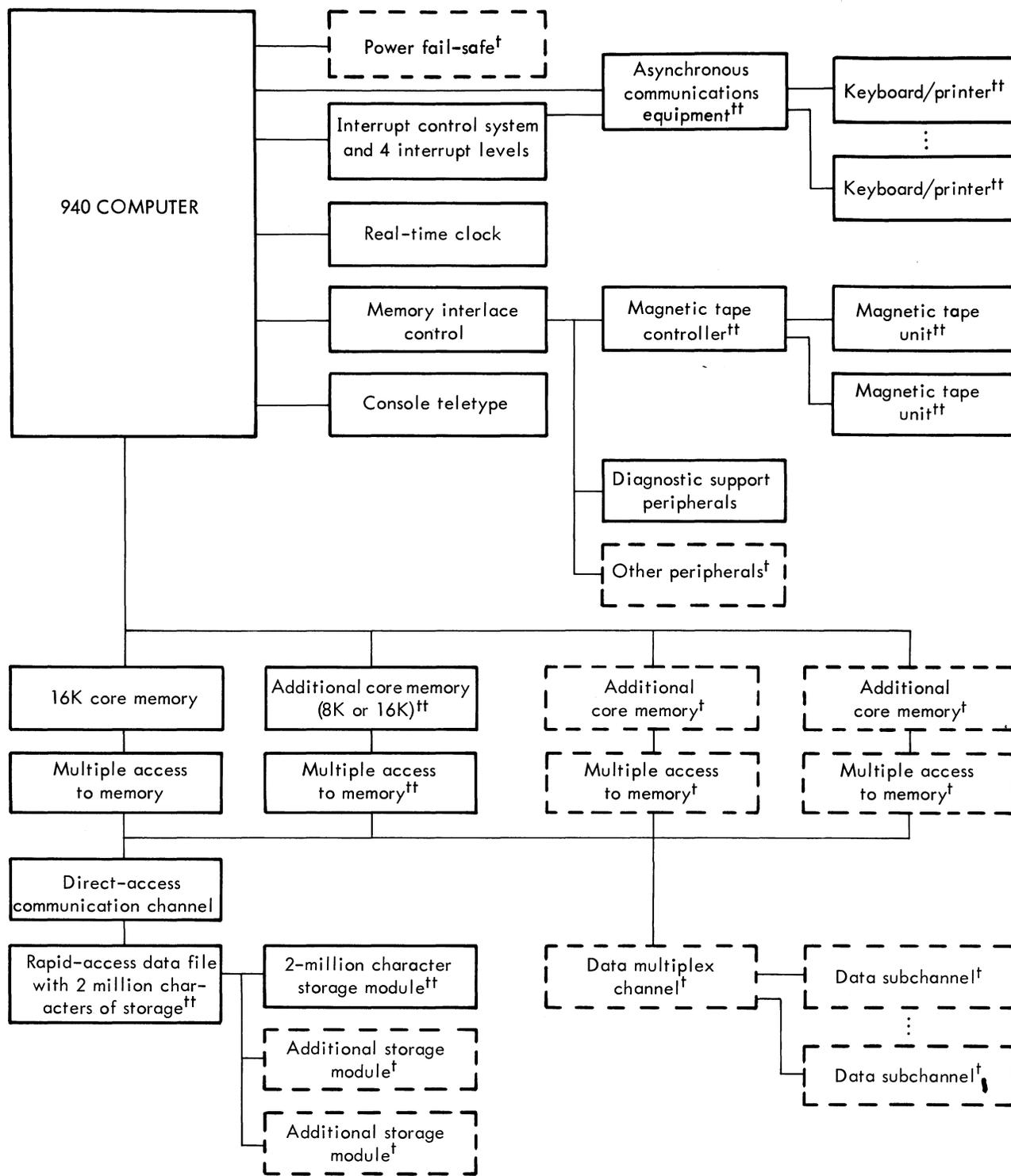
Figure 1. SDS 940 Time-Sharing Computer System
