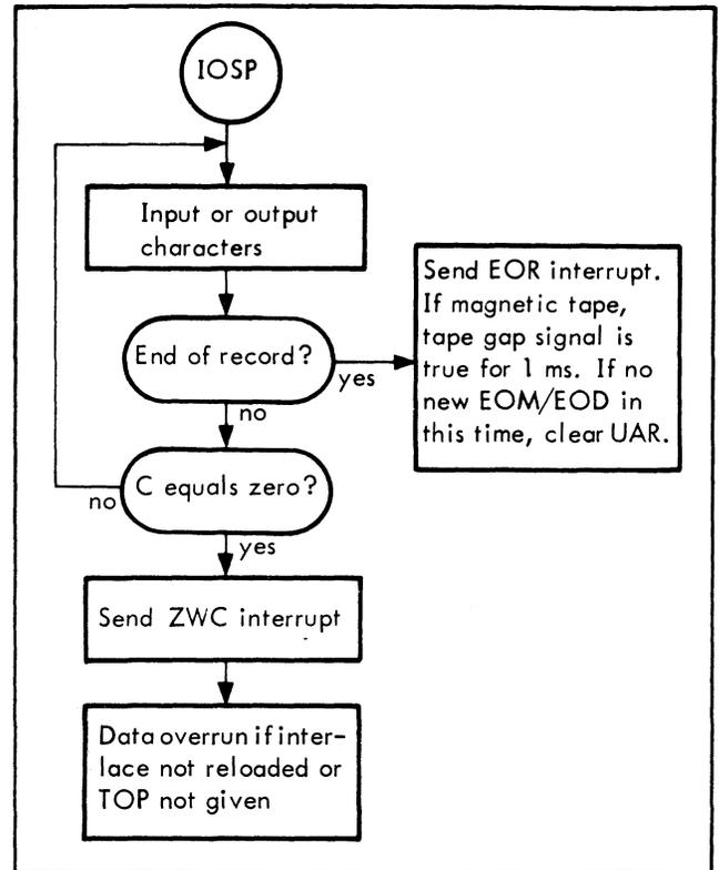
**Input C Words.** If the channel receives C words before the peripheral device encounters the end-of-record, the channel generates a zero word count interrupt (if armed). The program should reload the interlace portion of the channel to continue reading the record. Failure to reload the interlace before the peripheral device sends enough characters to overflow the word assembly register causes a character rate error; this sets the channel error indicator.
