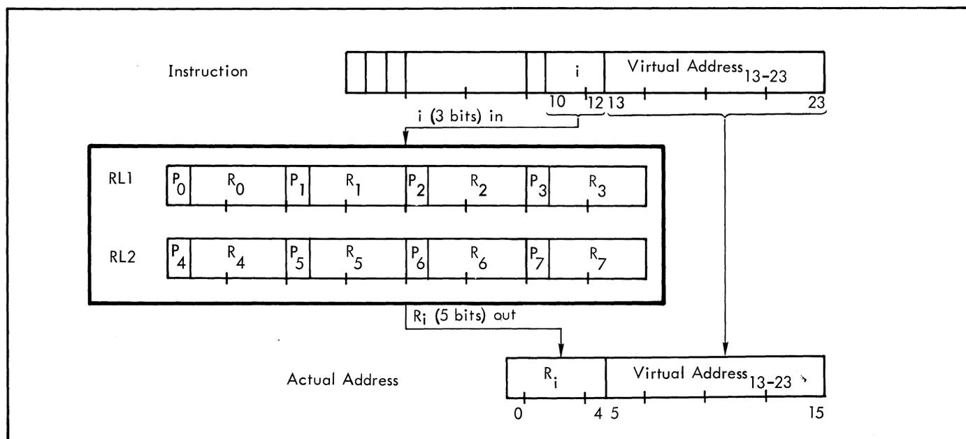
Figure 3. SDS 940 Mapping Process
