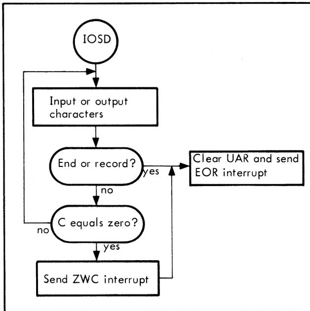
The IOSD function is designed for use on devices that are normally operated on the basis of the word count only. Typewriters and paper-tape devices are of this type, as are the printer and card punch when the user does not wish to stay connected until the operation is complete.
