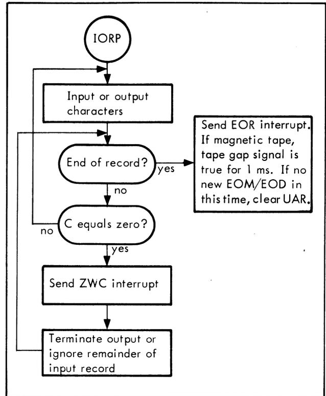
A program should not use the IORP function with devices that do not generate end-of-record responses upon output termination; such devices are paper tape and typewriter. These devices do terminate output but give the program no indication when they receive the last character.
