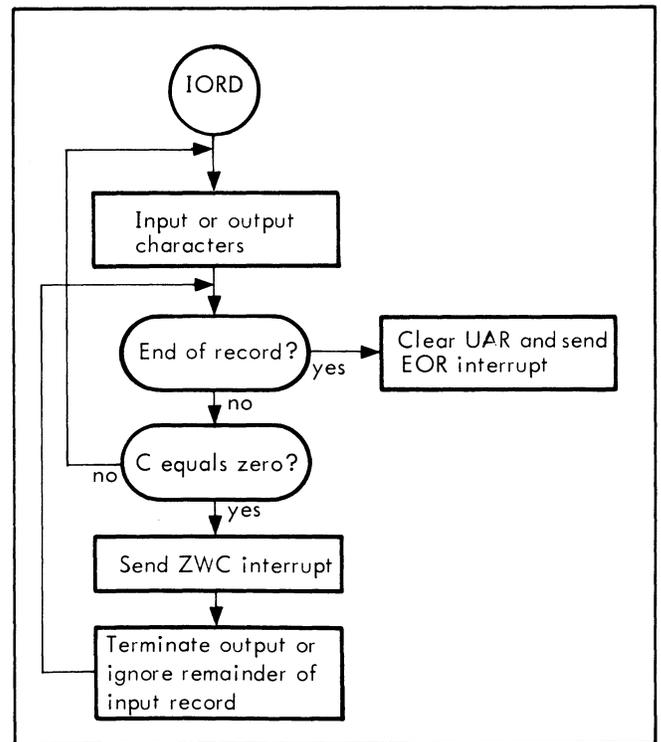
A program should not use the IORD function with devices that do not have end-of-record conditions on output (e.g., devices such as the paper tape punch and typewriter). These devices do terminate output but give the program no indication when they receive the last characters.
