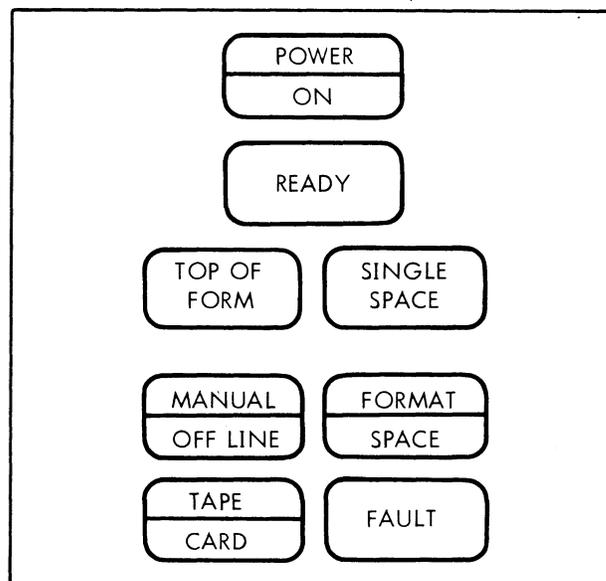
Figure 10. Printer Control Indicator Lights and Switches
