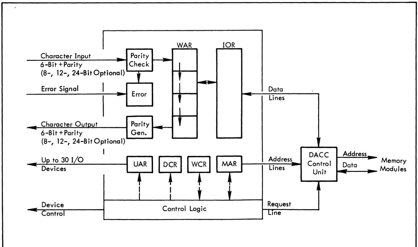
Figure 7. Typical SDS 940 Direct-Access Communication Channel, Block Diagram
