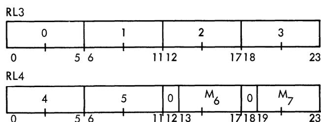
Actually, only the portions of the two registers labeled  $M_6$  and  $M_7$  are implemented with flip-flops. The other six registers may be thought of as though they permanently contained the following values:
