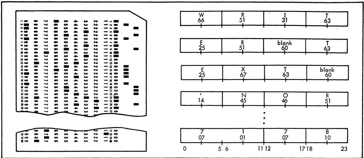
Figure 9. Card Read Into Memory in Hollerith
