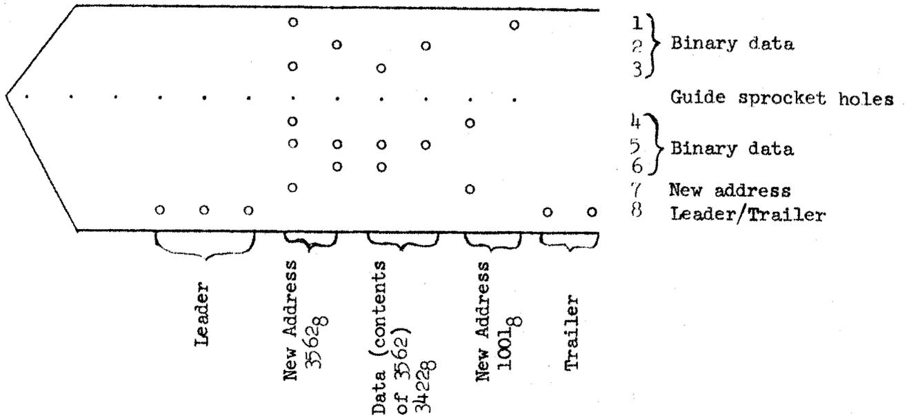
The distinction between RIM and BIN is that any number of Data words may follow an Address word, each filling successive locations with BIN tape while with RIM tape each Data word must be preceded by an Address word. Also, BIN tape often has a check-sum word at the end of the tape. The Bootstrap-loader switch will read either format, but will ignore any check-sums.
