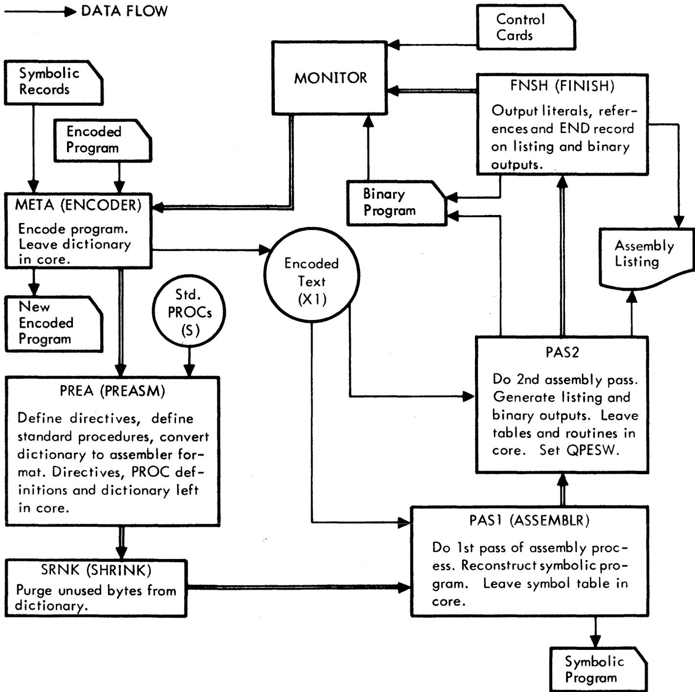
Figure 1-1. MONITOR-META-SYMBOL Data Flow
