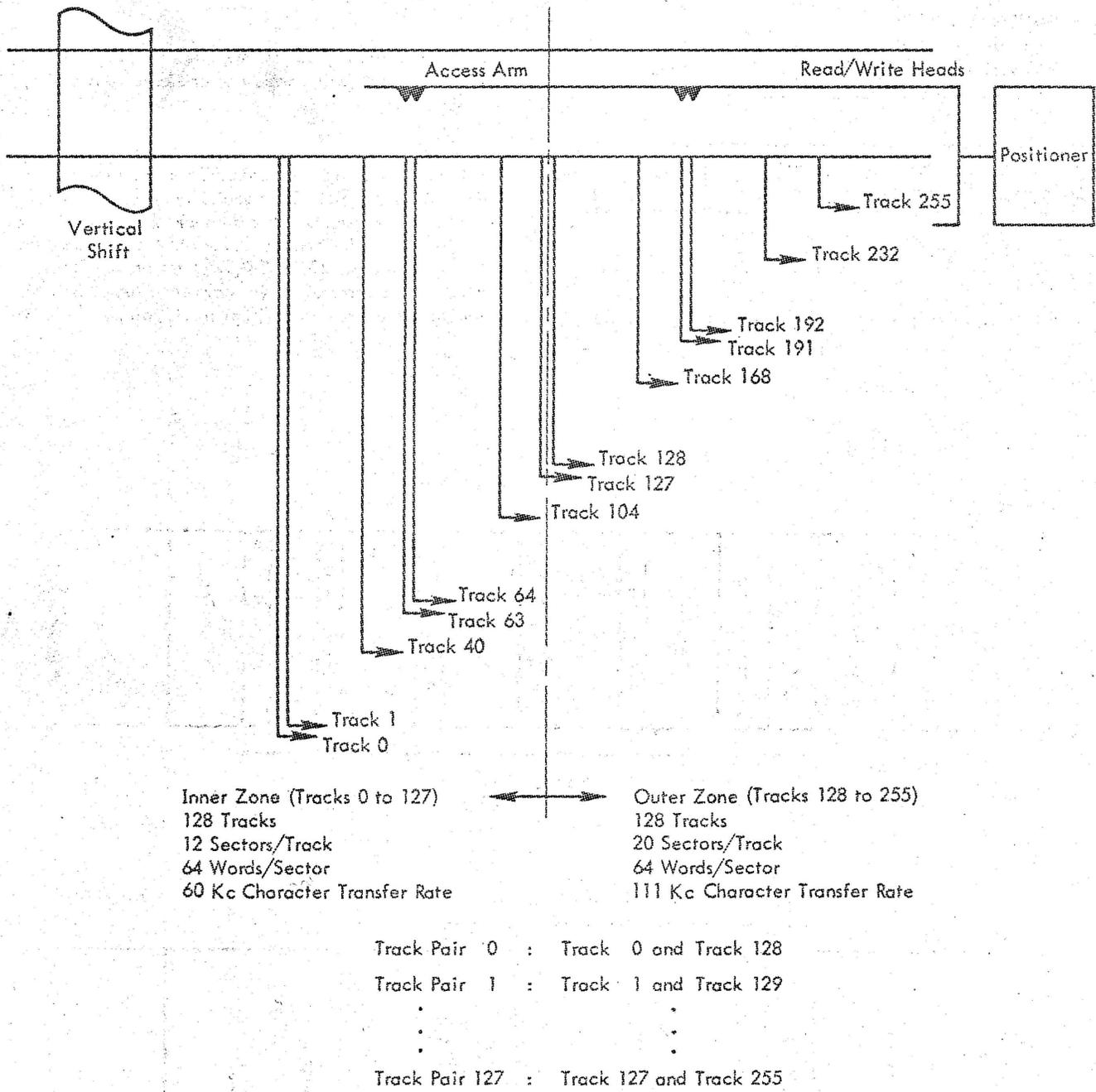
Figure 6. Organization of Model 9165 Inner/Outer Recording Zones and Track Pairs
