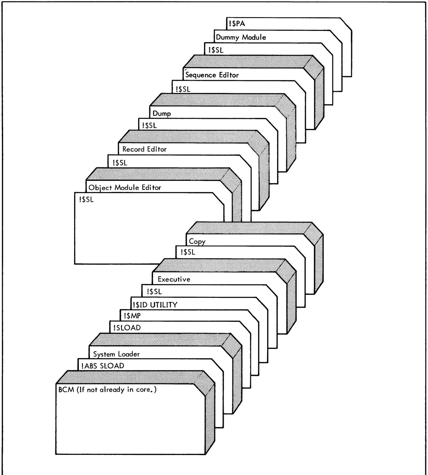
Figure 13. Deck Setup to Punch Absolute Utility Package
