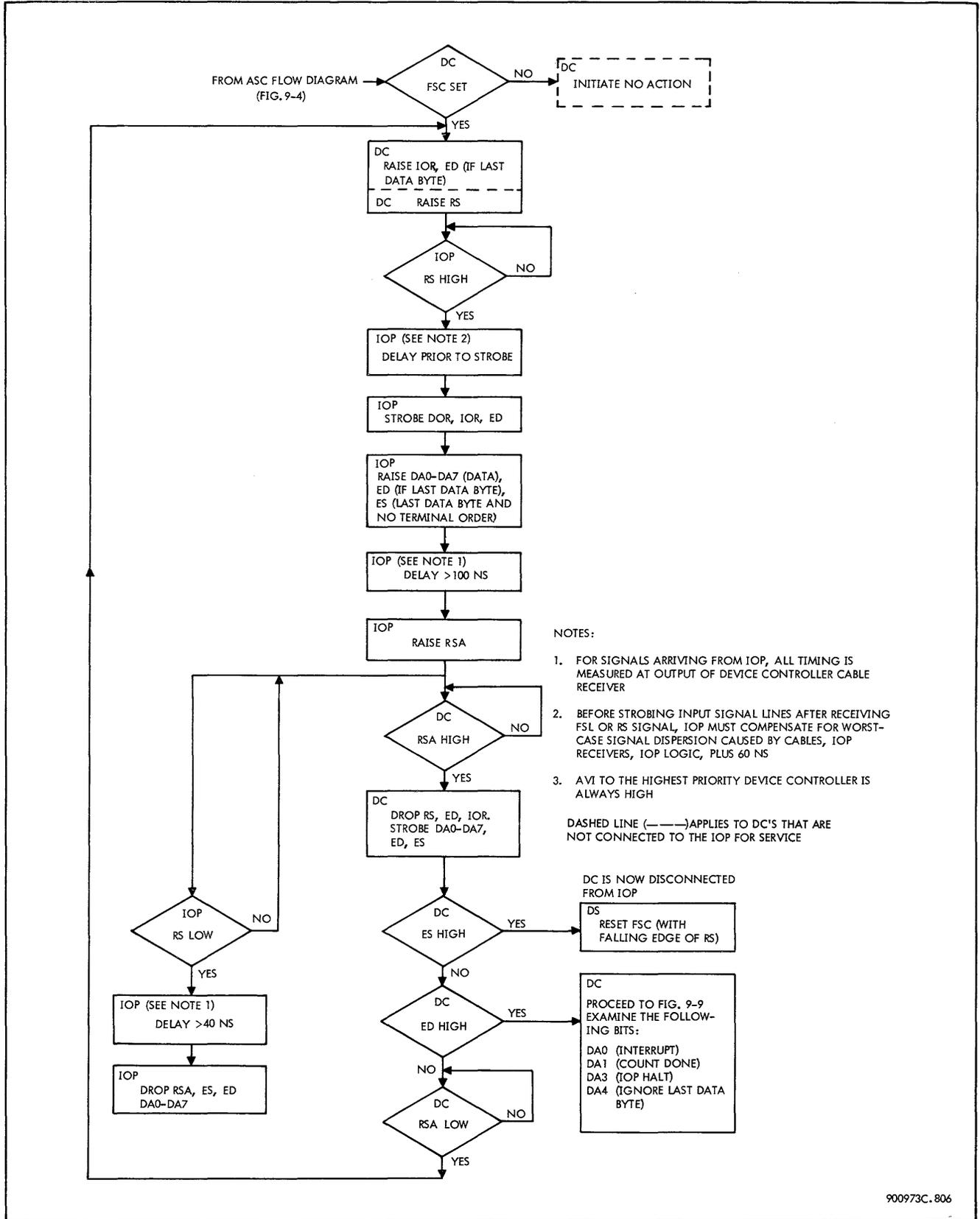
Figure 9-6. Service - Data Output, Flow Diagram
