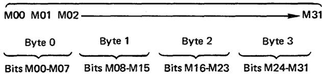
The most significant bit and byte are M00 and byte 0, respectively. The partial write mode allows writing of one or more bytes within a word without altering the remaining byte or bytes within the word. The Sigma 5 and 7 memories consist of one to eight memory banks. Each bank is functionally independent and provides storage for 4K, 8K, 12K, or 16K words.
