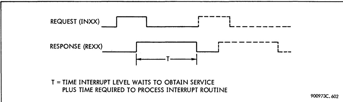
Figure 7-2. External Interrupt Request and Response, Timing Diagram
