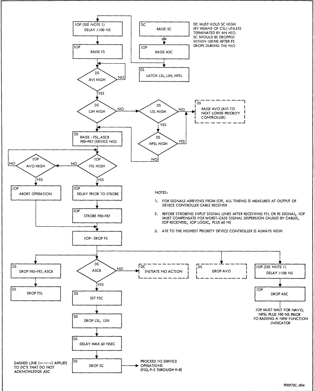
Figure 9-4. ASC (Prior to Service Connection), Flow Diagram
