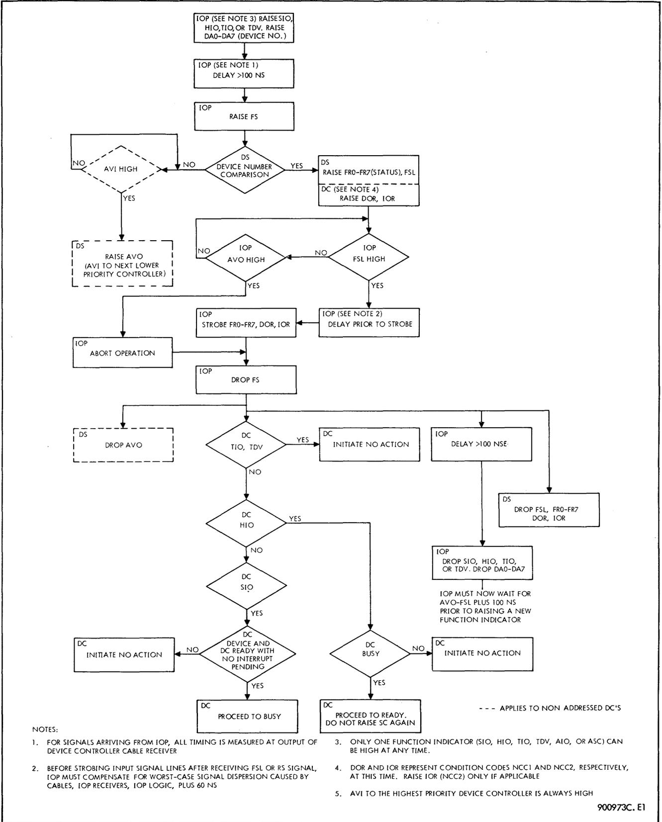
Figure 9-2. SIO, HIO, TIO, and TDV, Flow Diagram
