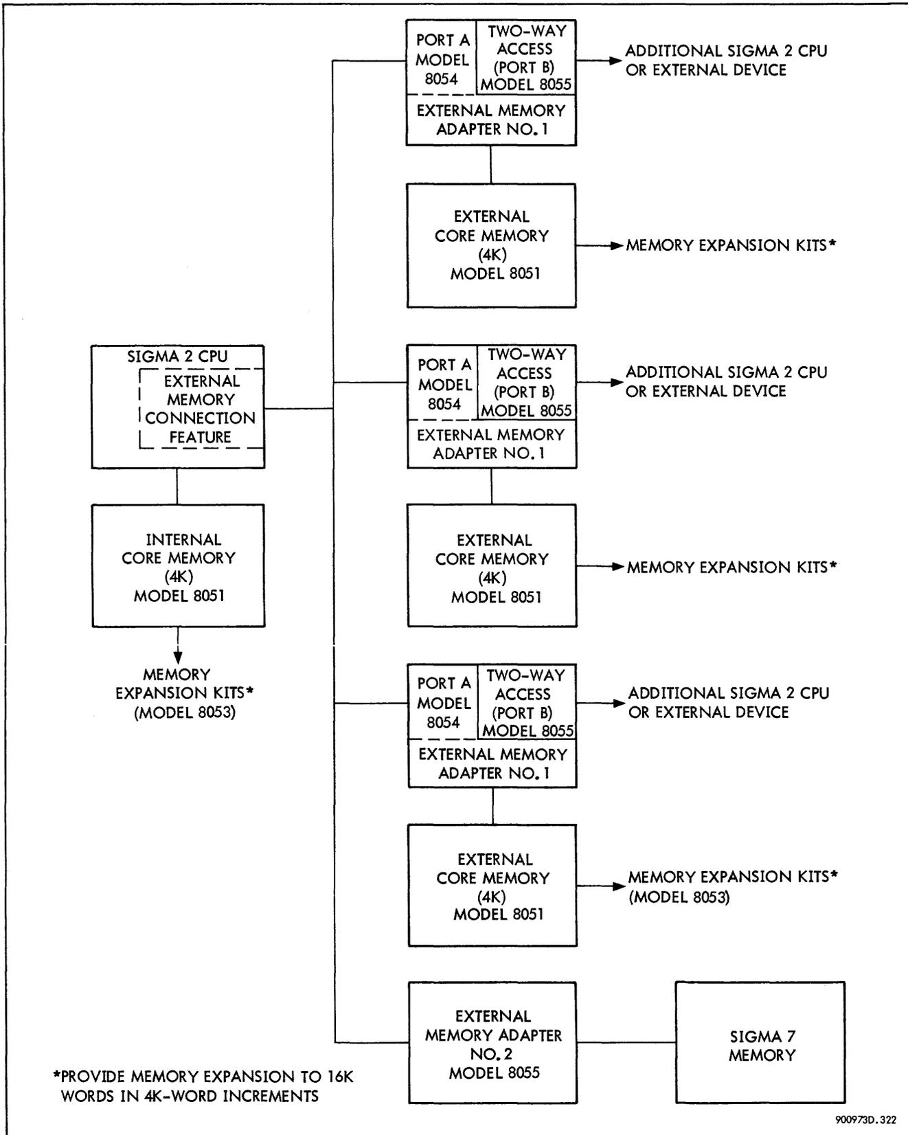
Figure 4-1. Sigma 2 Memory System, Block Diagram
