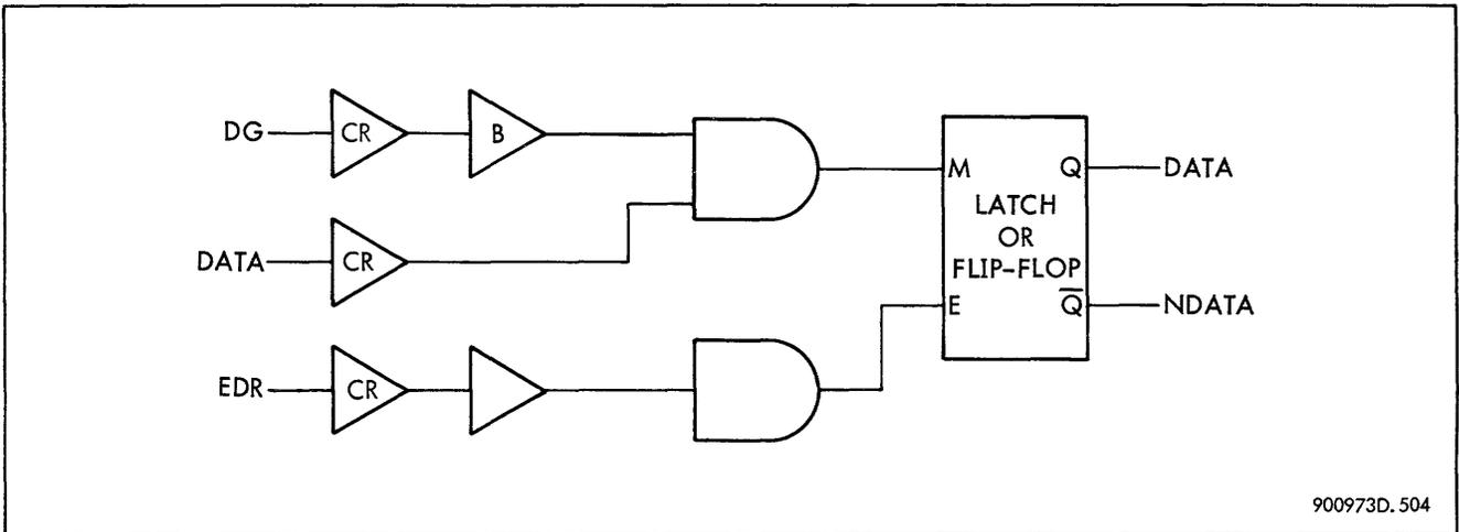
Figure 6-4. Read and Hold Memory Data, Logic Diagram
