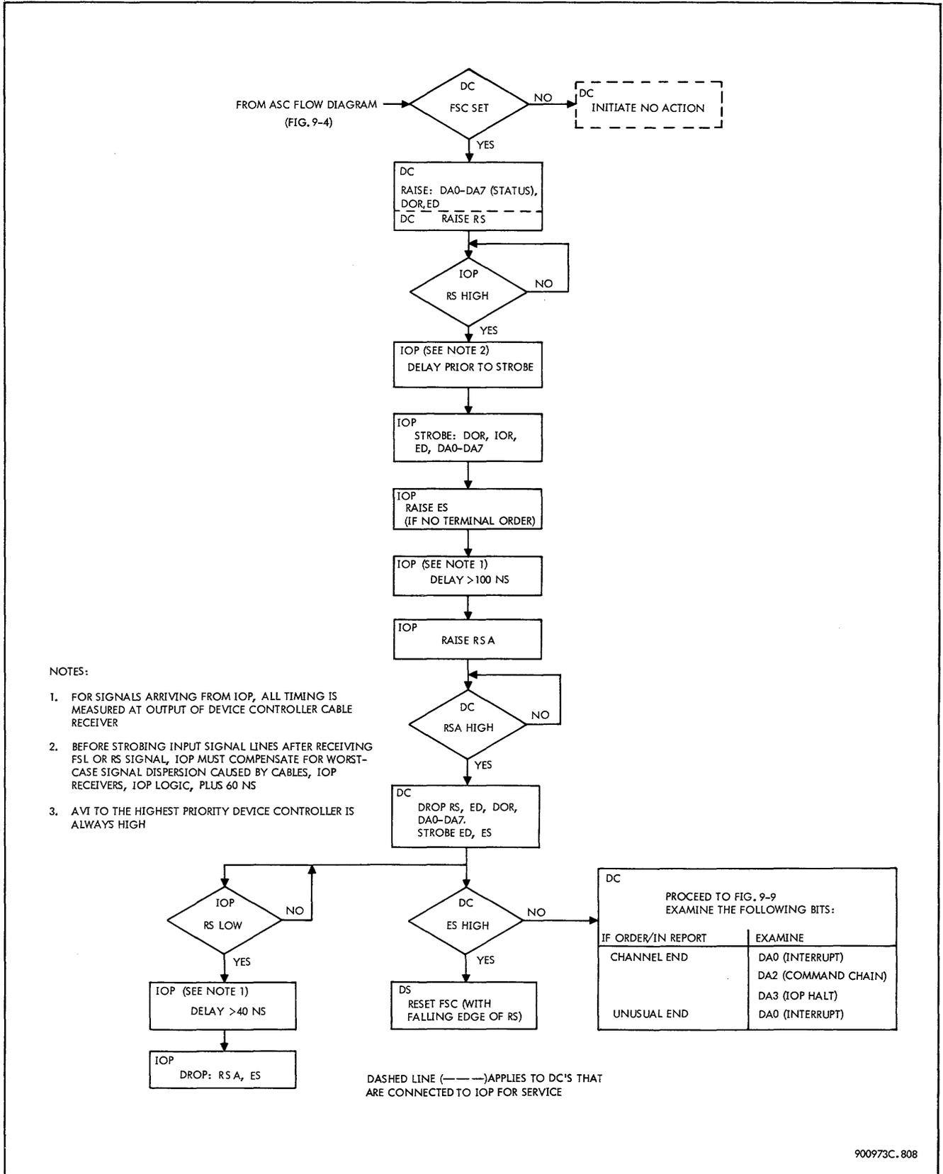
Figure 9-8. Service - Order Input, Flow Diagram
