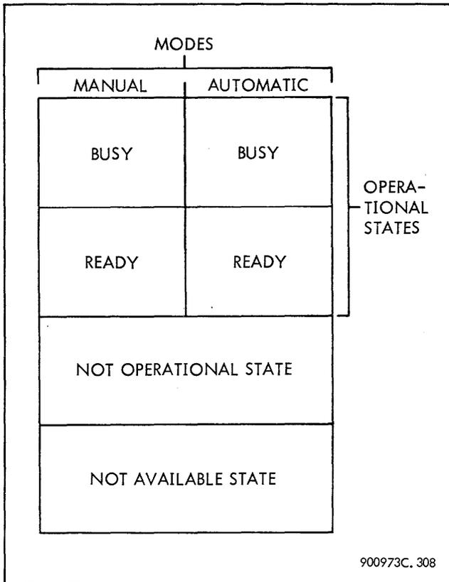
Figure 3-8. Device Mode and State Diagram
