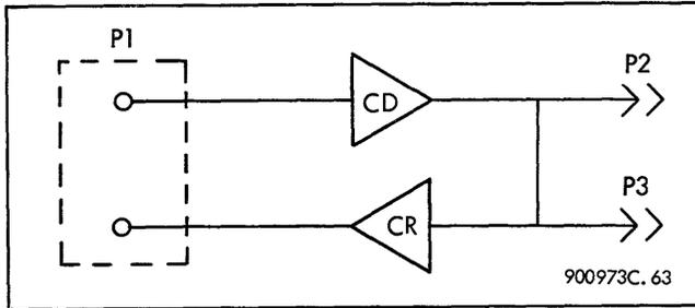
Figure 7-3. AT11 Cable Driver-Cable Receiver Circuit, Schematic Diagram
