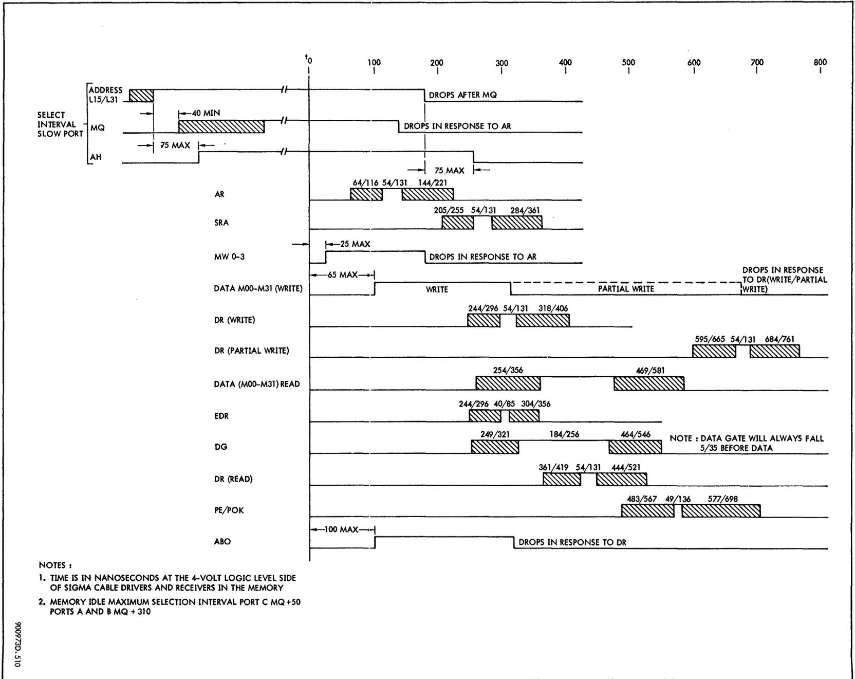
Figure 6-3. Ports 1, 2, 3, and 4, Timing Diagram
