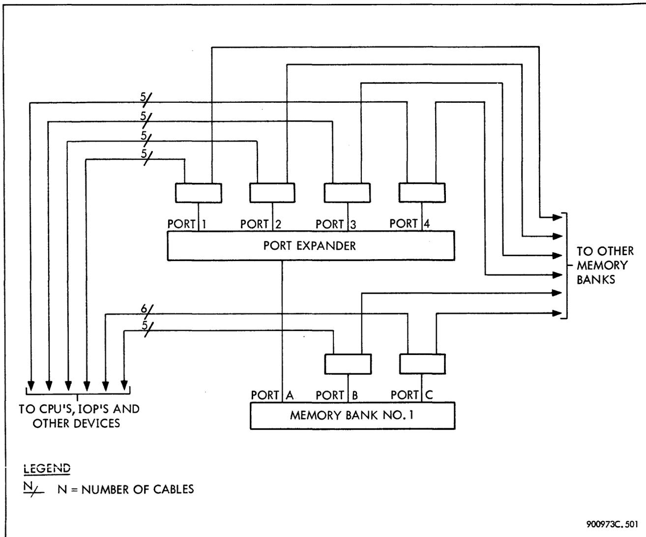
Figure 6-1. Memory Port Expander, Installation Block Diagram
