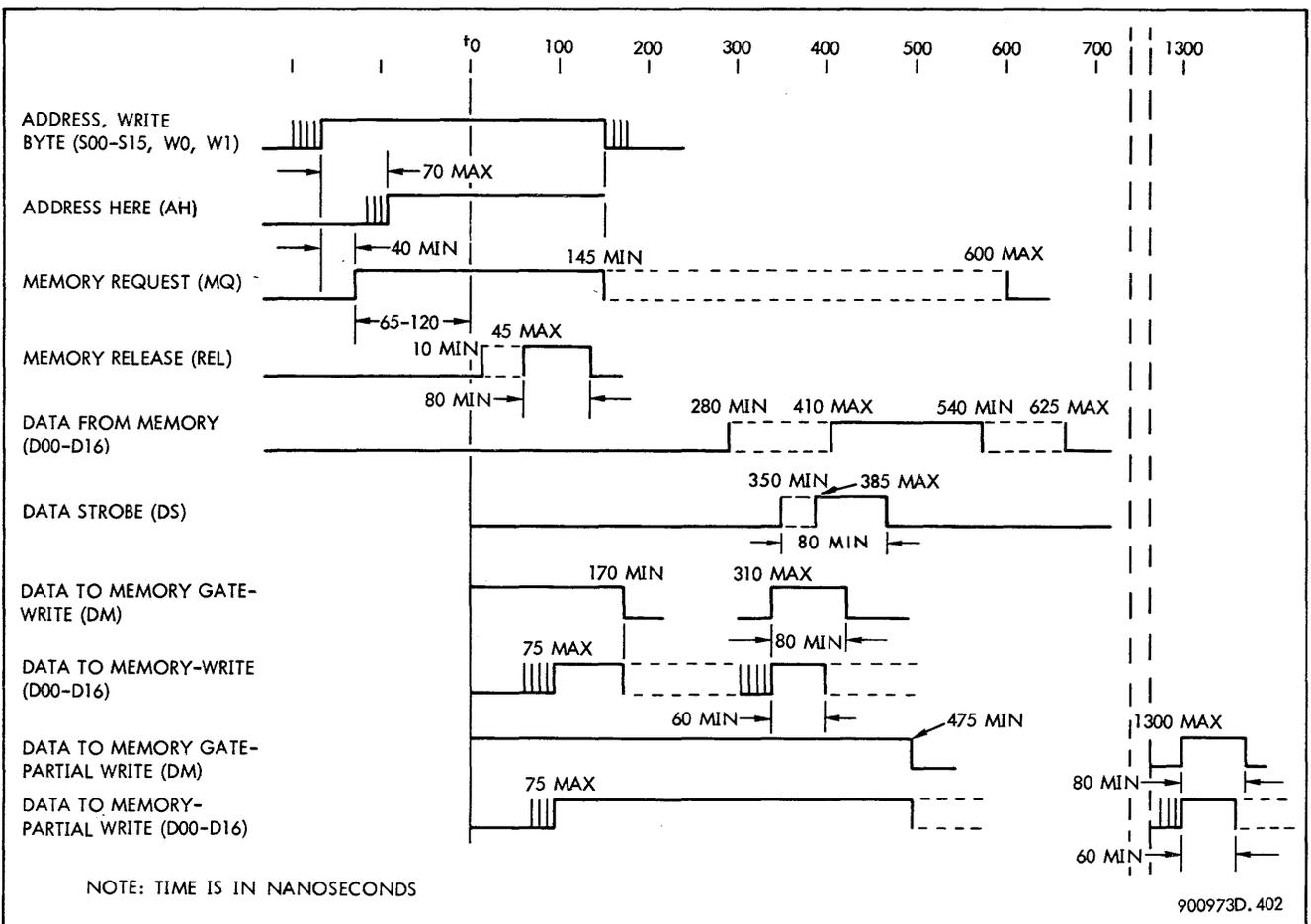
Figure 4-2. Sigma 2 External Memory, Timing Diagram
