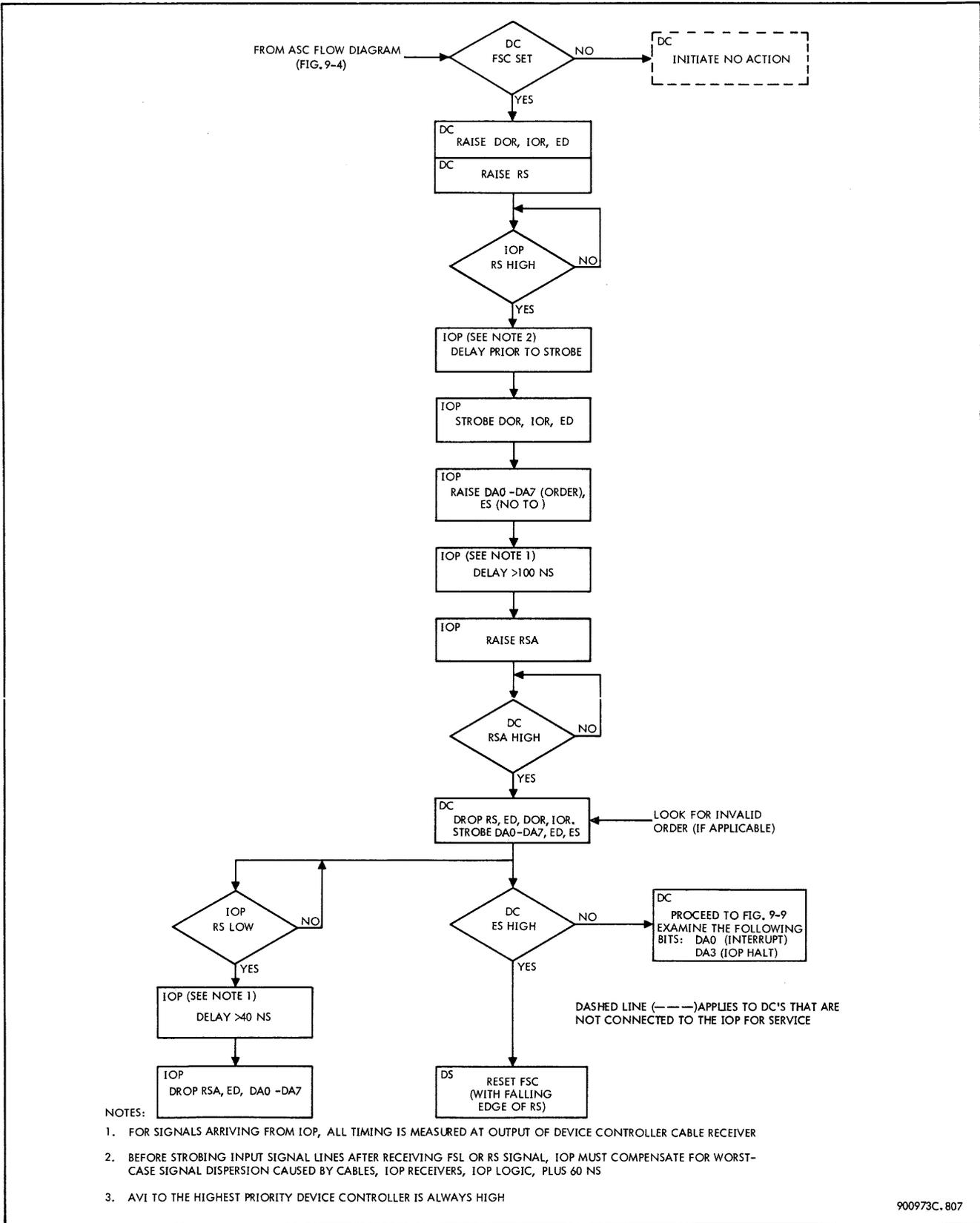
Figure 9-7. Service - Order Output, Flow Diagram
