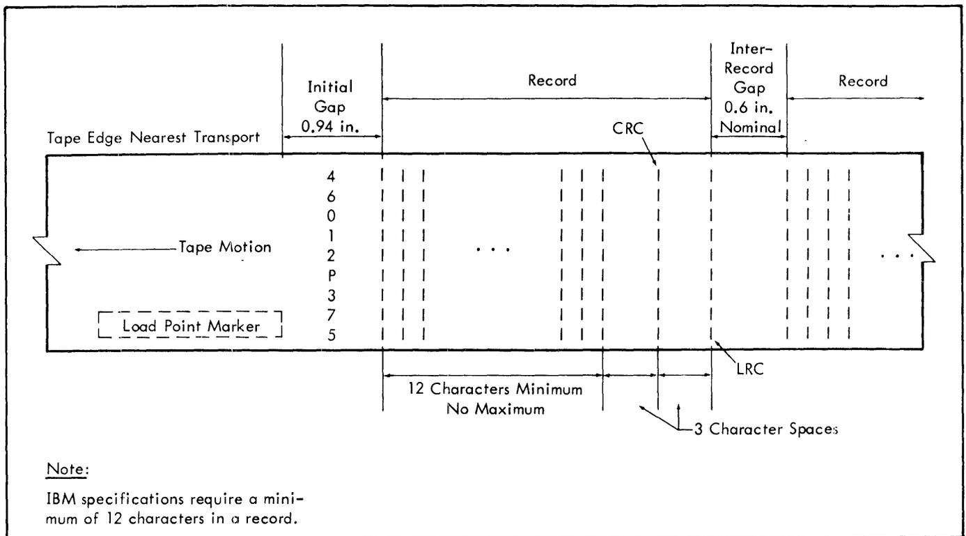
Figure 2. Physical Spacing on Tape
