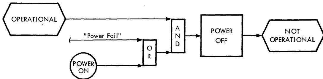
Figure 10. Device State Sequence From "Operational"
