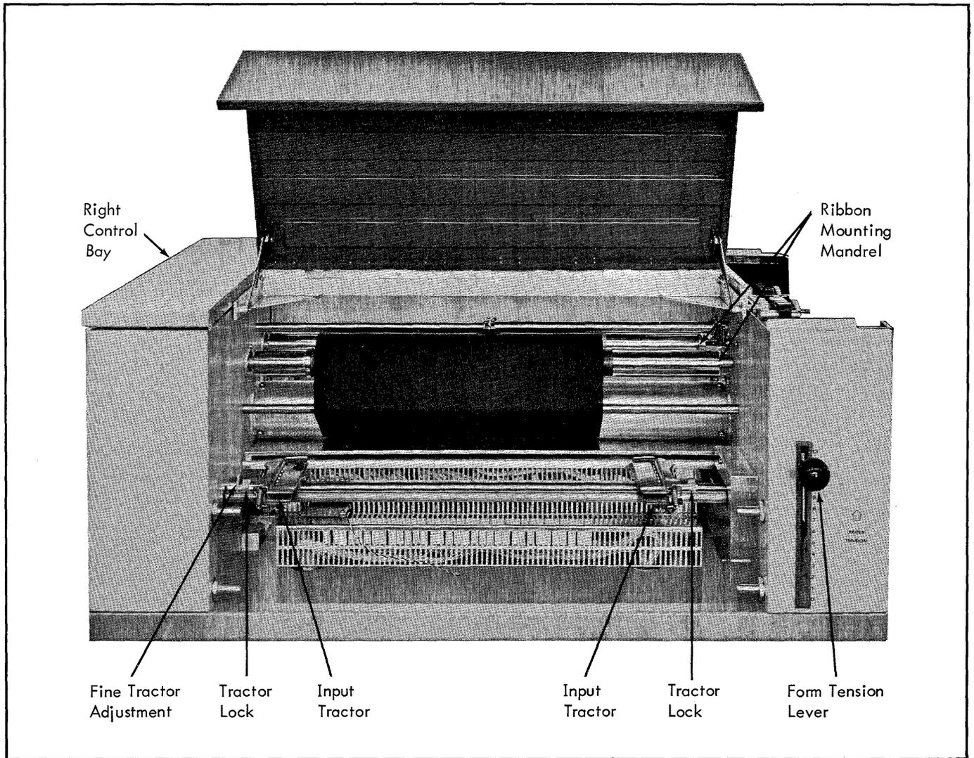
Figure 4. Printer Mechanism, Rear View
