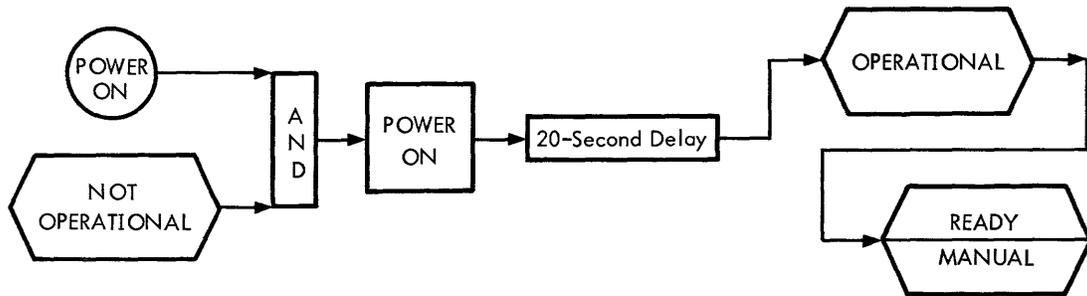
Figure 9. Device State Sequence From "Not Operational"
