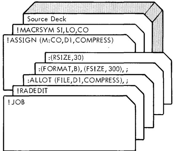
In this example, the CO device is assigned to a RAD file called COMPRESS in a background data area of the RAD. The compressed output is written on the COMPRESS file.
