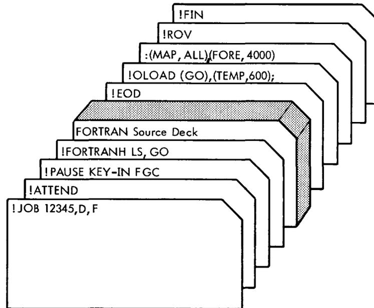
In this example, the !ATTEND command will inhibit the Monitor ABORT routine so that corrective action can be taken at the console in case of error. The FORE option on the !OLOAD command gives the FWA of the program in the Foreground area of memory.
