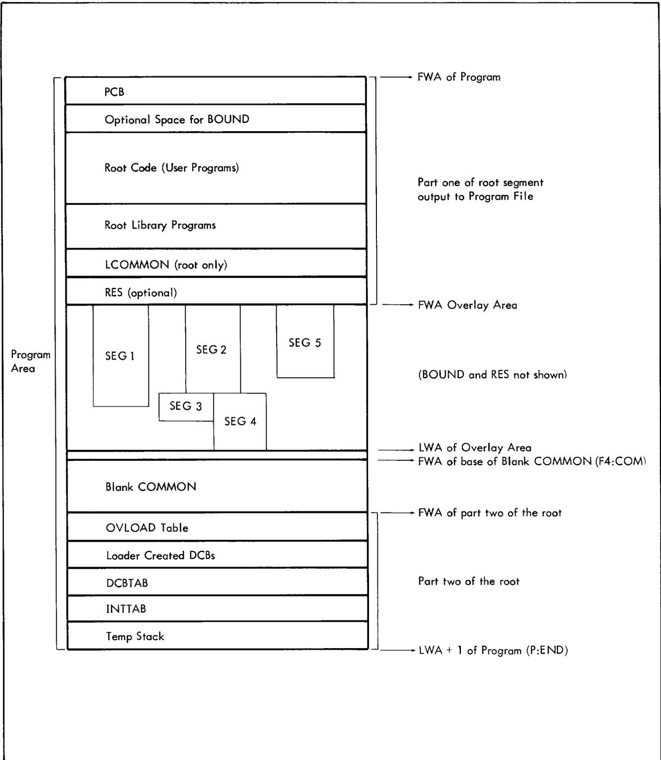
Figure 13. Standard Core Layout of a Program
