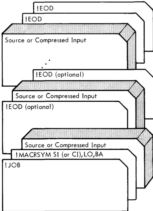
In this example, successive assemblies are performed with a single MACRSYM command until a double EOD is read. The device assignments and options on the MACRSYM command apply to all assemblies within the batch. A program is considered terminated when an END Macro-Symbol directive is processed.
