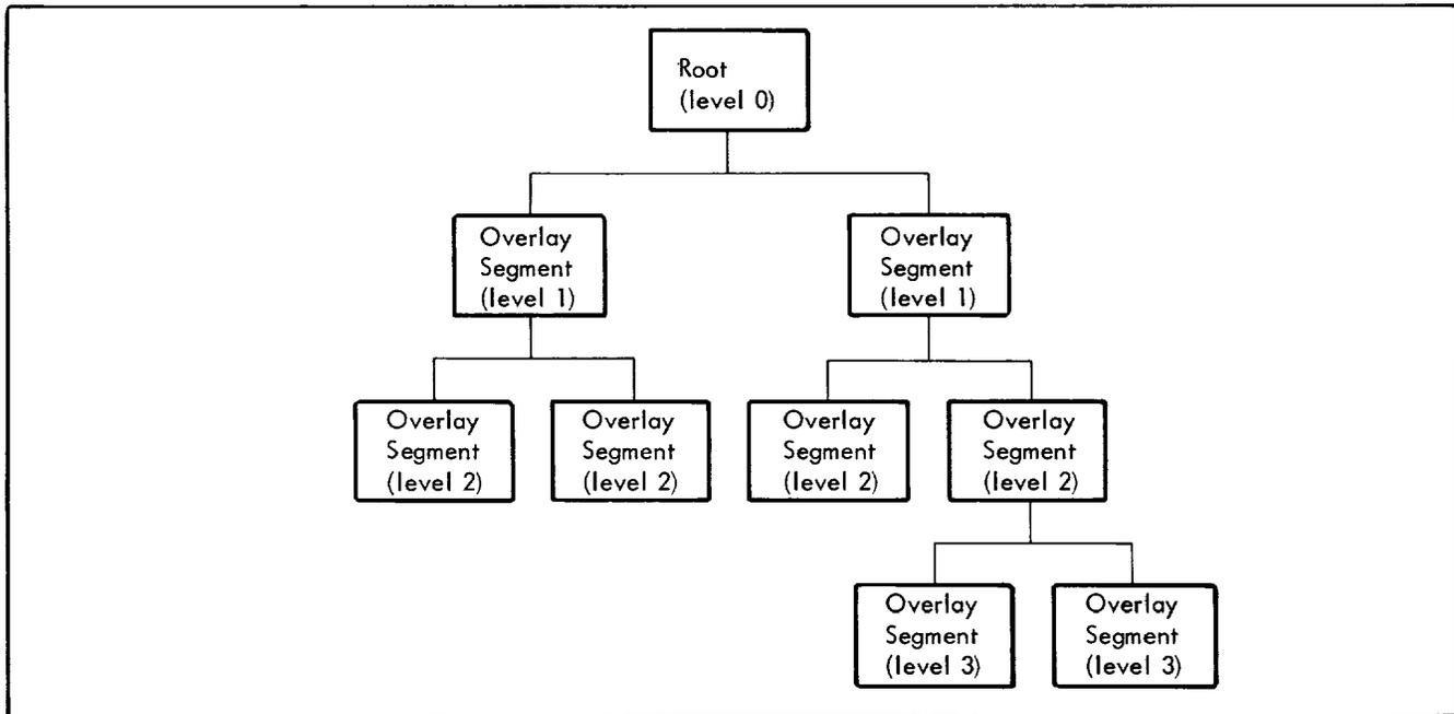
Figure 1. Overlay Structure
