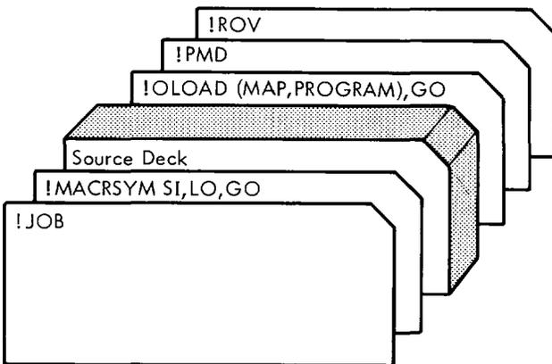
In this example, the binary object program produced from the assembly is placed in a temporary (GO) file from which it is later loaded and executed. The resultant file is always temporary and cannot be retained from one job to another. The Overlay Loader loads the program root into the OV file for execution. A postmortem dump is specified.
