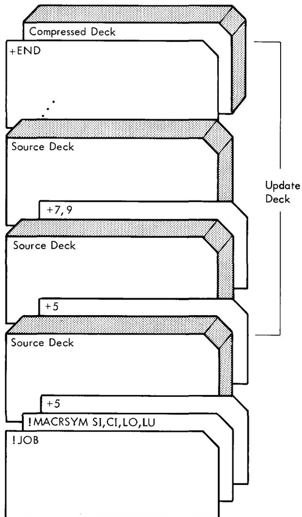
In this example, the compressed input (deck) is received from the CI device, listing output is produced on the LO device, and listing of the update deck is also produced on the LO device. The update deck is enclosed in the bracket.
