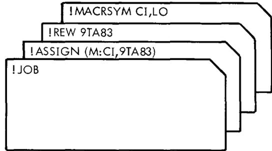
In this example, the CI device is assigned to the designated magnetic tape to read the compressed input to be assembled. This is the next logical job step to follow the previous example.
