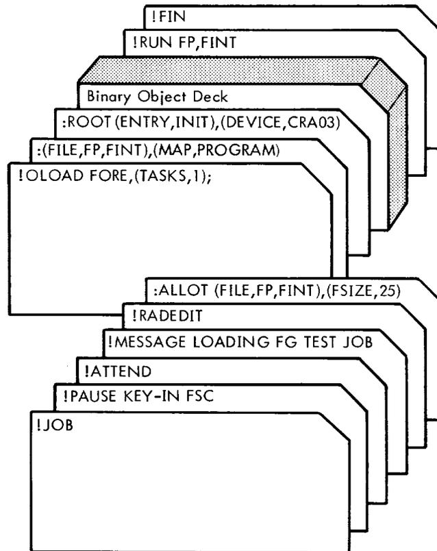
In this example, the RAD Editor allots a file, (FINT) in the Foreground Programs (FP) area of the RAD. The Overlay Loader loads the binary object deck in the file FINT in core image format. The !RUN control command causes execution of the foreground program. A PROGRAM map is specified.
