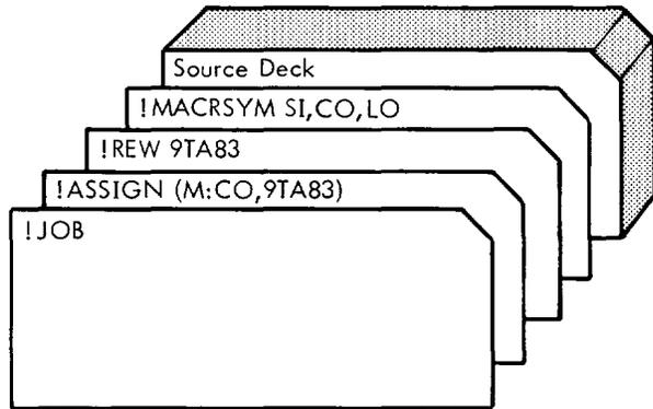
In this example, the CO device is assigned to the designated 9-track magnetic tape unit to receive the compressed output.
