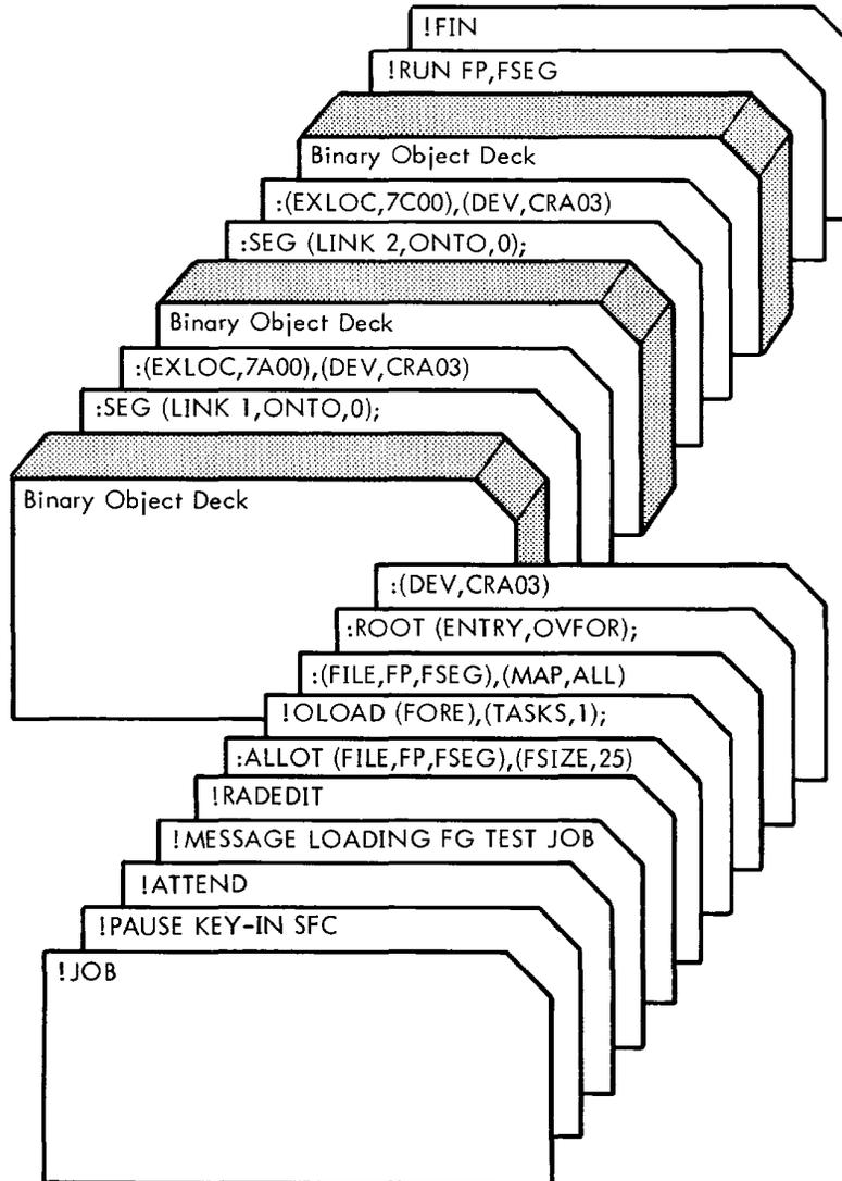
In this example, the RAD Editor allots space for a file called FSEG in the Foreground Programs (FP) area of the RAD. The Overlay Loader loads a root and two segments into FSEG in core image format. The overlaid program is executed via the !RUN control command. An ALL map is requested.
