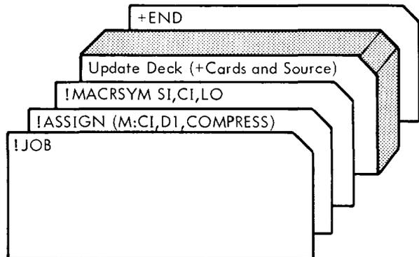
In this example, the CI (compressed input) device is assigned to the COMPRESS file in a background area of the RAD. The source update deck will be read from the SI device. In effect, this will update the assembly given in the previous example.
