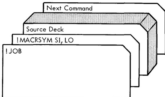
In this example, the symbolic input is received from the SI device and the listing output is produced on the LO device.
