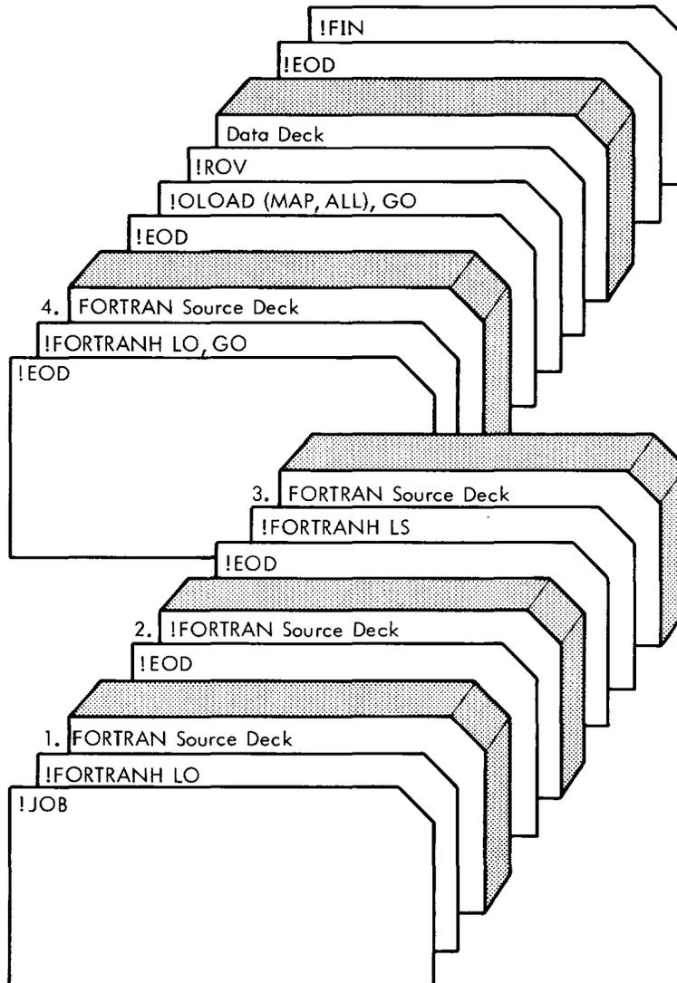
In this example, the first two source decks are compiled with mixed (source and object language) listed output. The next source program (3) is compiled with a source listing (only) being output. The final source deck (4) will compile with the object module being output on both the BO and GO files. The Loader inputs the object module from the GO file to form the Root and outputs the executable program to the OV file. The program (called OV) is executed via the !ROV command.
