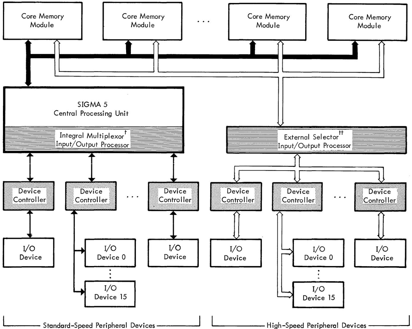
Figure 1. A typical SIGMA 5 System
