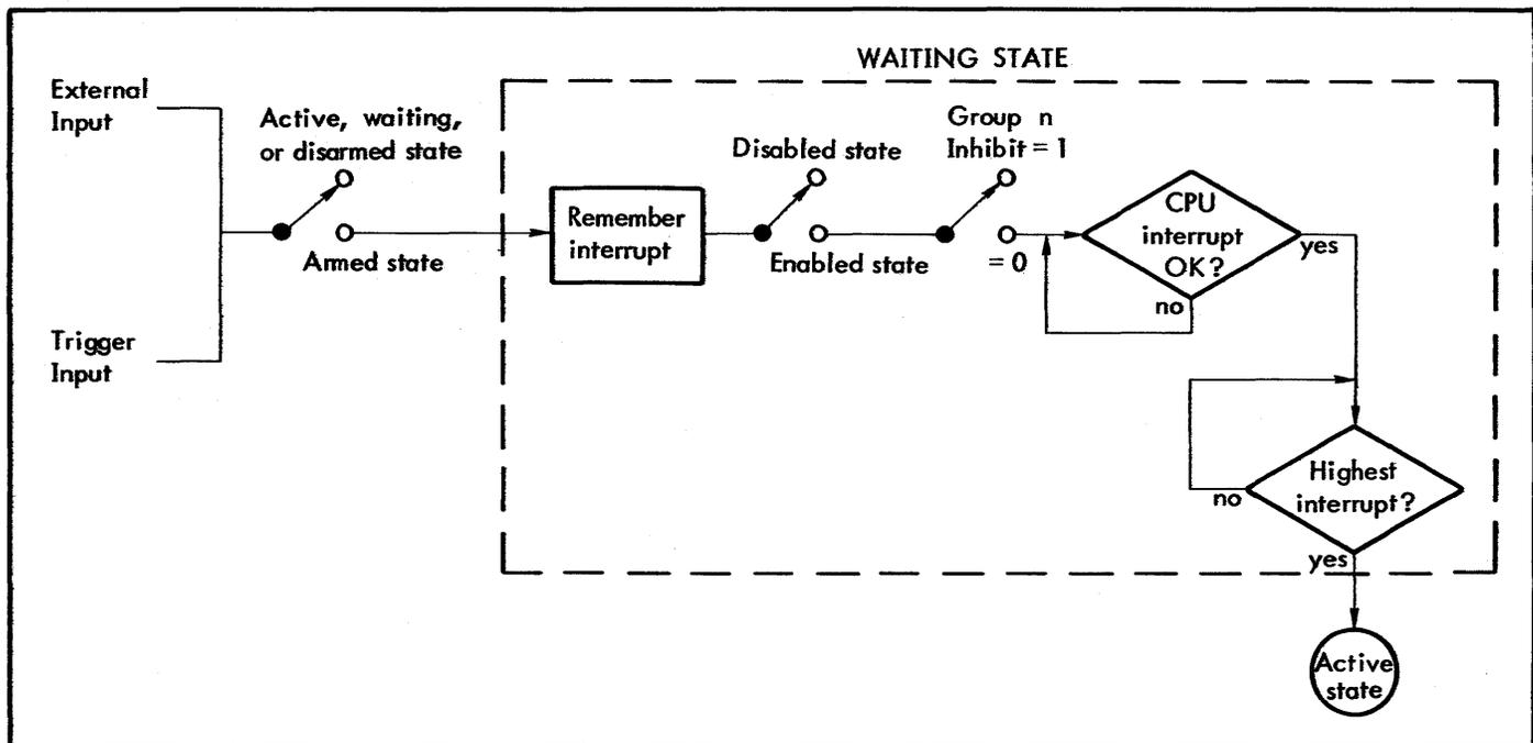
Figure 10. Operational States of an Interrupt Level
