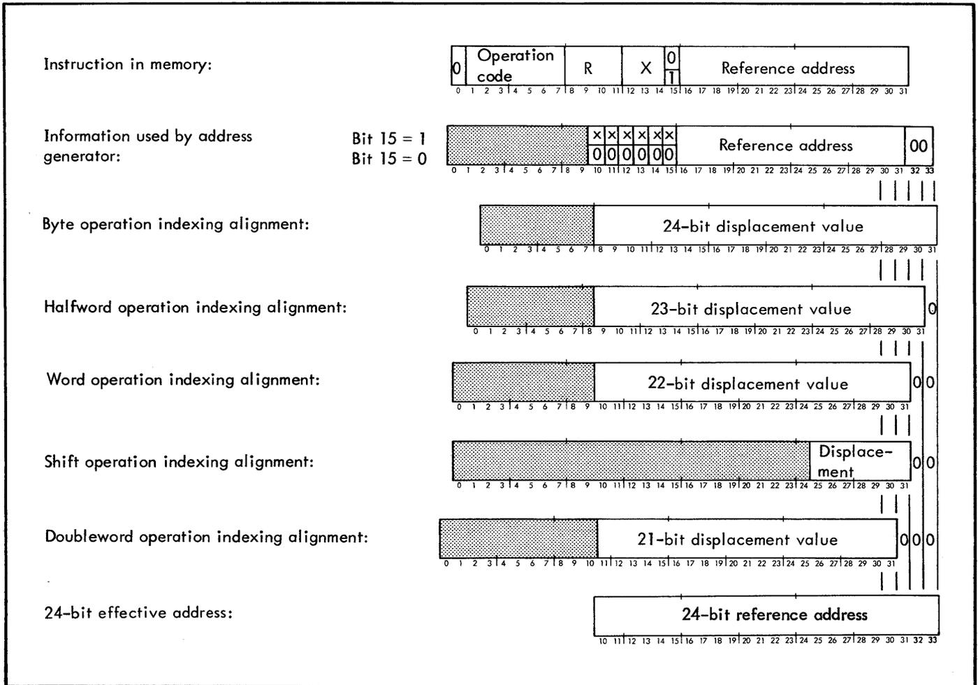
Figure 6. Index Displacement Alignment (Real Extended Addressing)
