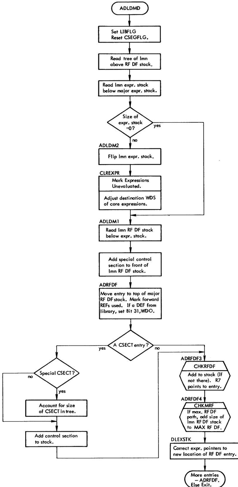
Figure 20b. PASS1 Load Module Processor (ADLDM) Flow Chart
