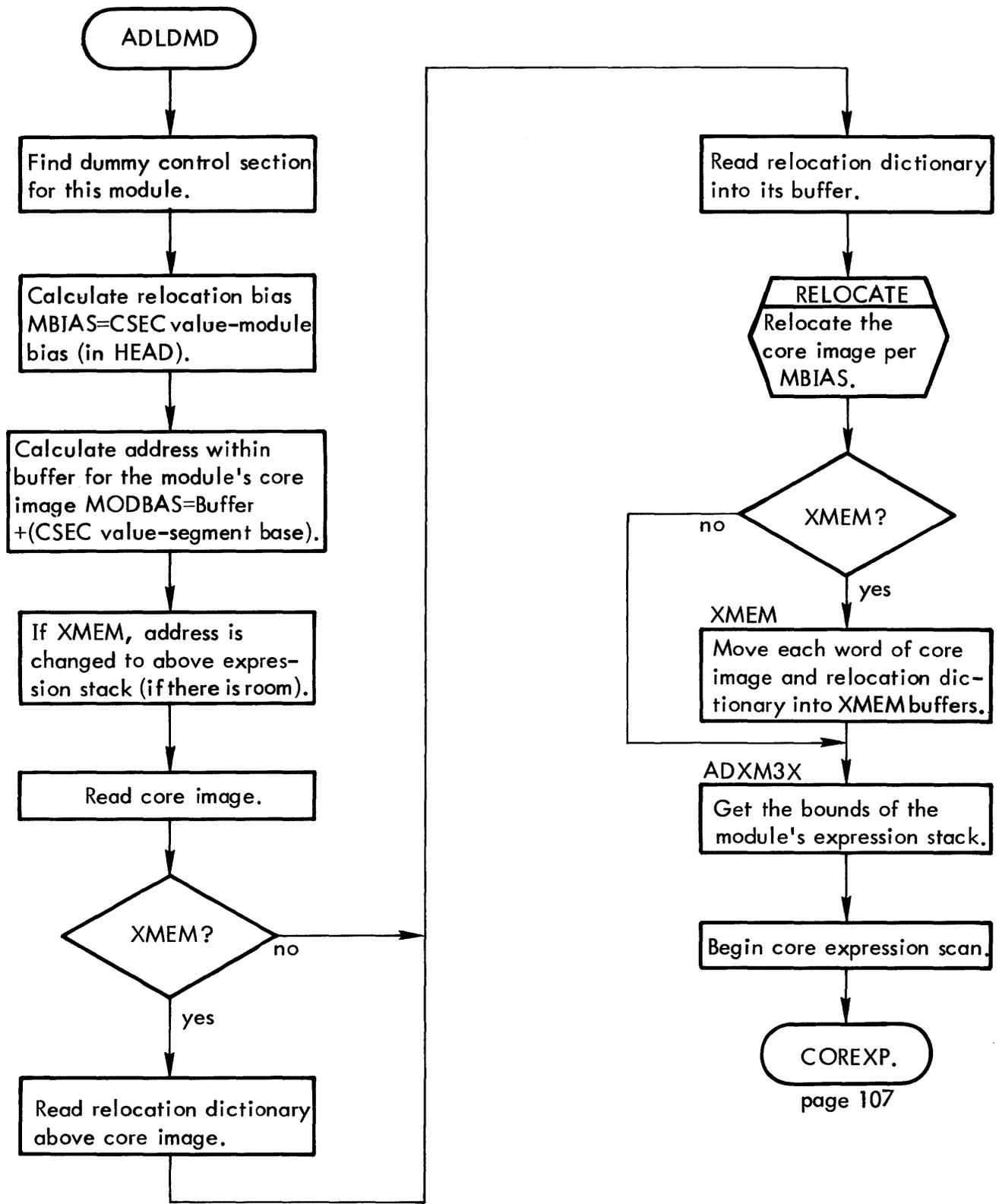
Figure 28. PASS2 Load Module Processor Flow Chart
