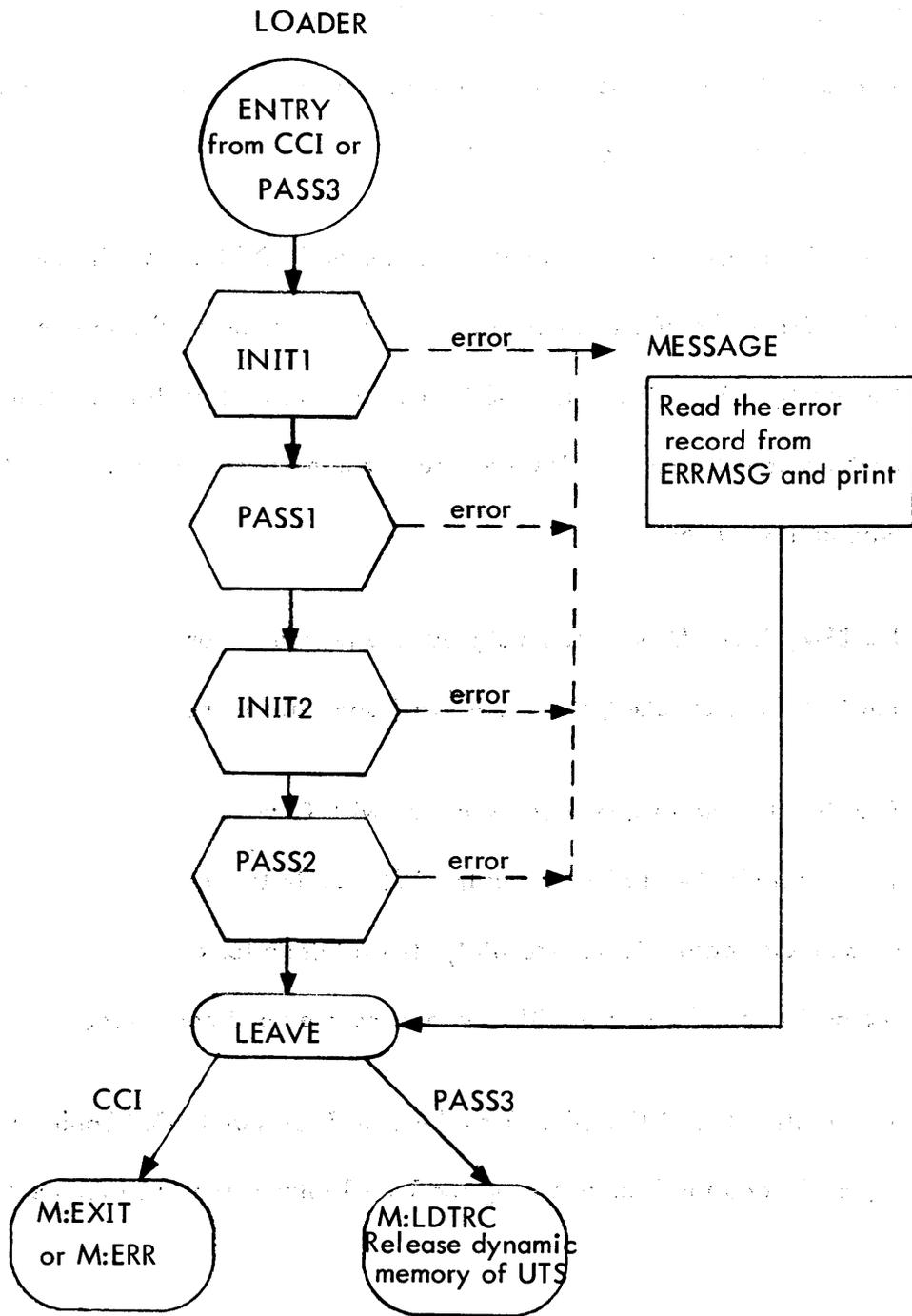
Figure 17. The Loader Driver (in LDR) Flow Chart
