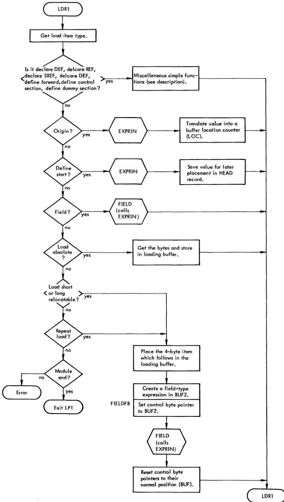
Figure 26. PASS2 Object Module Processor Flow Chart
