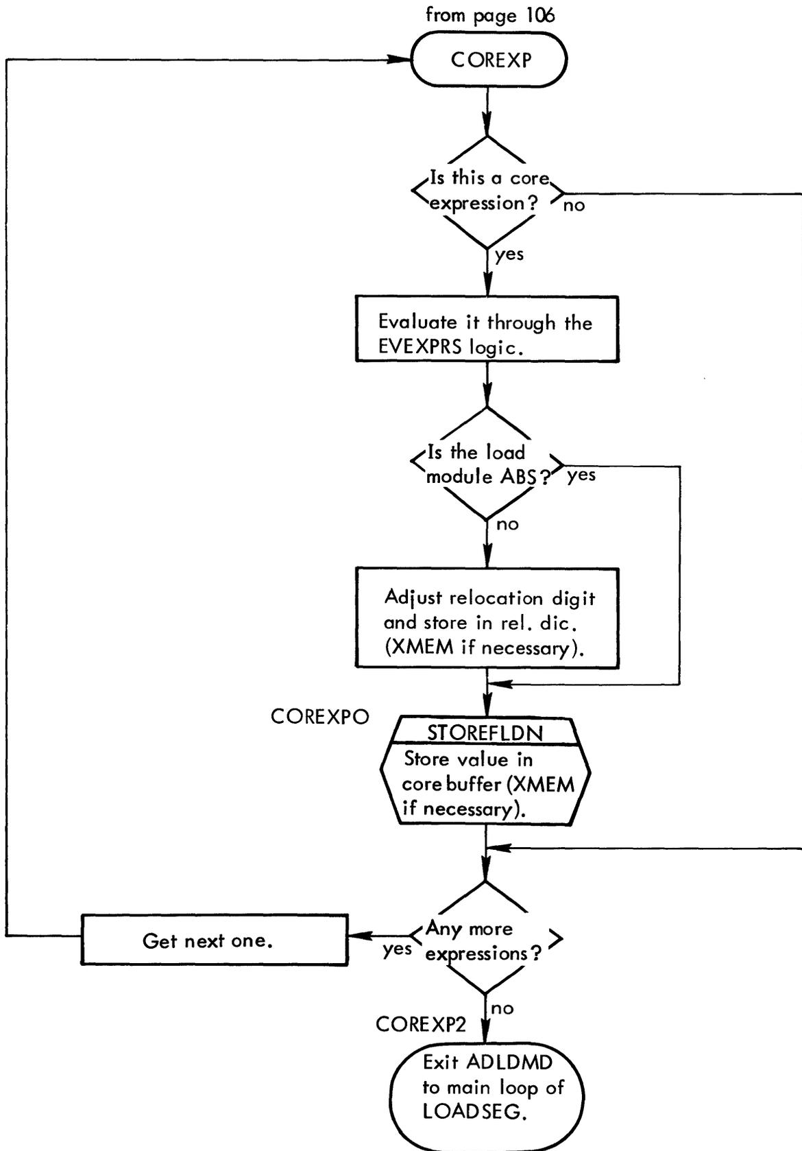
Figure 28. PASS2 Load Module Processor Flow Chart (cont.)
