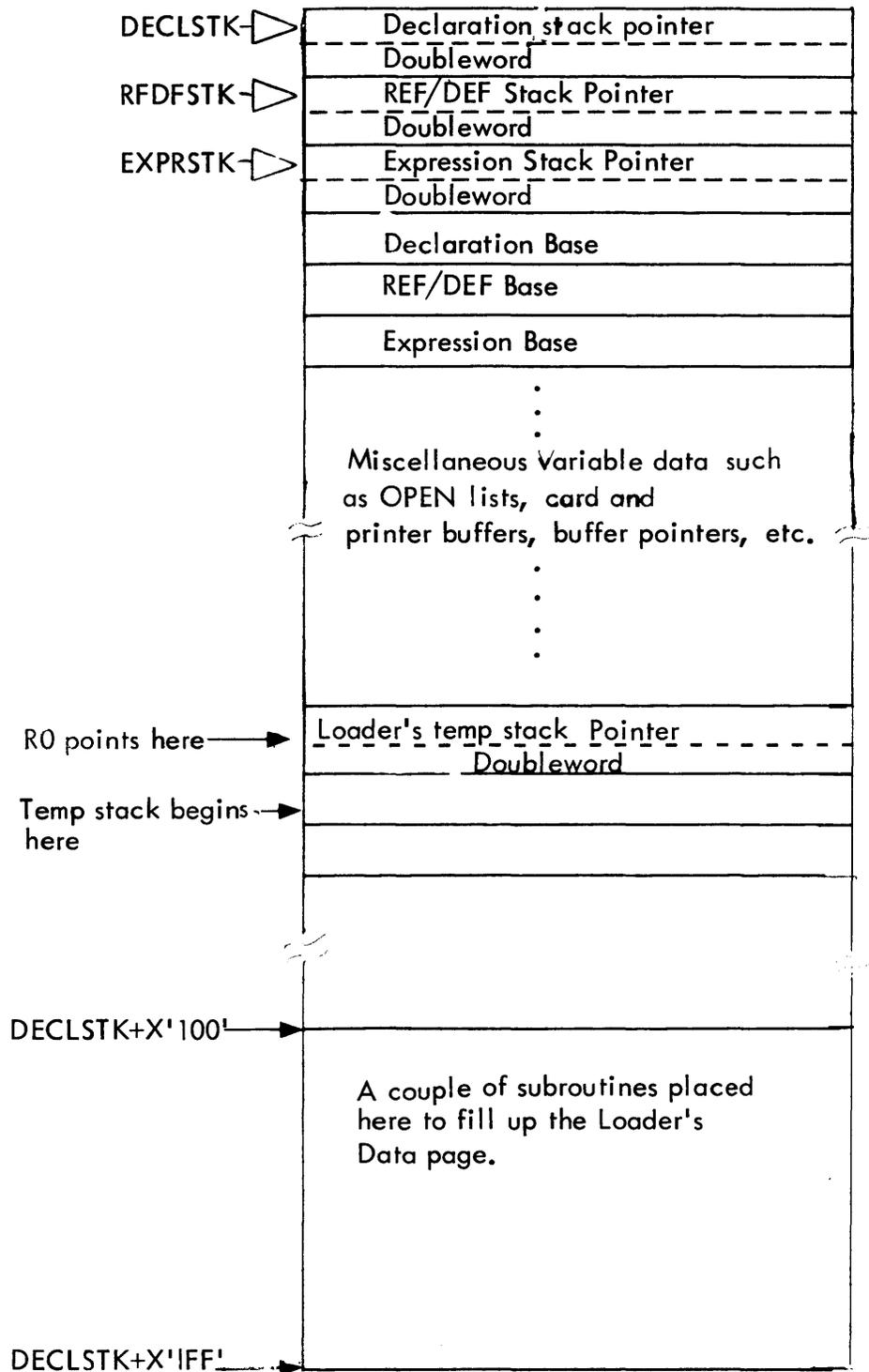
Figure 6. Loader's DATA (00) Area (Within LDR)
