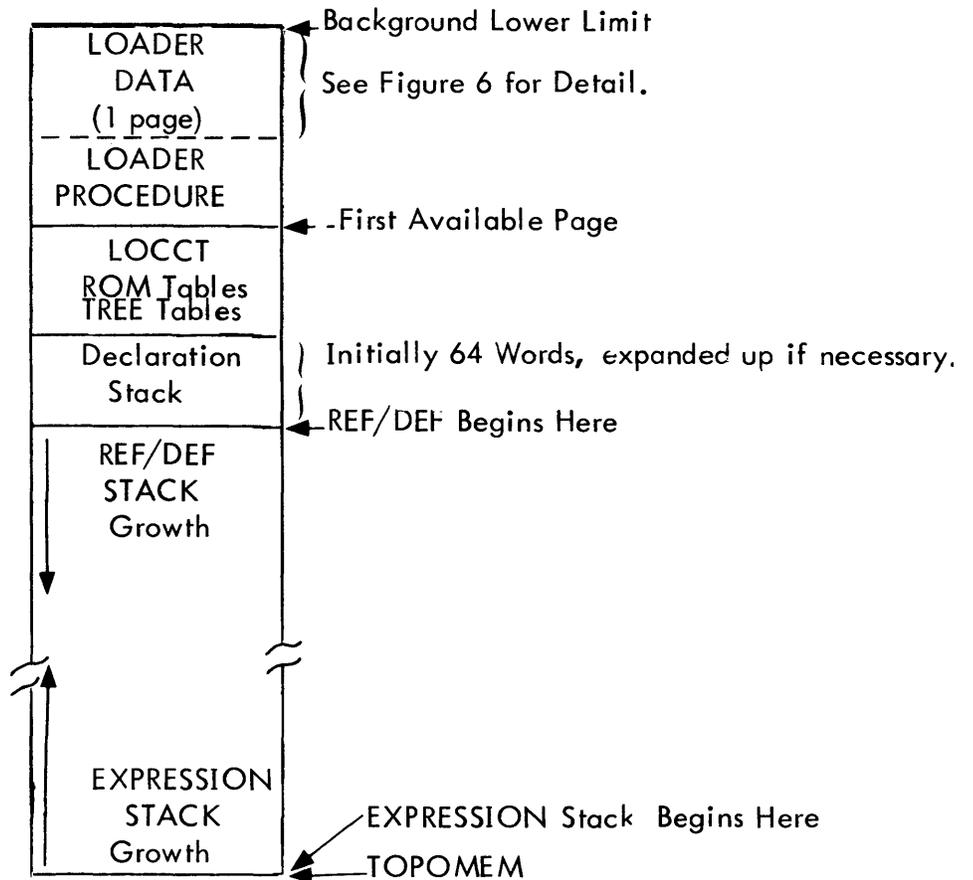
Figure 7. How the Loader Uses Memory: Pass One
