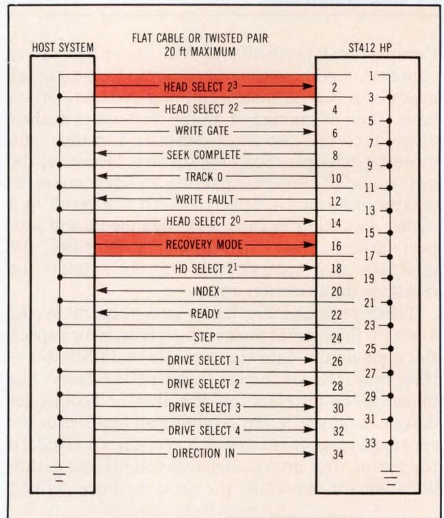
**Fig 2** The control signal connector in the ST412 HP employs two lines that were reserved on the ST506/412 interface: recovery mode and an additional head select. These changes represent the only pinout differences between the two interfaces.
