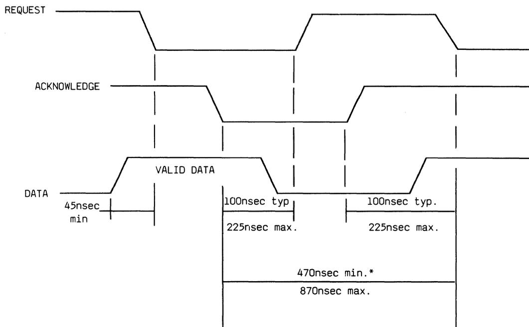
\*Minimum worst case timing assumes Acknowledge is asserted 70nsec prior to internal clock (400nsec)
