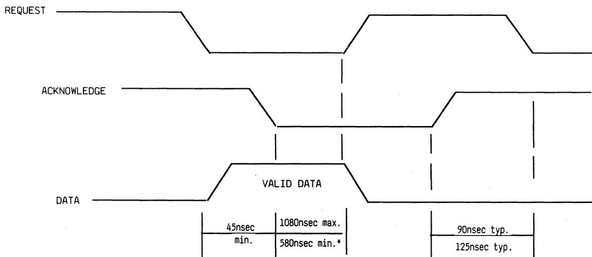
\*Minimum worst case timing assumes Acknowledge is asserted 80nsec prior to internal clock (400nsec).
