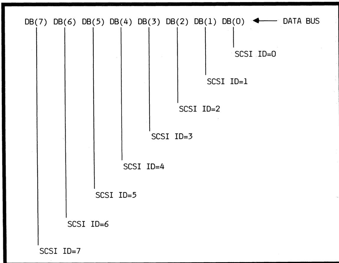
Figure 5: Sample SCSI Configurations
