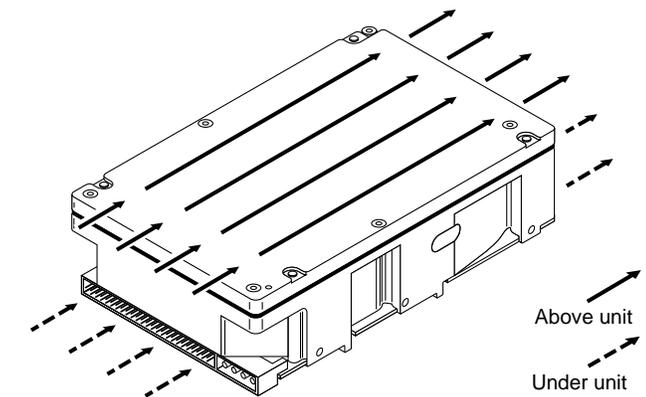
**Note.** Air flows in the direction shown (back to front) or in reverse direction (front to back)
