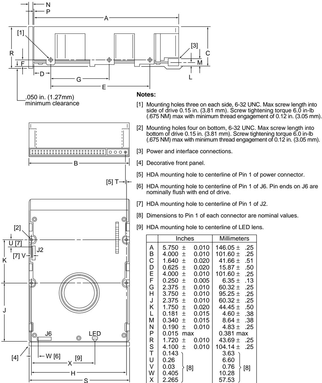
Figure 6. Mounting configuration dimensions for "N" models
