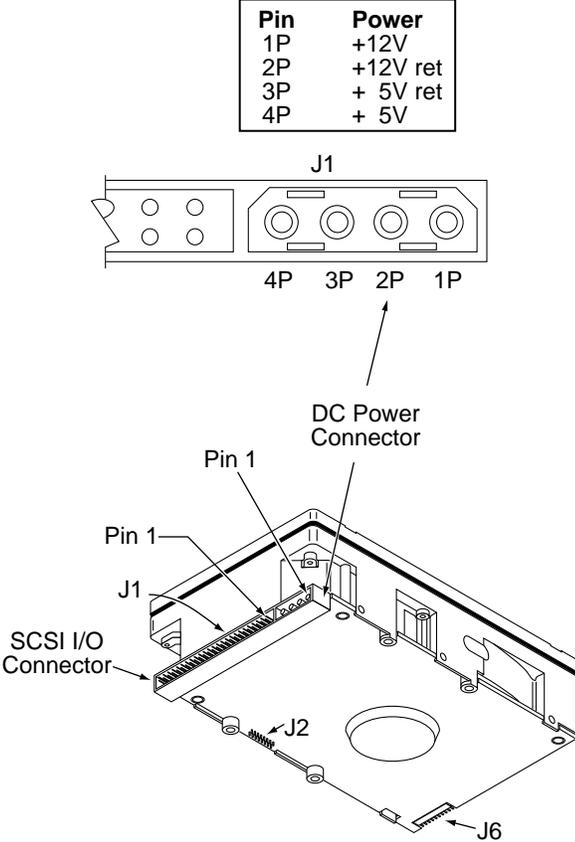
Figure 13. Physical interface for "N" model drives
