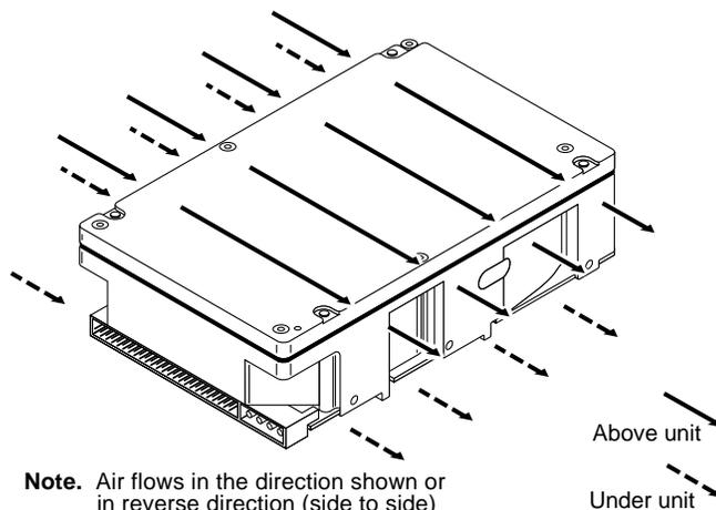
**Note.** Air flows in the direction shown or in reverse direction (side to side)
