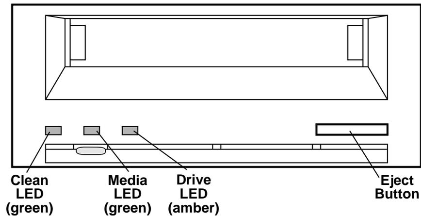
Figure 19. Front Panel of an Internal Drive
