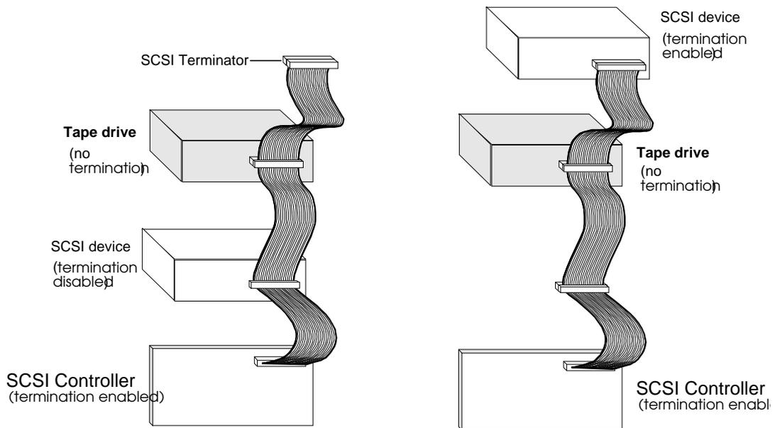
Figure 12. Two SCSI Termination Examples for Internal Drives
