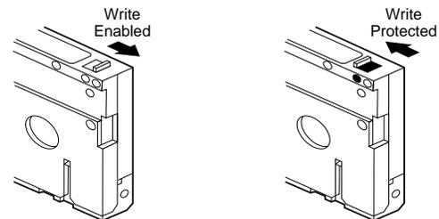
**Figure 23. Write-Protect Tab on the DDS Cartridge**
