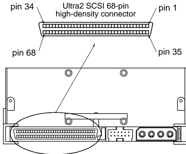
Figure 11. Interface Connector on an Internal Drive
