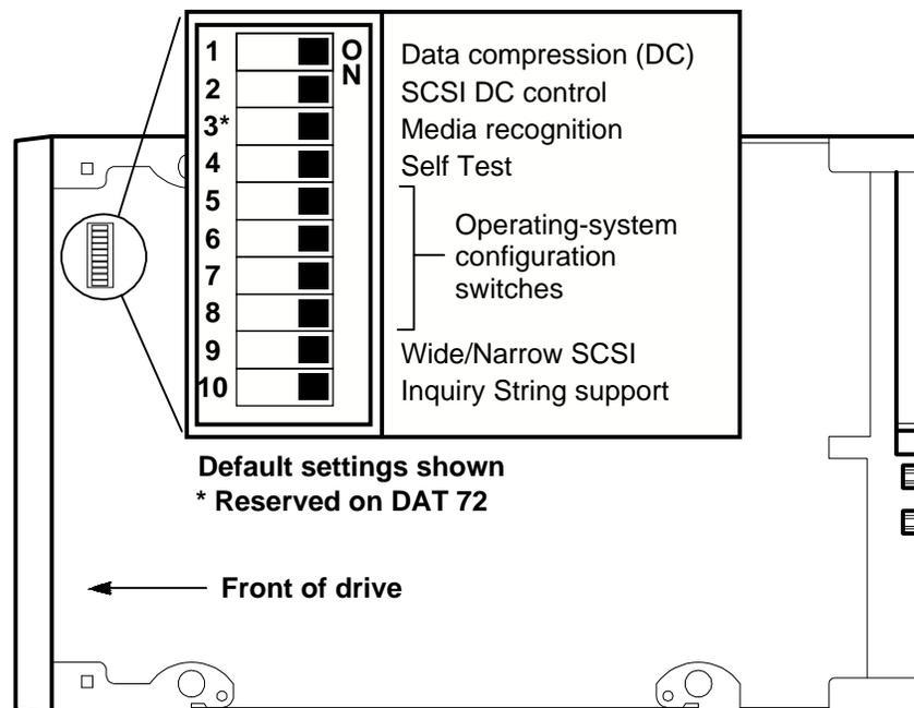
Figure 7. DIP Switch Settings for an Internal Drive
