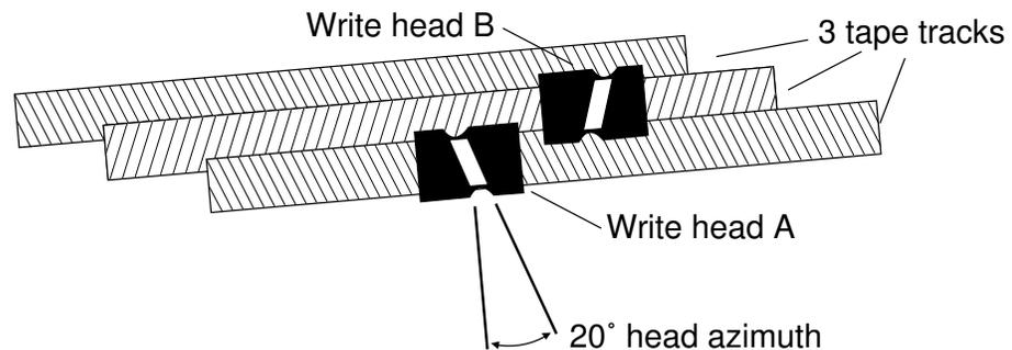
**Figure 21. Alternating Azimuth Angles on Tape Tracks**
