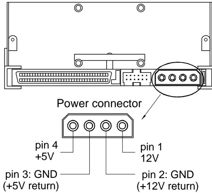
**Figure 13. Power Connector on the internal Drives**
