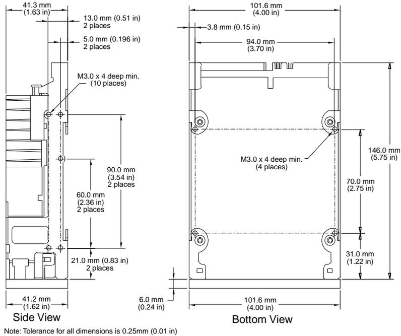
**Figure 4. Internal Drive—Dimensions**
