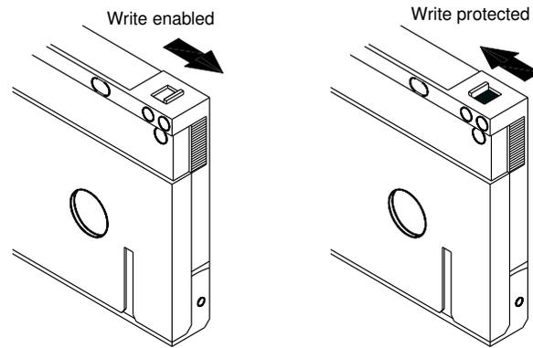
Figure 18. Write-Protect Tab on a DDS Cartridge
