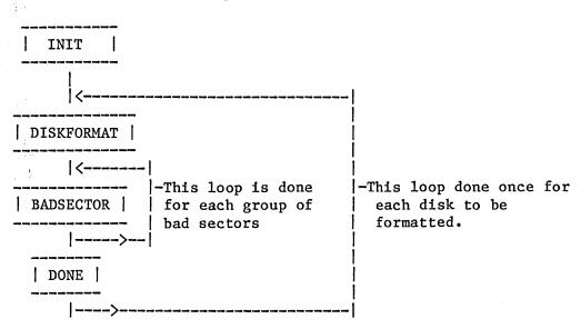
The INIT, DISKFORMAT, and BADSECTOR routines are free to use any MS-DOS system calls, except for file I/O and FAT pointer calls on the disk being formatted. DONE may use ANY calls, since by the time it is called the new disk has been formatted.
