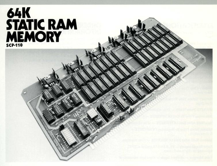
The Seattle Computer 64K Static RAM was designed for system engineers who need fast, highly reliable S-100 memory. To speed system design and integration, the static memory board was developed to be easy to interface with a variety of microprocessors and DMA devices.
