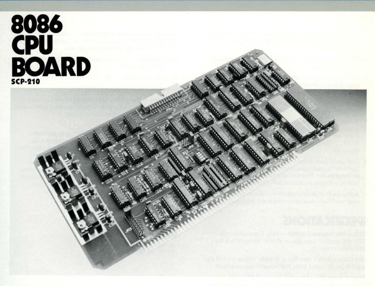
The advanced design of the Seattle Computer 8086 CPU board delivers true 16-bit performance to the S-100 bus. Because of its 16-bit architecture and faster clock rate, it has many times the throughput capabilities of the IBM PC and other 8088 based systems.
