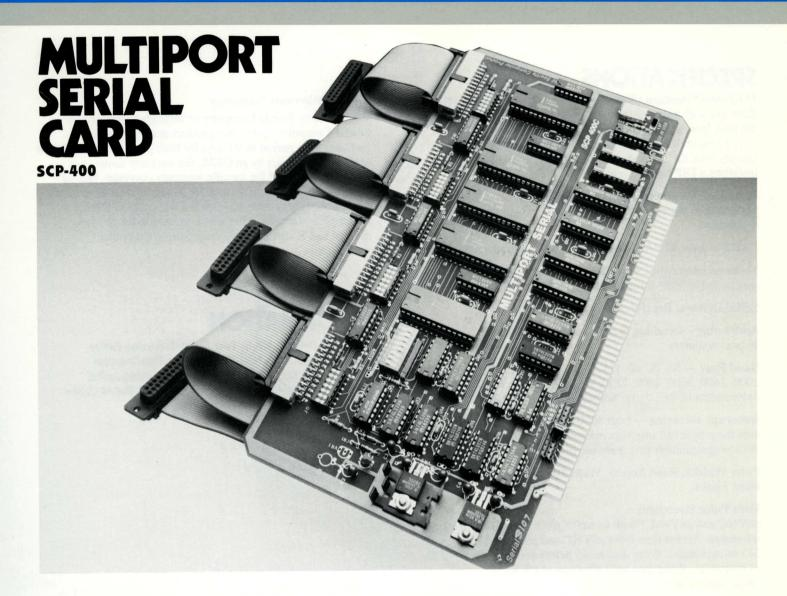
In S-100 (IEEE-696) systems, the Seattle Computer Multiport Serial Card gives designers the option of either two or four RS-232 serial ports per card. The baud rate for each port is independently software programmable. As a result, only one board is necessary to connect low, medium and high speed devices; i.e., printers, modems and terminals. Each port has a configurable shunt block for customizing of handshaking and data lines. This eliminates the need for customized cables.
