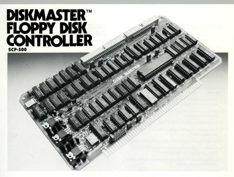
The Seattle Computer DiskMaster™ gives system designers a flexible, high performance floppy disk controller for the S-l00 (IEEE-696) bus. The DiskMaster supports both 8″ and 5.25″ floppy disk drives.
