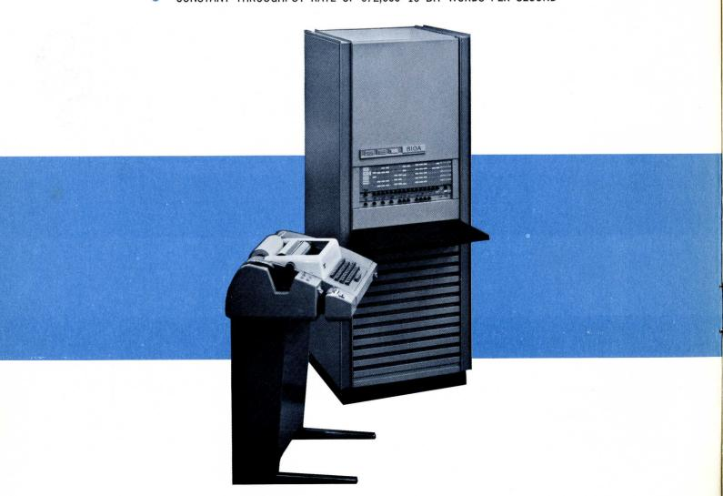
THE SEL 810A GENERAL PURPOSE 16-BIT PARALLEL COMPUTER HAS THE HIGHEST THROUGHPUT RATE OF ANY MACHINE IN ITS SIZE AND PRICE CLASS. IN ADDITION TO FULFILLING REQUIREMENTS FOR VERSATILE HIGH SPEED COMPUTATION, THE SEL 810A PROVIDES SYSTEM CAPABILITIES DEVELOPED THROUGH EXTENSIVE SEL EXPERIENCE IN THE DATA ACQUISITION AND CONTROL FIELDS. A COMPREHENSIVE INPUT/OUTPUT CONFIGURATION PRODUCES THE FLEXIBILITY NECESSARY FOR SEL 810A USE IN THESE APPLICATIONS:
