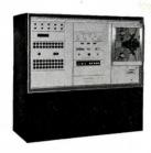
SEL MAGNETIC CORE MEMORY SYSTEMS provide capacity ranges from 128 to 8192 words per basic unit, and word size acording to customer requirement. Standard addressing types available are random access, sequential, sequential / interlace. Combinations of types are also available.
