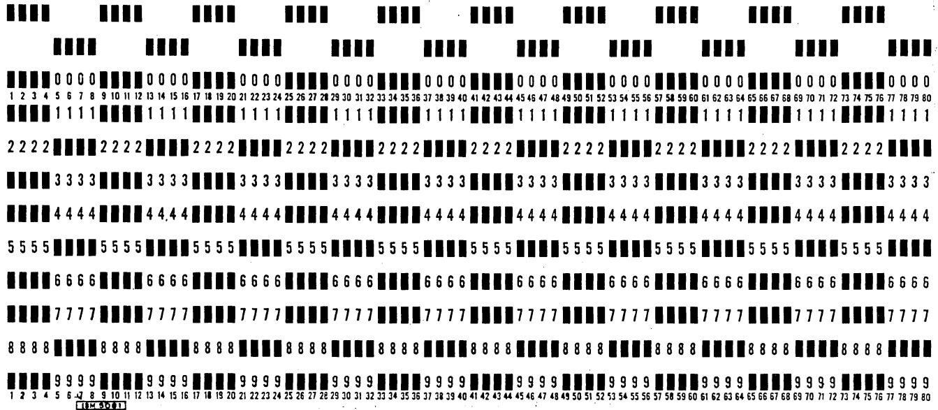
2. The card shown below is an image of the BCD card needed for this program when performing the stored card BCD test. Program storage is in locations 00414<sub>8</sub> through 00533<sub>8</sub>.
