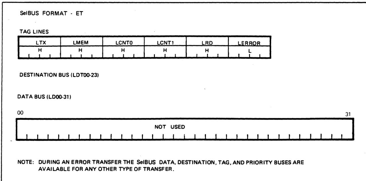
Figure 3-6. Error Transfer (ET) Format
