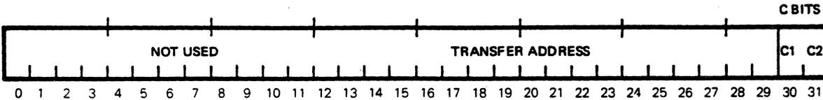
Figure 2-3. Input/Output Command Doubleword (IOCD) Format
