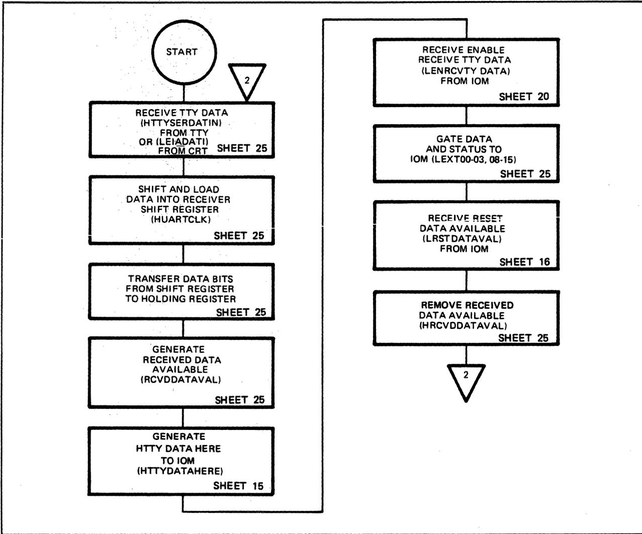
Figure 3-14. Input Data Transfer (TTY)
