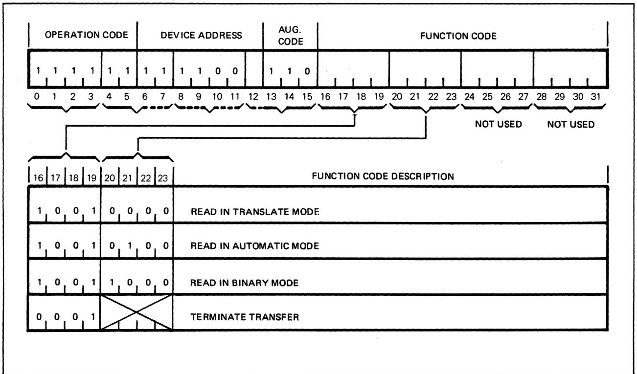
Figure 2-12. Card Reader Command Device Instruction Format
