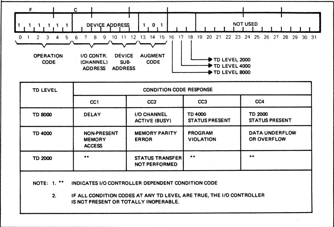
Figure 2-5. Test Device (TD) Instruction Format
