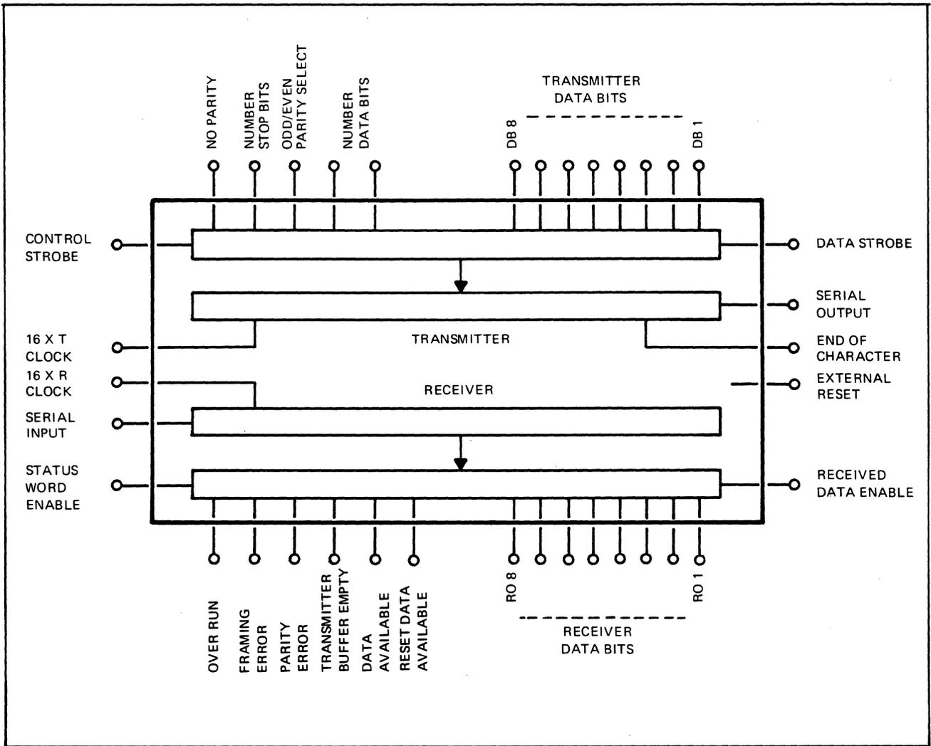
Figure 3-10. Block Diagram - Universal Asynchronous Receiver/Transmitter (UART)
