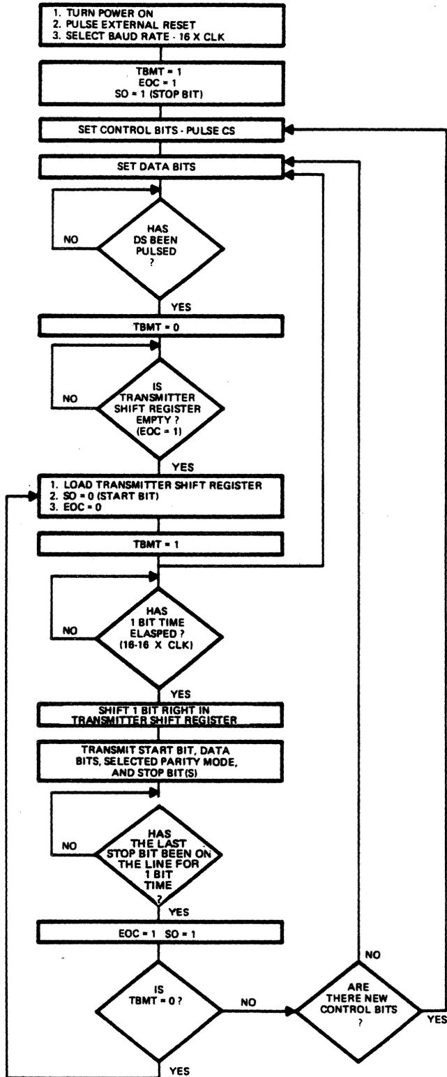
Figure 3-11. UART - Transmitter Flow Diagram
