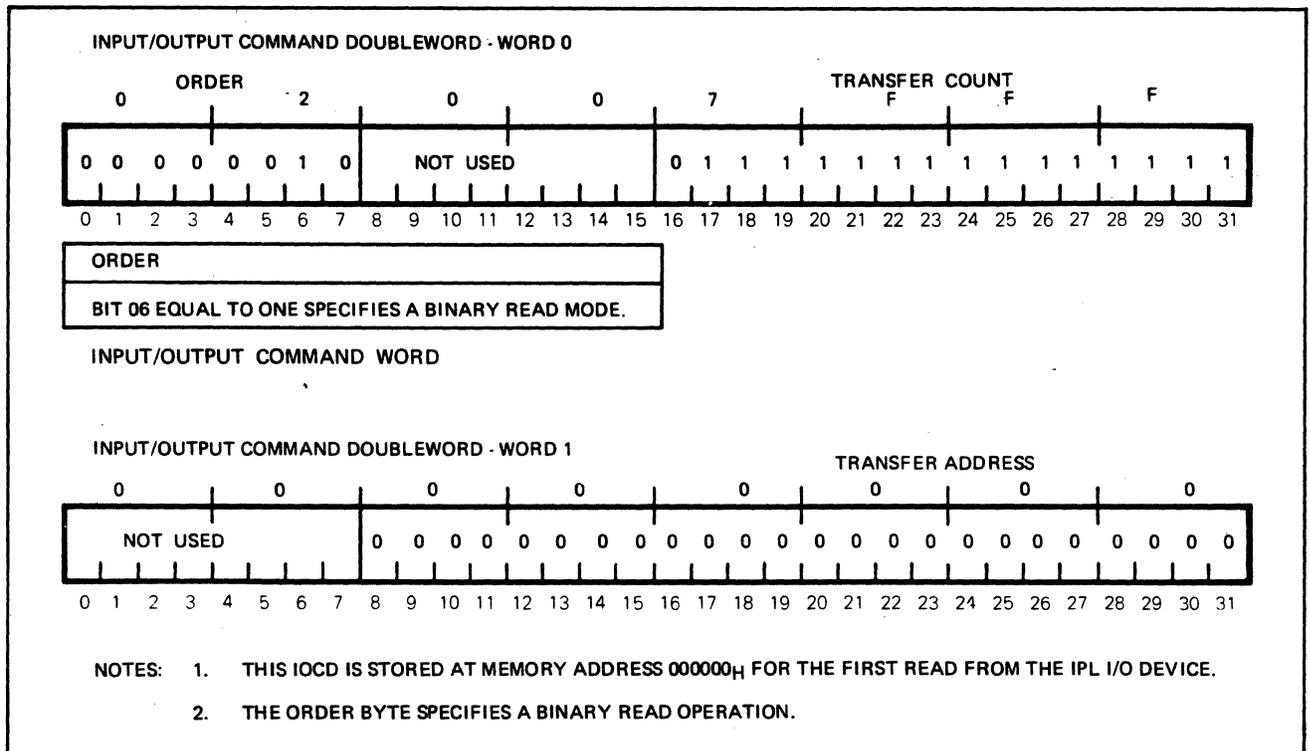
Figure 2-4. IPL Basic Input/Output Command Doubleword (IOCD) Format
