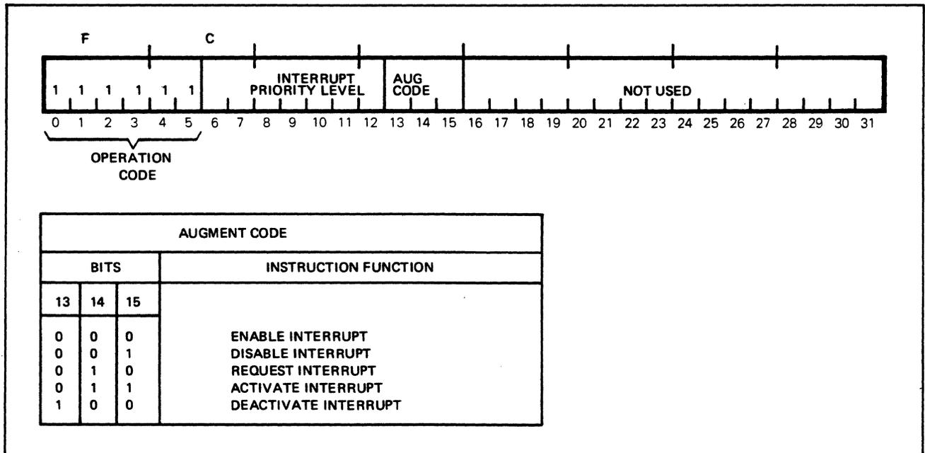
Figure 2-6. Interrupt Control Instruction Format
