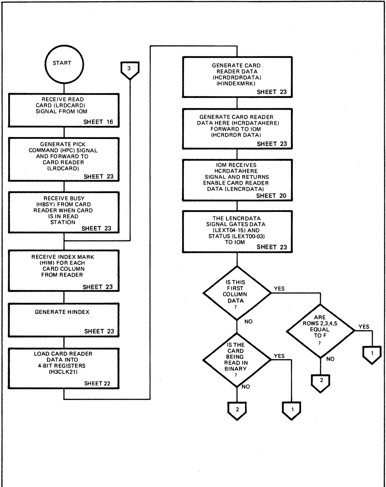
Figure 3-20. Card Reader Operation (Sheet 1 of 2)
