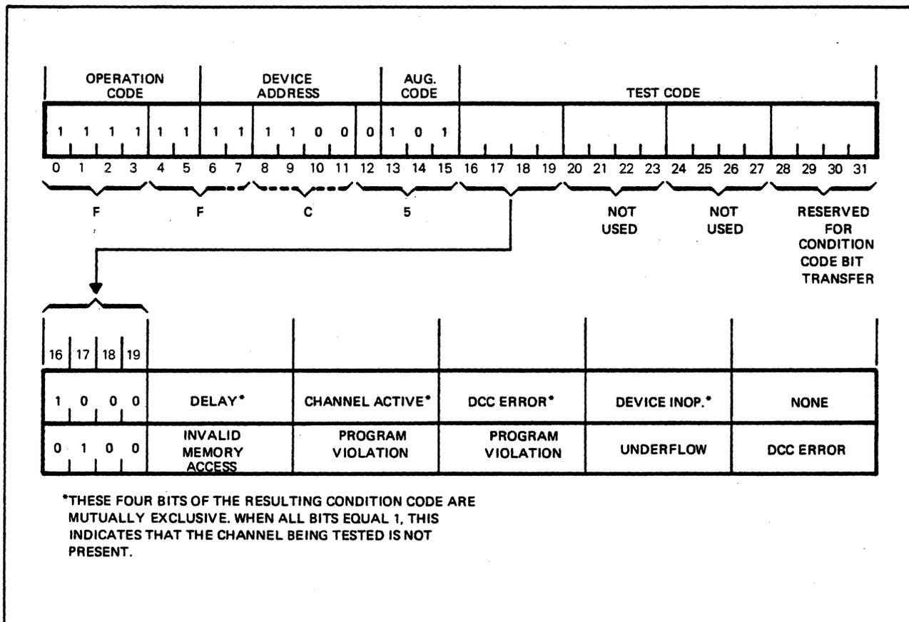
Figure 2-13. Card Reader Test Device Instruction Format
