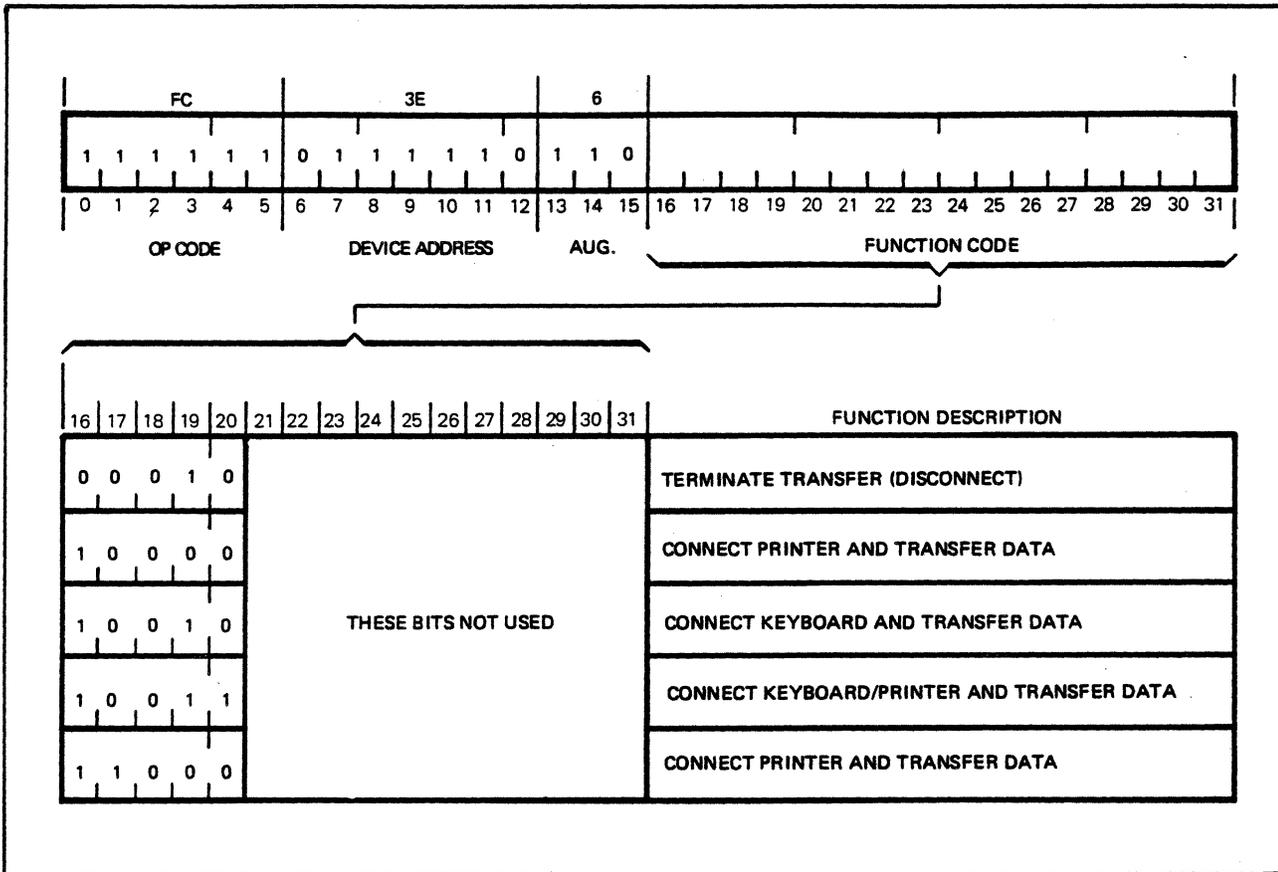
Figure 2-8. Command Device Format TTY System
