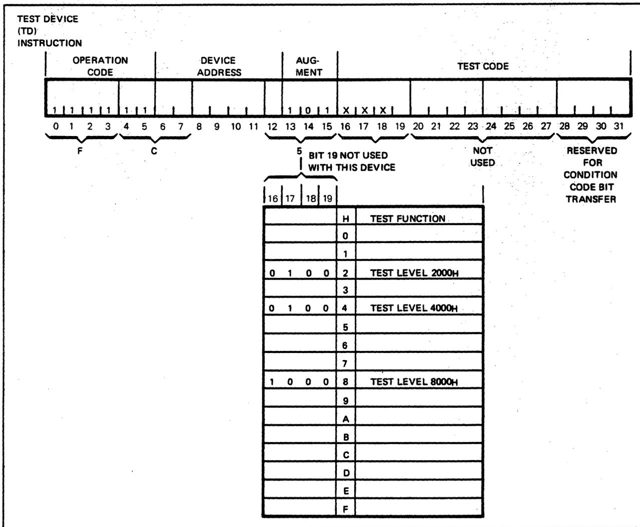
Figure 2-11. Line Printer Test Device Instruction Format
