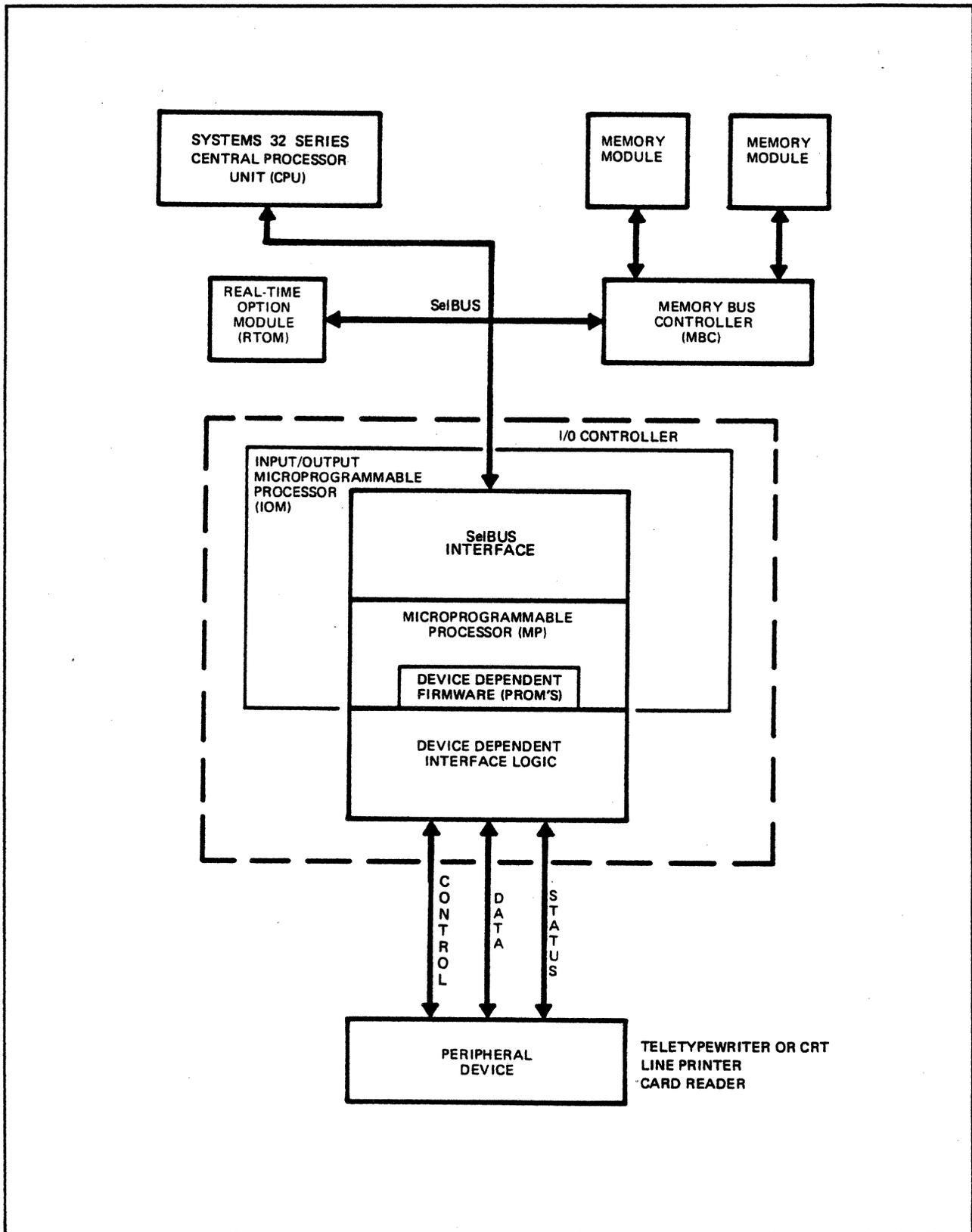
Figure 3-1. Block Diagram - SYSTEMS 32 SERIES Computer
