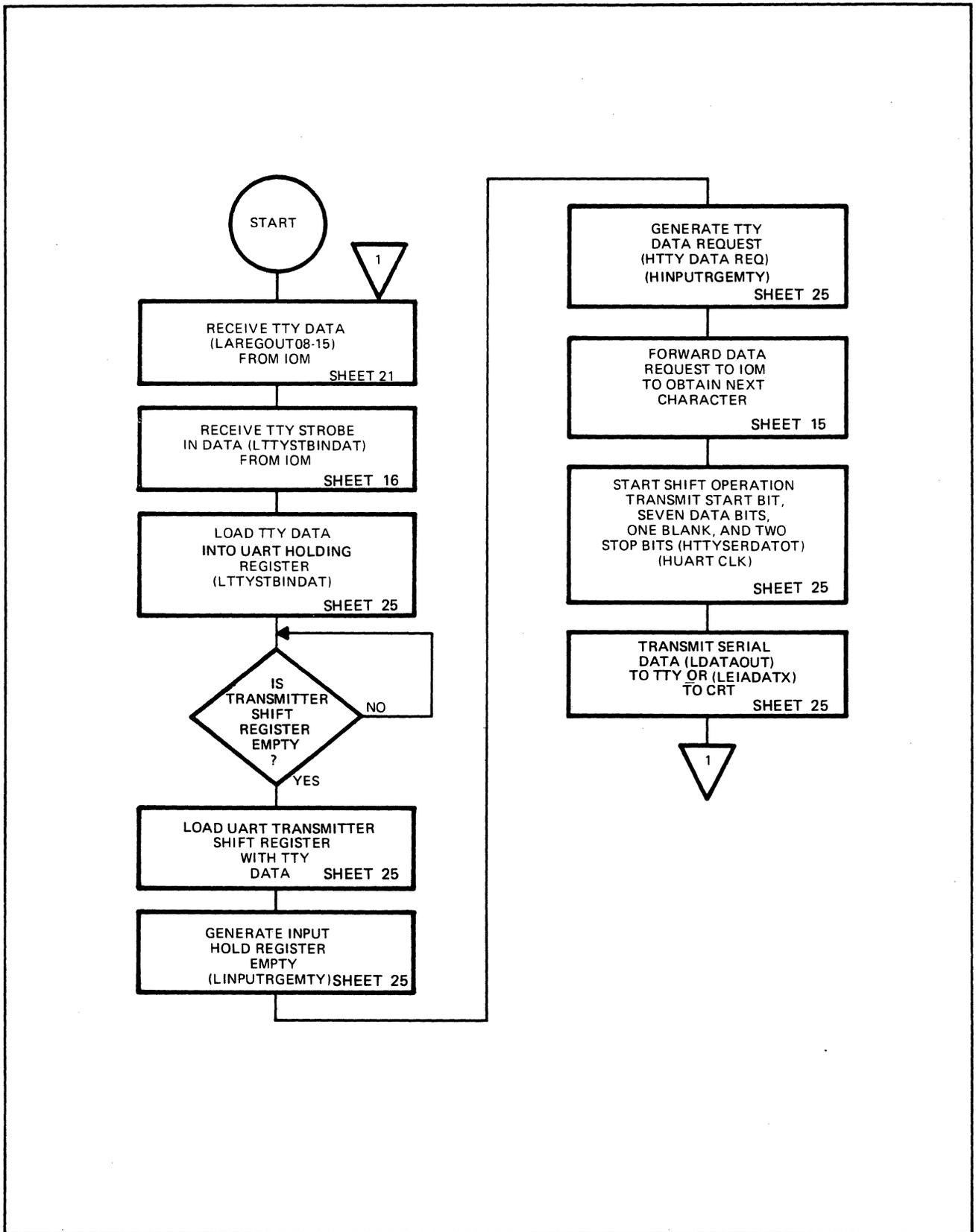
Figure 3-13. Output Data Transfer (TTY)
