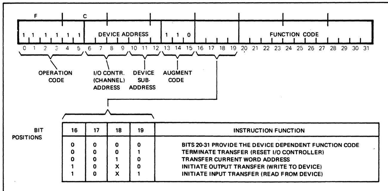
Figure 2-1. Command Device (CD) Instruction Format
