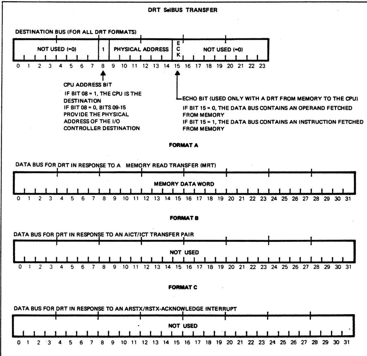
Figure 3-5. Data Return Transfer (DRT) Format (Sheet 1 of 2)
