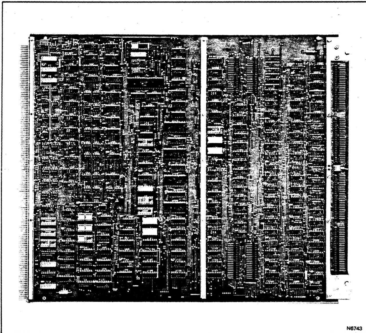
Figure 1-1. Copper TLC Controller
