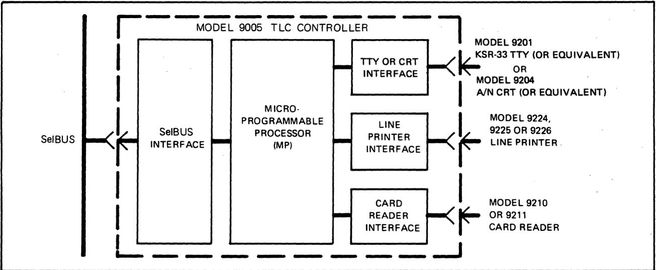
Figure 1-2. Block Diagram - TLC Controller
