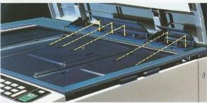
The sensor uses mirrors to read sizes optically (the light waves appear solely for illustration).
