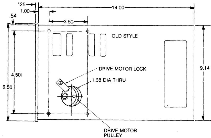
Figure 20 Standard Mount Physical Dimensions
