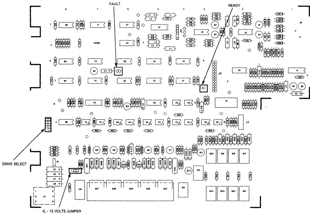
Figure 22 SA1000 Control PCB
