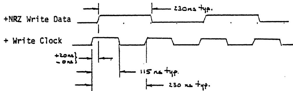
Figure 9. MFM ENCODE TIMING
