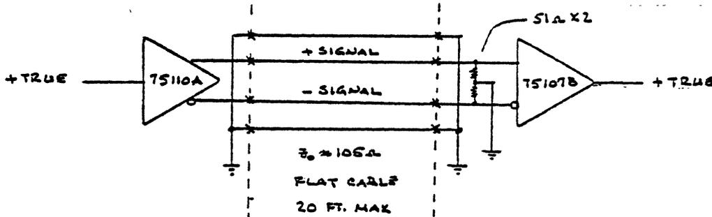
Figure 6. DATA LINE DRIVER/RECEIVER (POSITION LOGIC)
