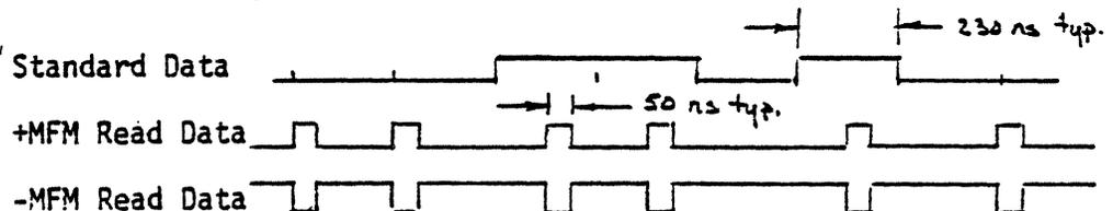
Figure 8. MFM READ DATA TIMING
