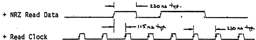
Figure 10. NRZ READ DATA DECODE TIMING
