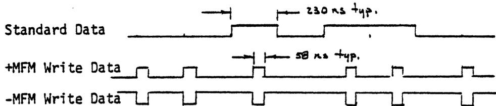
Figure 7. MFM WRITE DATA TIMING
