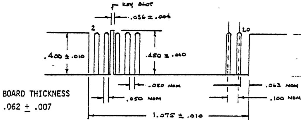
Figure 1. J1, J2, J3, and J4 CONNECTOR DIMENSIONS
