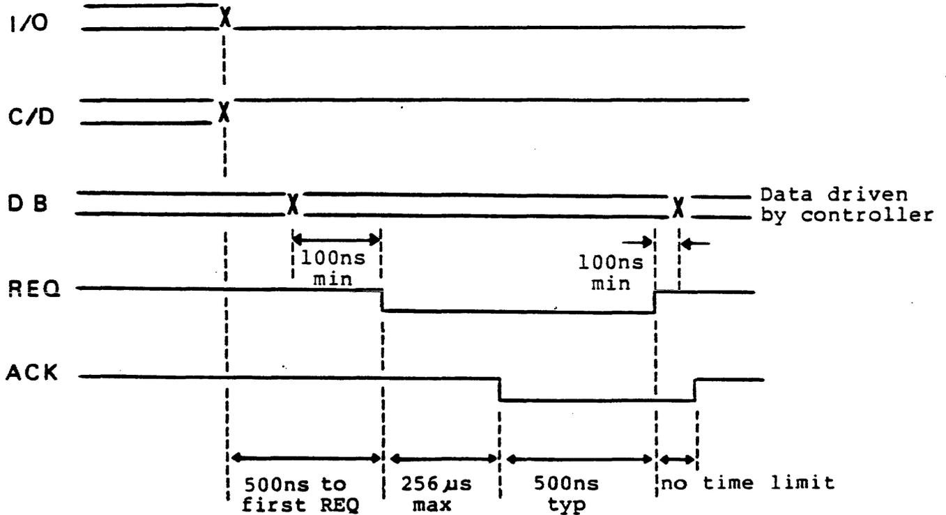
Note 1: For Status Byte Transfer (I/O, C/D asserted and MSG deasserted); or Interrupt Byte Transfer (MSG, I/O, C/D asserted), REQ is asserted 500ns (typical) after the assertion of any of the above bits.
