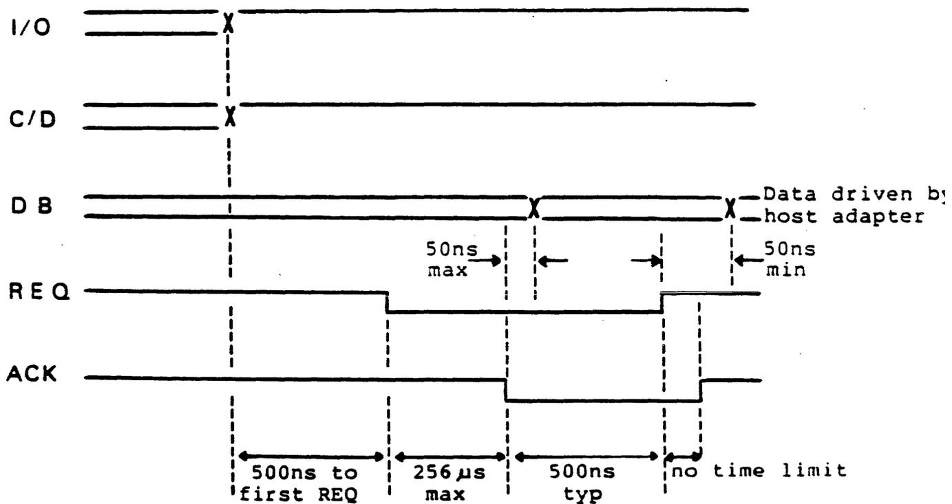
Note 1: Data driven by the host adapter is stable 50ns max at the host adapter end after ACK is asserted, and 50ns min after REQ is deasserted.
