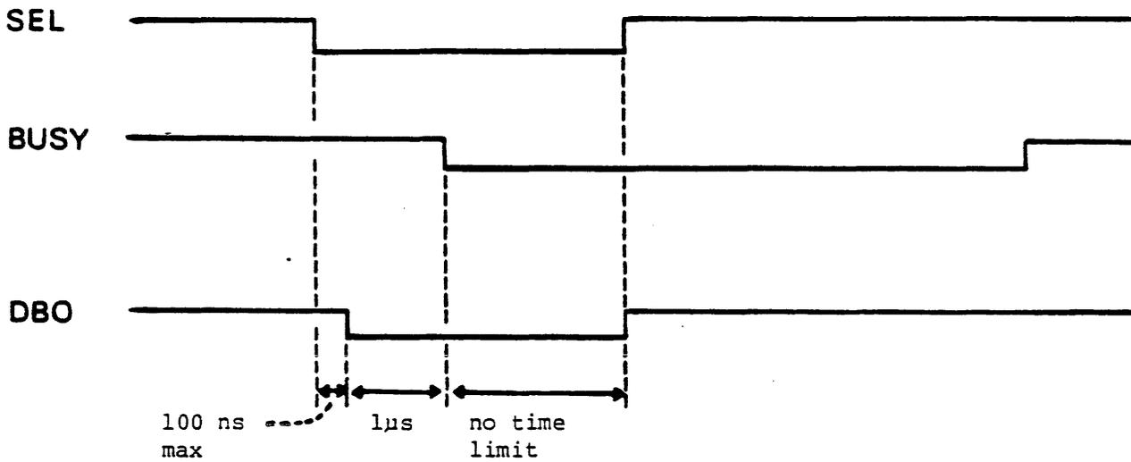
Note: SEL must be deasserted before the controller will assert REQ.
