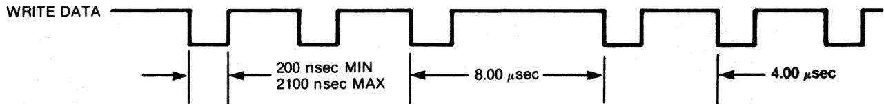
FIGURE 1-10. WRITE DATA TIMING (FM)
