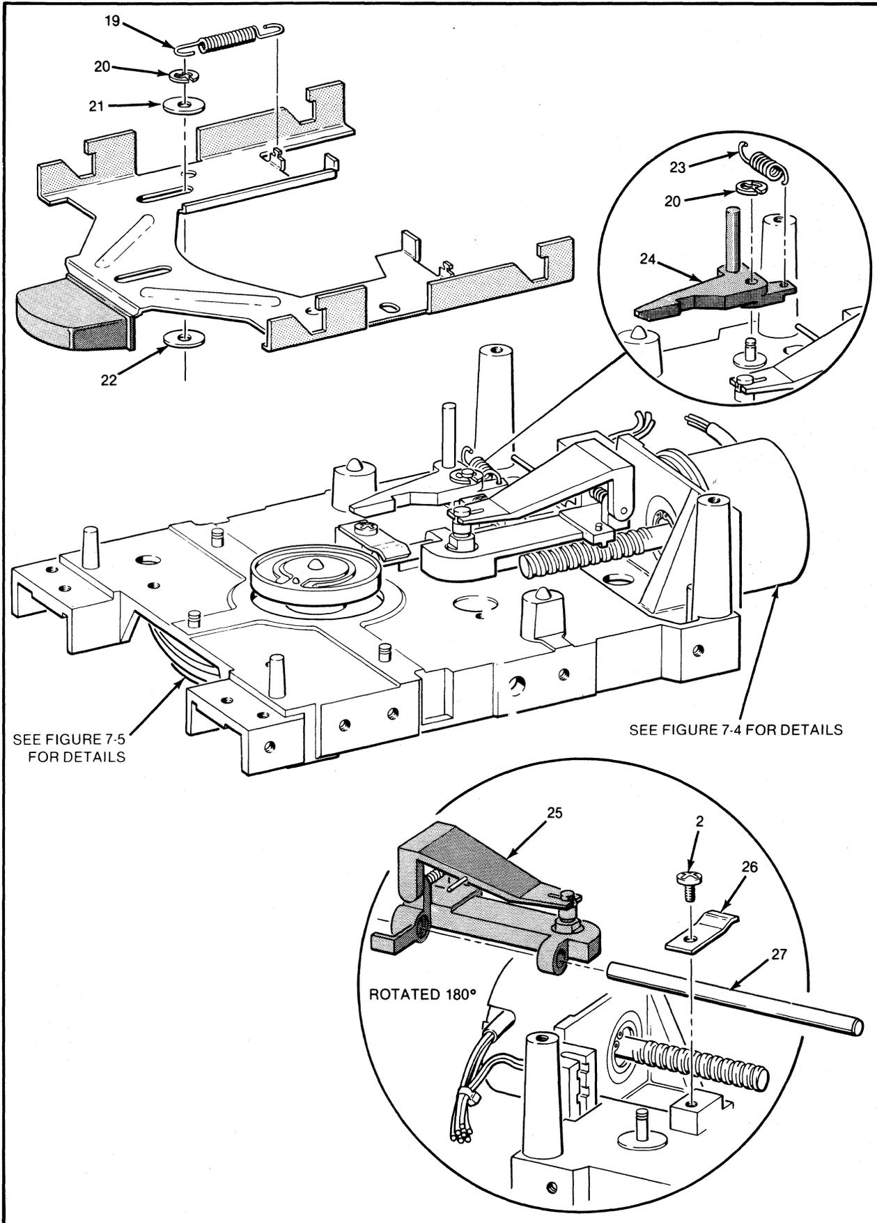
**FIGURE 7-3. EJECTOR HEAD AND CARRIAGE ASSEMBLY**
