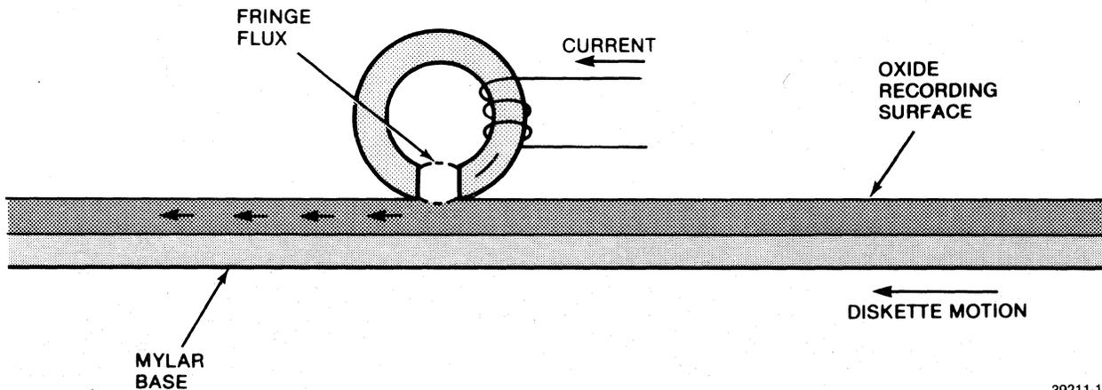
FIGURE 4-2. BASIC READ/WRITE HEAD
