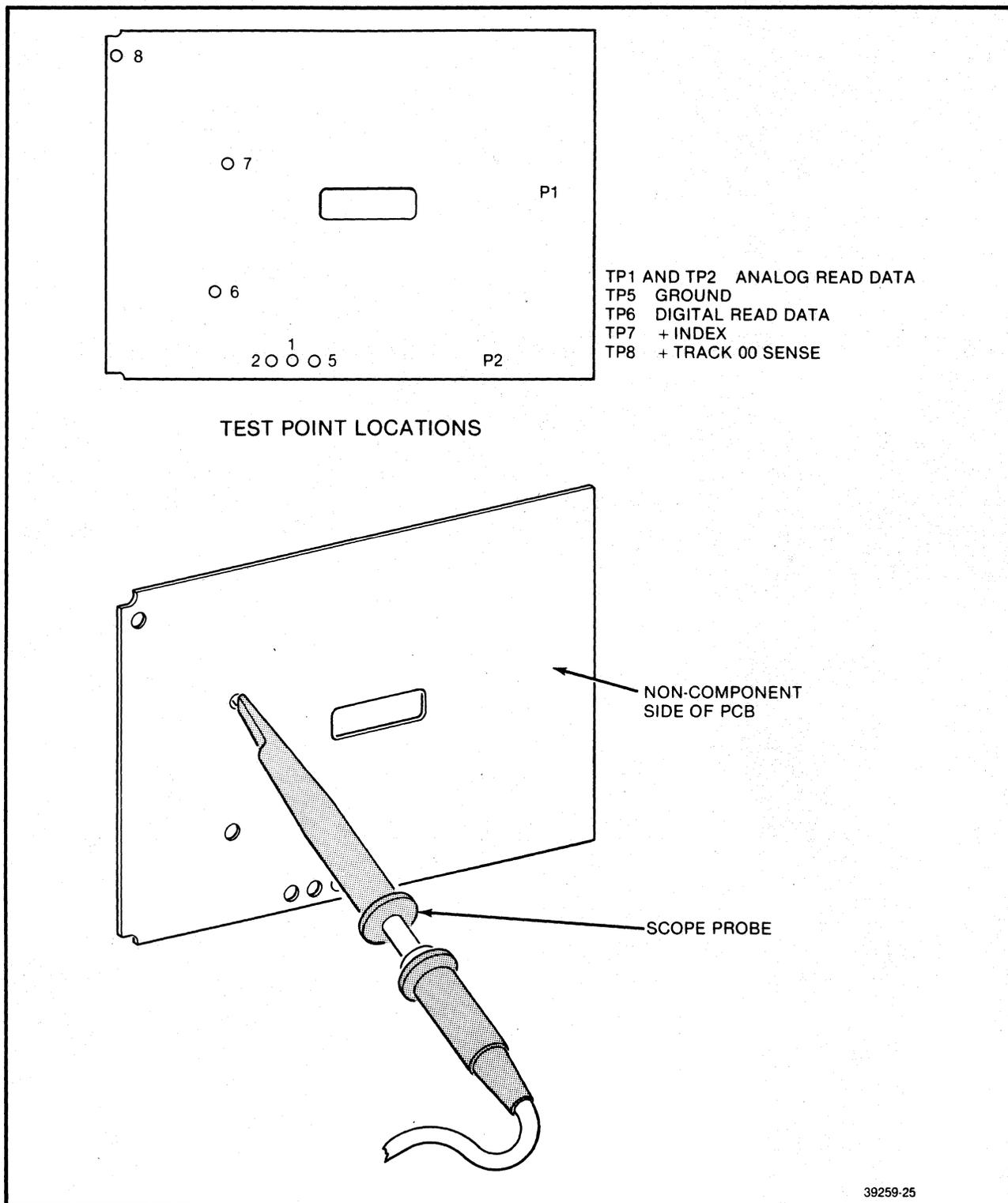
FIGURE 5-6. TEST POINT LOCATIONS AND PROBE POSITIONING
