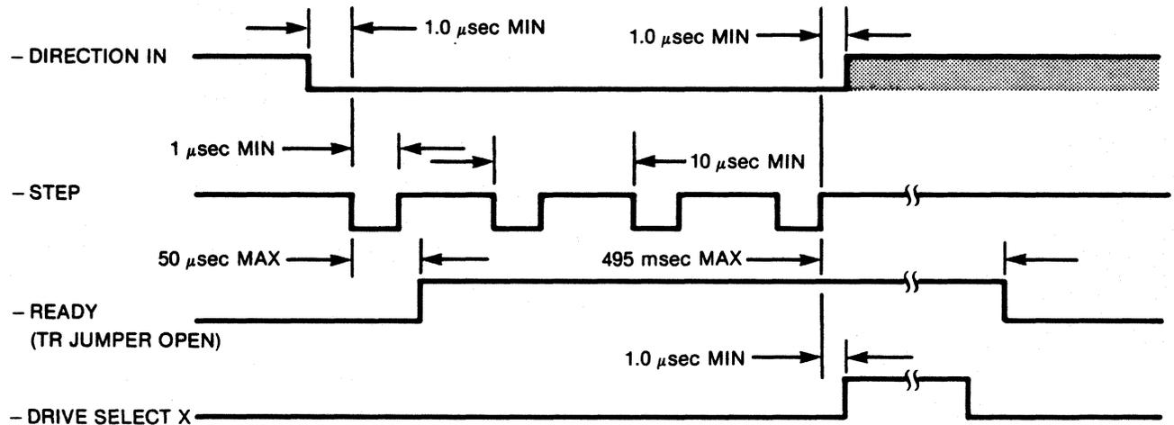
FIGURE 1-5. BUFFERED STEP MODE
