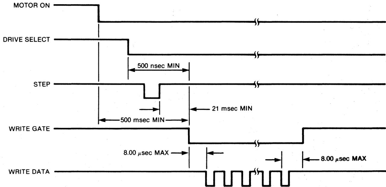
FIGURE 1-9. WRITE INITIATE TIMING
