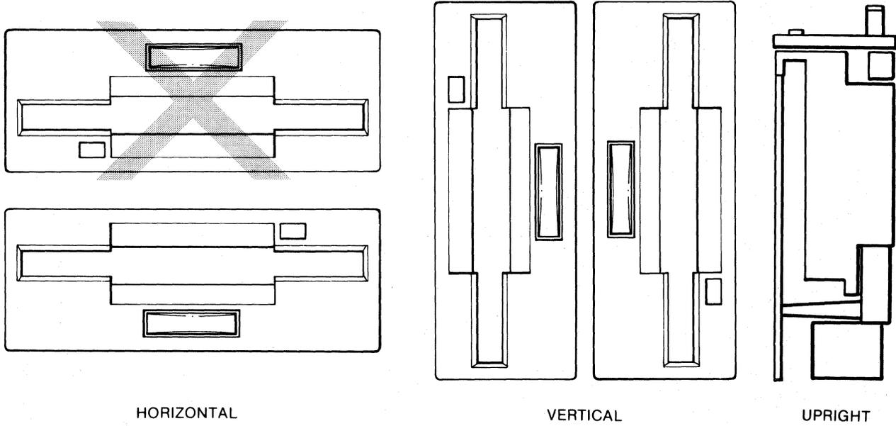
**FIGURE 1-13. RECOMMENDED MOUNTING POSITIONS**
