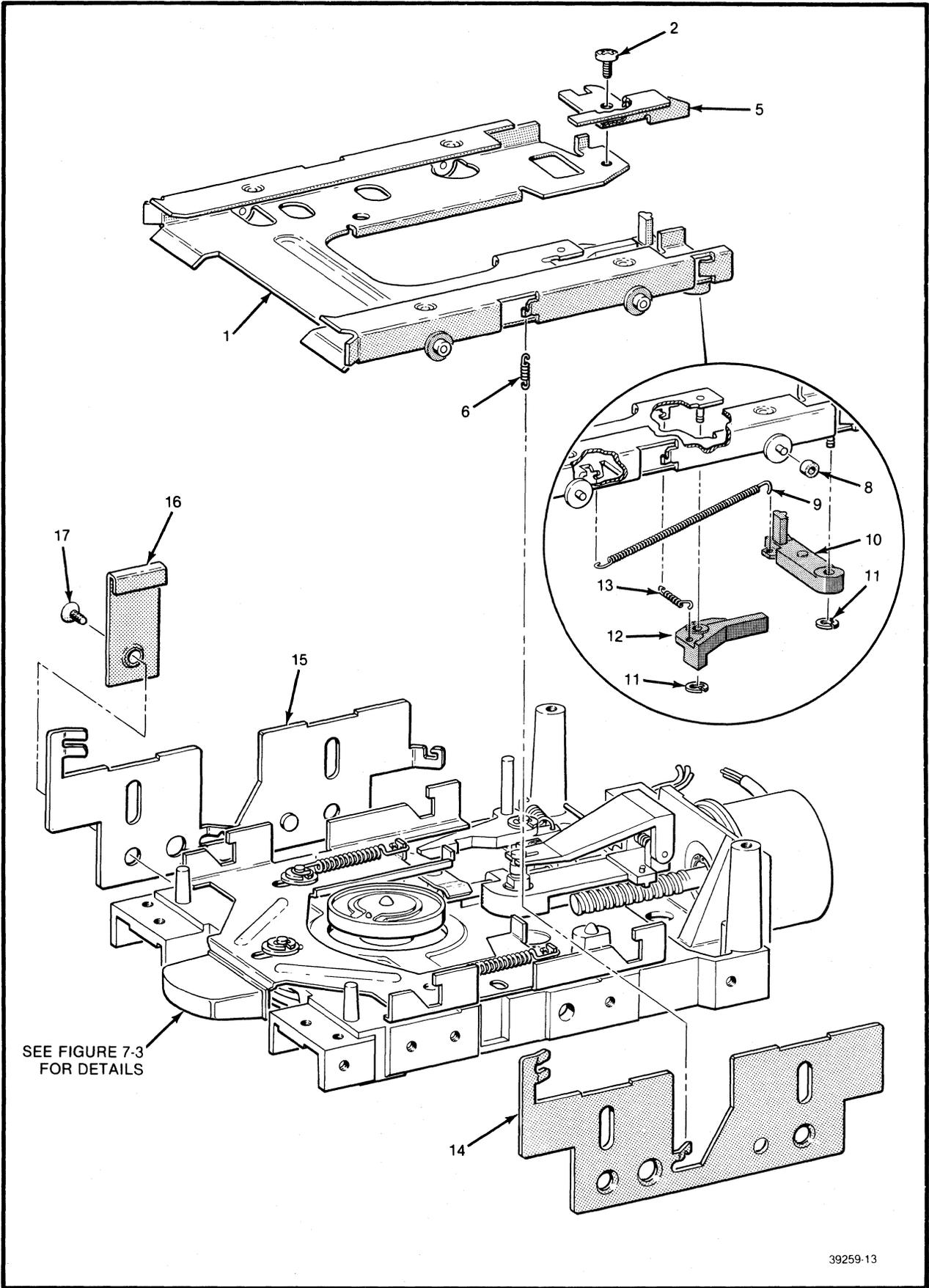
**FIGURE 7-2. PLATFORM EJECTOR/ELEVATOR ASSEMBLY**
