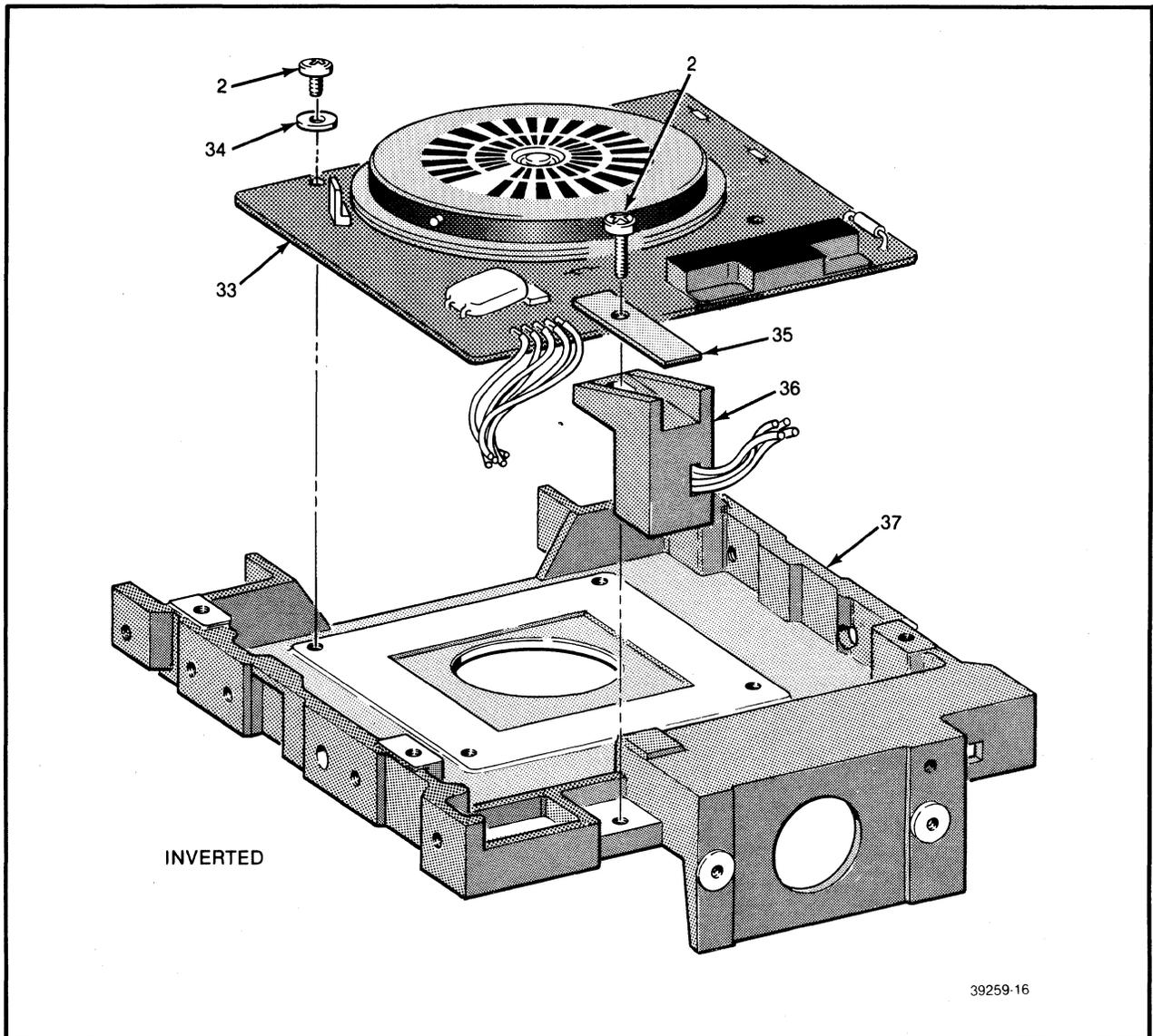
**FIGURE 7-5. BRUSHLESS SPINDLE MOTOR, TK 0 AND ELEVATOR DETECTOR ASSEMBLY**
