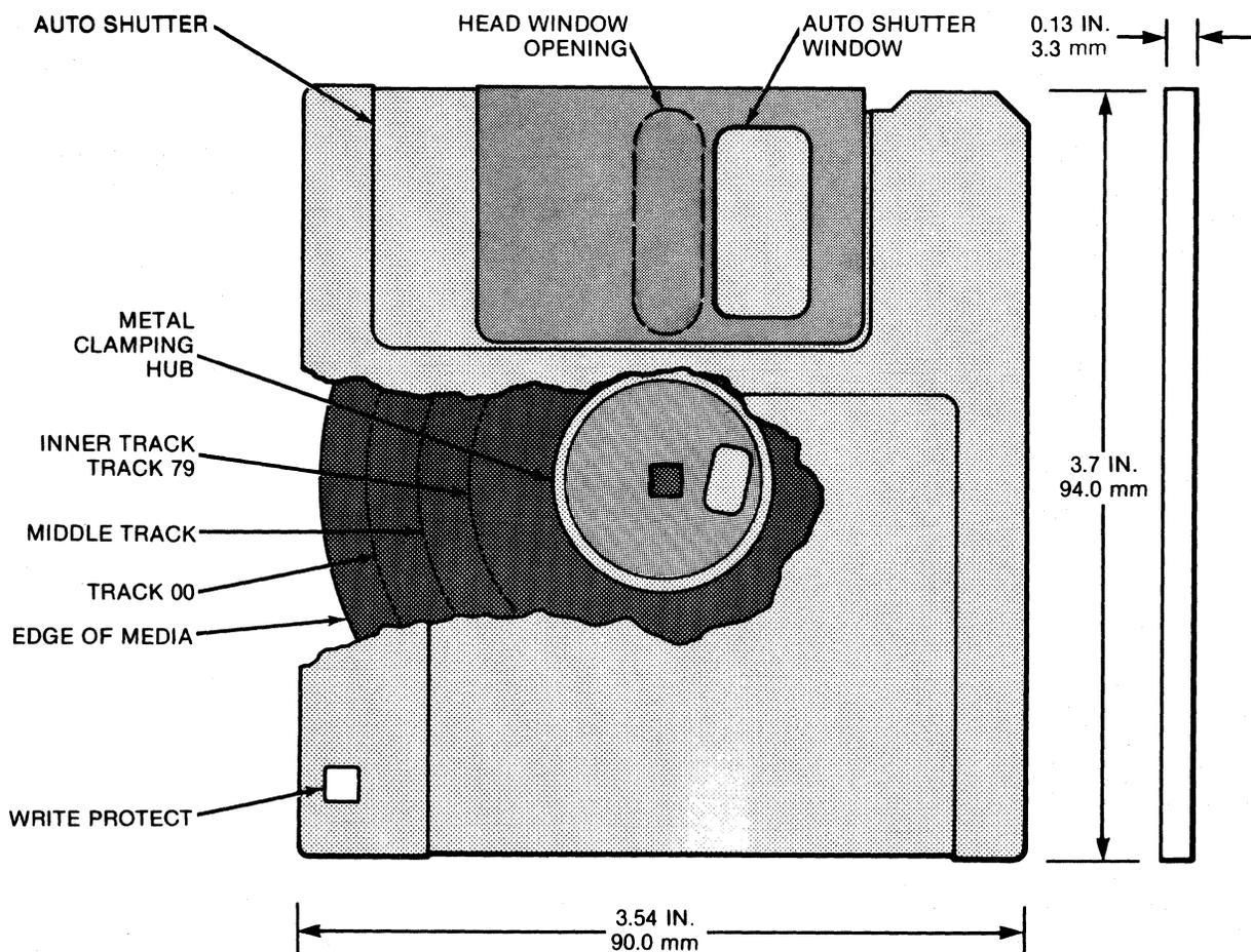
FIGURE 1-12. SA130 MICROCARTRIDGE NOMENCLATURE
