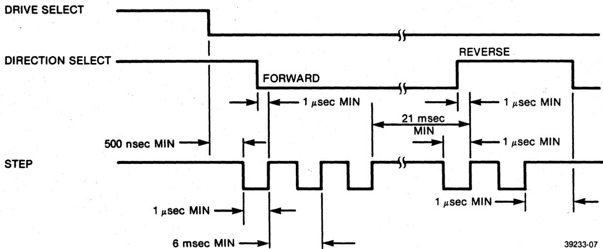
FIGURE 1-3. TRACK ACCESS TIMING
