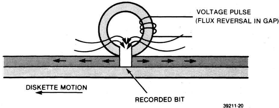
FIGURE 4-4. READING A BIT
