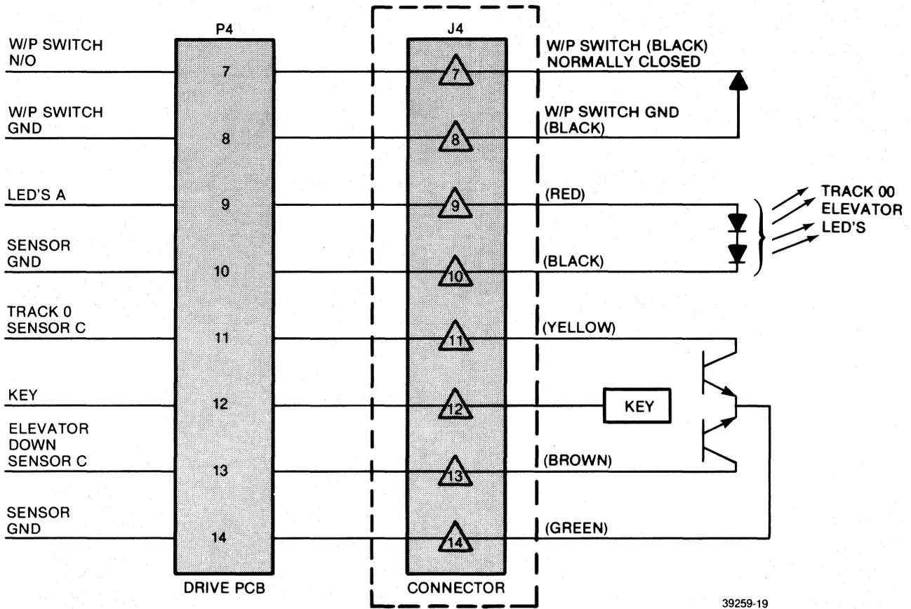
FIGURE 10-1. WRITE PROTECT — TRACK 00 — ELEVATOR DOWN SENSOR CONNECTIONS
