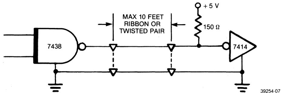
FIGURE 2-2. INTERFACE SIGNAL DRIVER/RECEIVER
