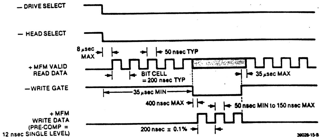
FIGURE 2-10. MFM READ/WRITE DATA TIMING
