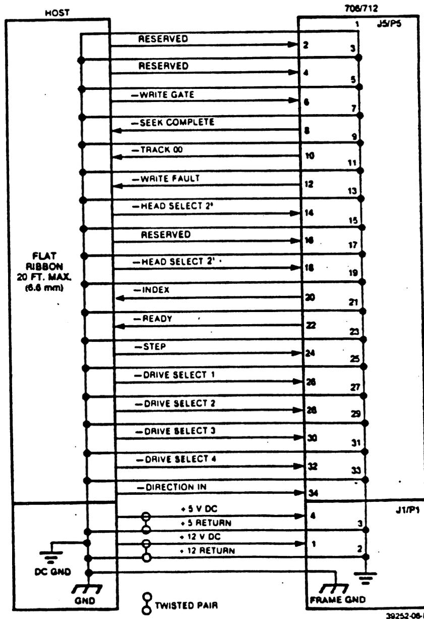
★ FIGURE 2-1. J5 INTERFACE AND J1 POWER CONNECTIONS
