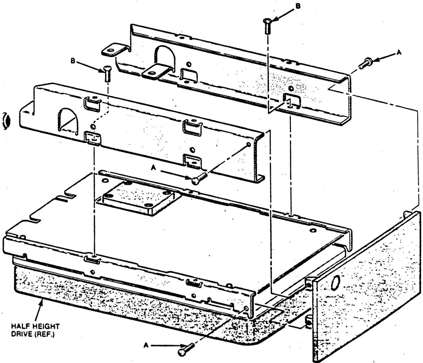
TORQUE SCREWS, B, TO 10 IN.-LBS.
