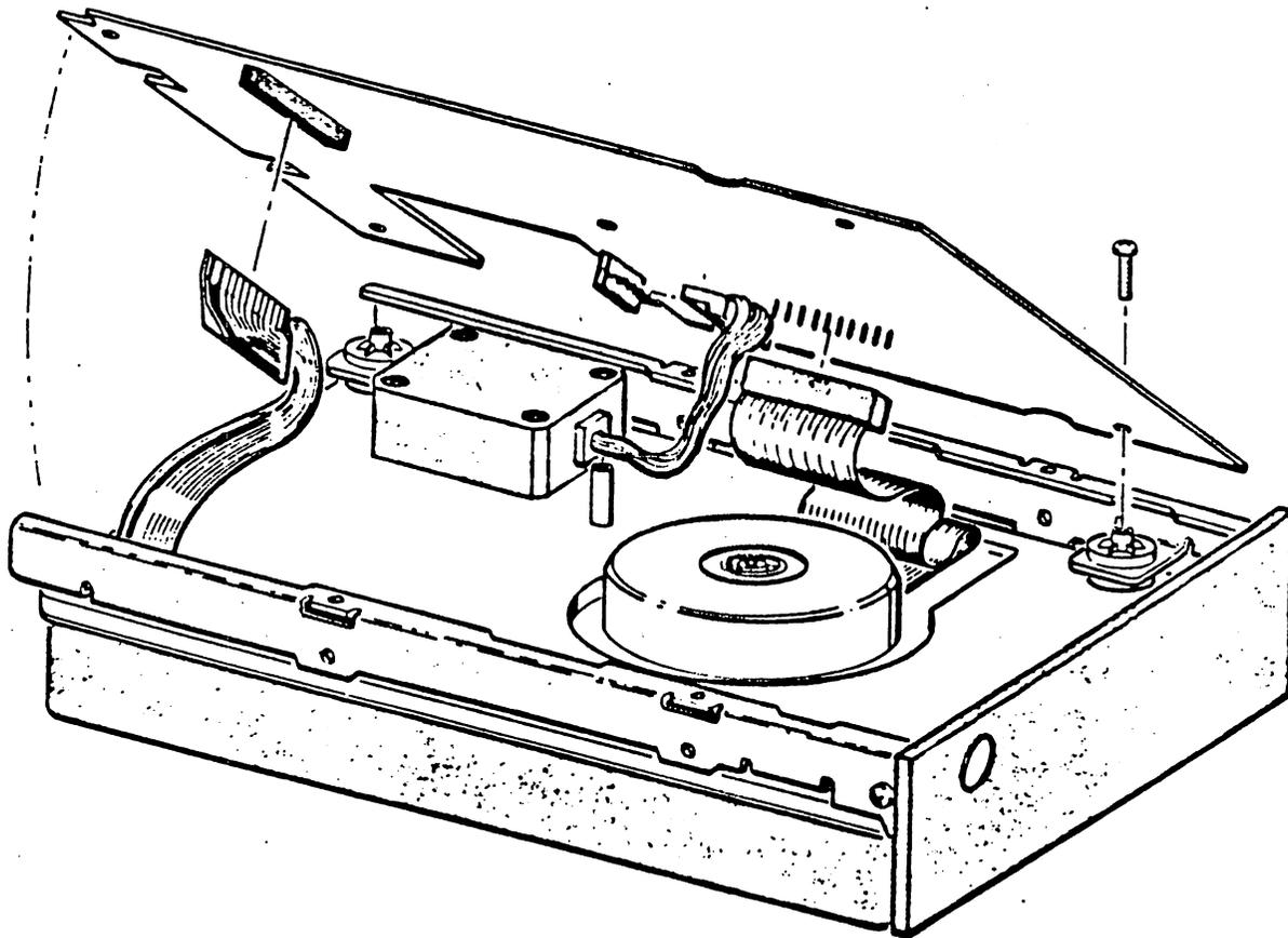
FIGURE 12-2. REMOVAL/REPLACEMENT OF CONTROL PCB
