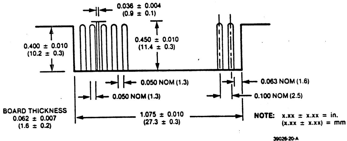
FIGURE 3-4. J6 CONNECTOR DIMENSIONS
