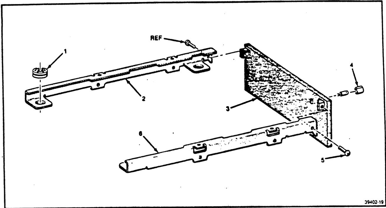
FIGURE 13-2. FRONT PANEL AND RAIL ASSEMBLY
