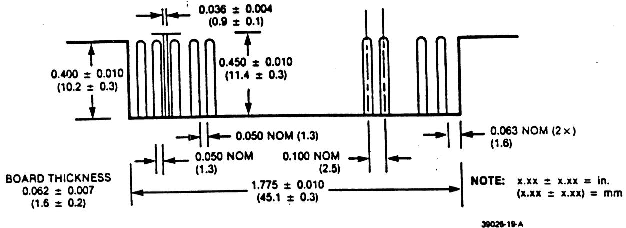
FIGURE 3-3. J5 CONNECTOR DIMENSIONS
