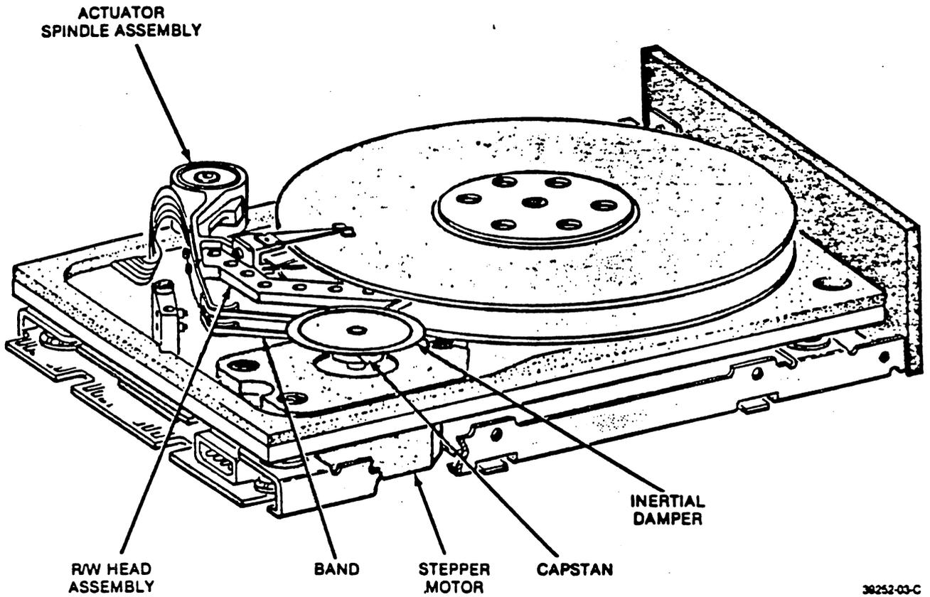
★ FIGURE 1-2. READ/WRITE HEAD POSITIONING MECHANISM
