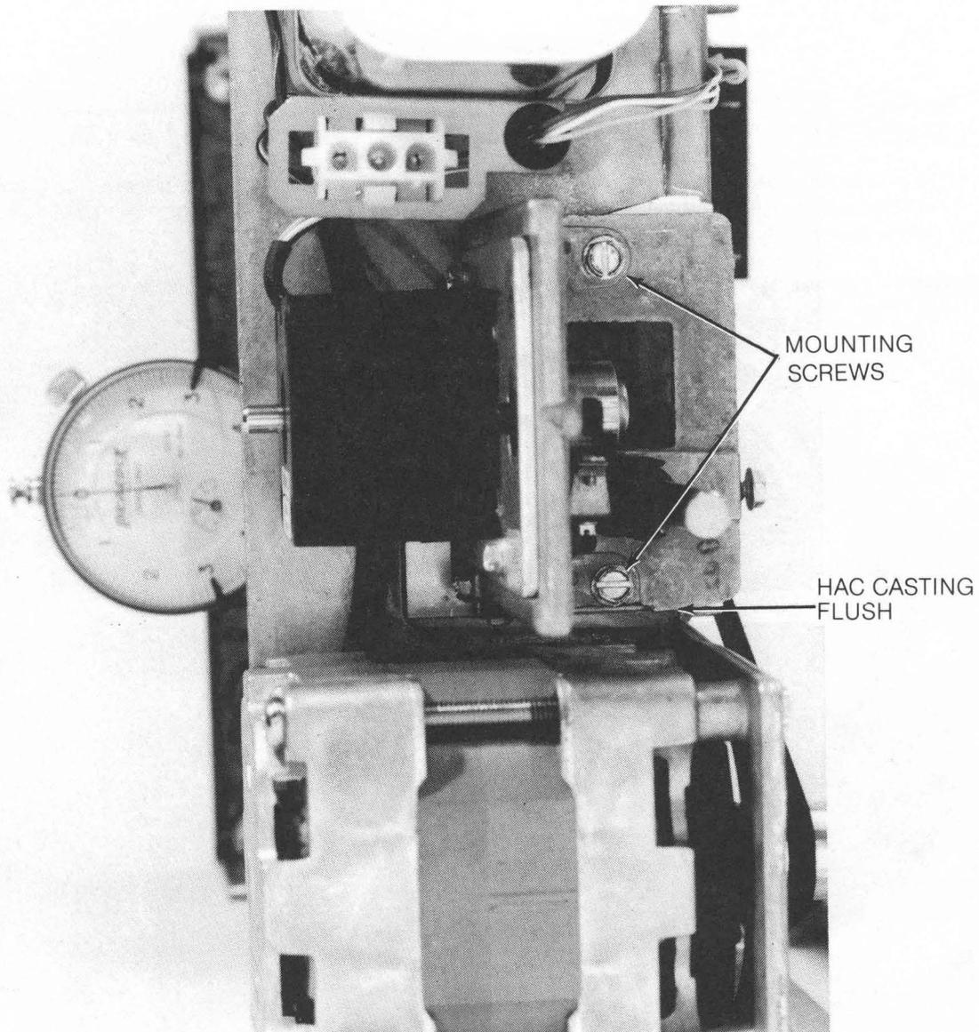
**FIGURE 44. PENETRATION ADJUSTMENT**
