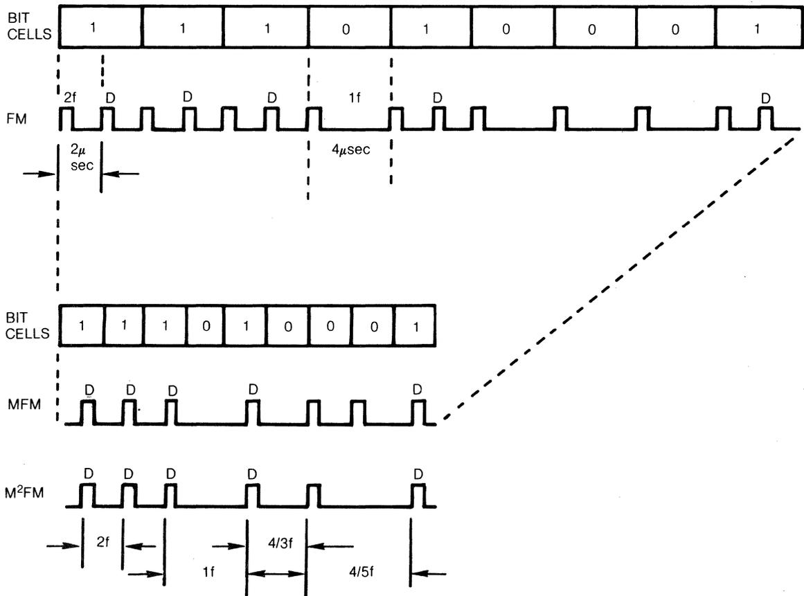
FIGURE 7. FM, MFM AND M<sup>2</sup>FM ENCODING
