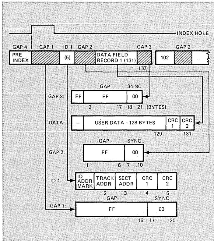
**Fig 3**—IBM format utilizes four kinds of record gaps.
