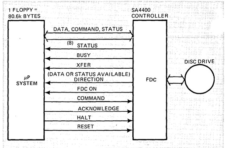
Fig 5—A typical mini-floppy controller, the Shugart SA4400, generates ten classes of signals to interface with a  $\mu P$  system.
