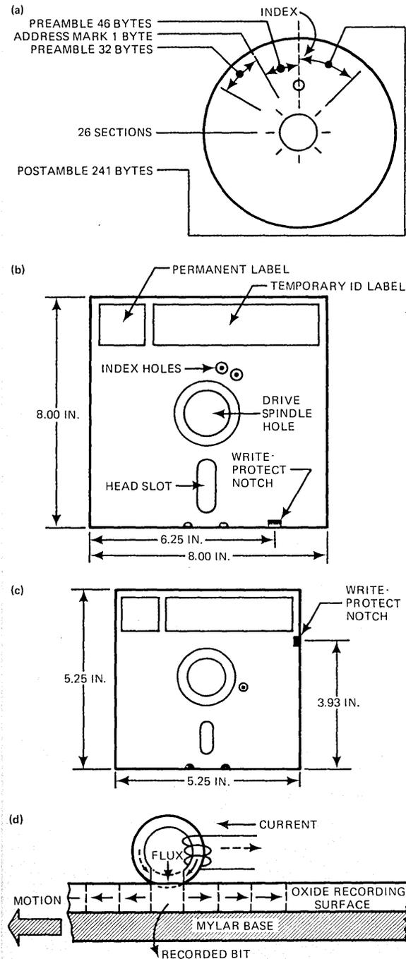
Without its protective envelope, a floppy disc (a) consists of a round platter of plastic coated with magnetic oxide and formatted in various ways. Two sizes are currently available: the full-sized disc (b) and the mini form (c). Part (d) shows a cross section of a disc to illustrate its composition and a simplified explanation of bit recording.
