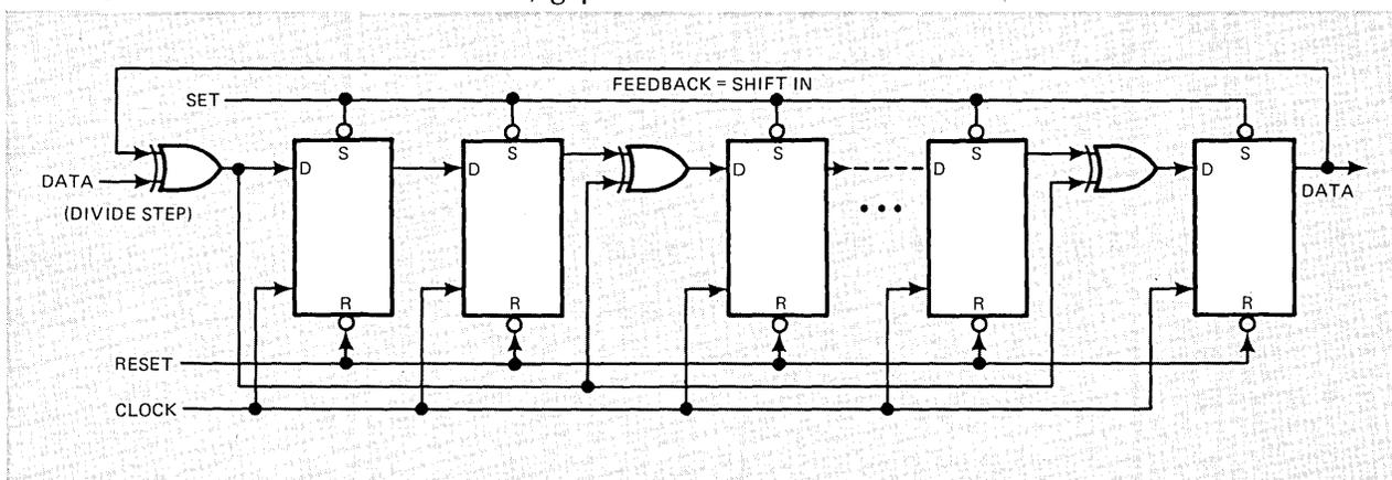
Fig 4—Flip flops and exclusive OR's generate a cyclic redundancy check. This particular circuit implements generation of the polynomial  $G(X)=X^{16}+X^{15}+X^2+1$ ; the result of dividing a bit string by this polynomial is the CRC check sum.
