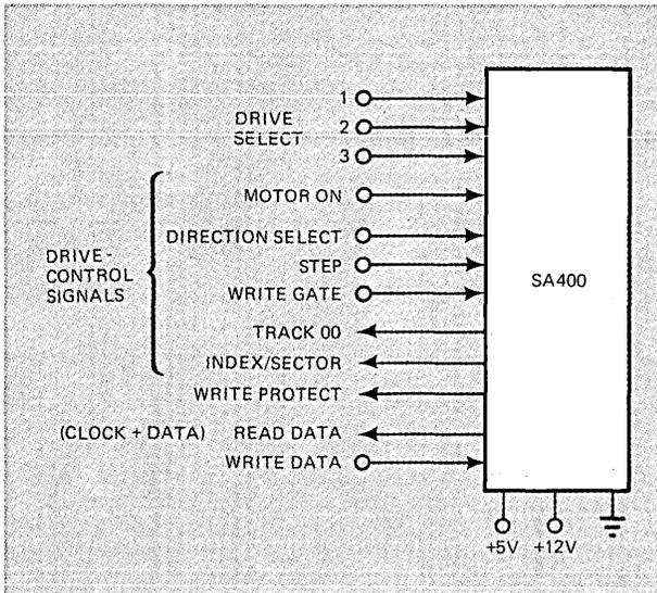
**Fig 1**—Six signals provide a floppy-disc drive's essential control functions. Additional signals select the proper drive in multidrive systems and control read/write and write-protect functions.
