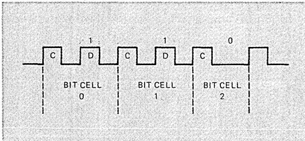
**Fig 2**—Recording method encodes both clock and data information on the same signal. Thus, each bit creates a clock pulse.
