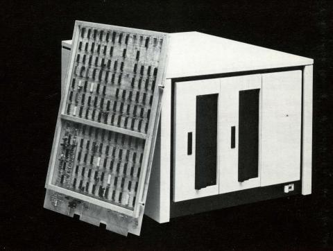
The Shugart SA8800 "Streaker" controller and SA3800 Subsystem offer the systems designer several very attractive system building blocks. The SA3800 provides a subsystem level component which shortens development time and minimizes initial program costs. Customers concerned with value added can start with the SA3800 and easily move to the Streaker as production experience with the SA3800 develops.
