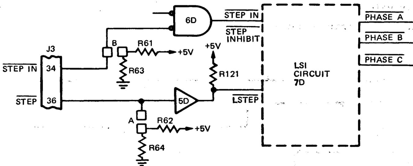
Figure 3-18. Stepper Motor Interface Gating Logic
