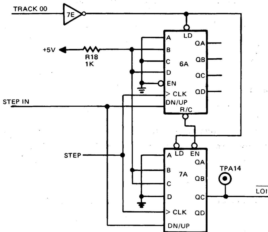
Figure 3-28. Write Current Switching
