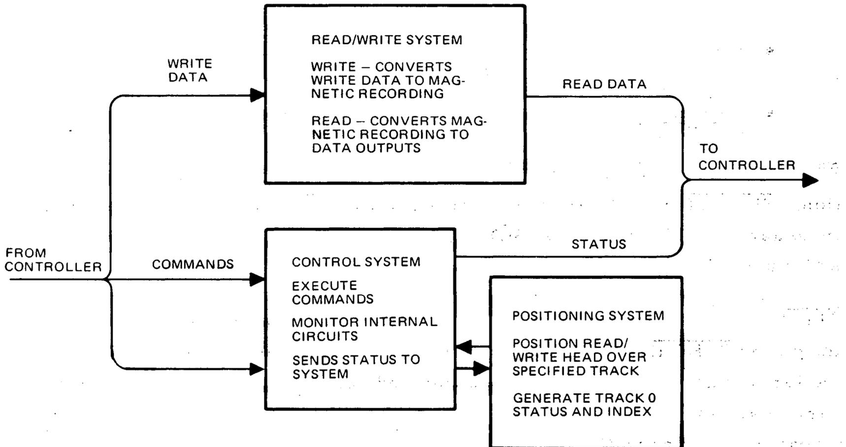
Figure 3-1. Floppy Disk Drive, Simplified Block Diagram
