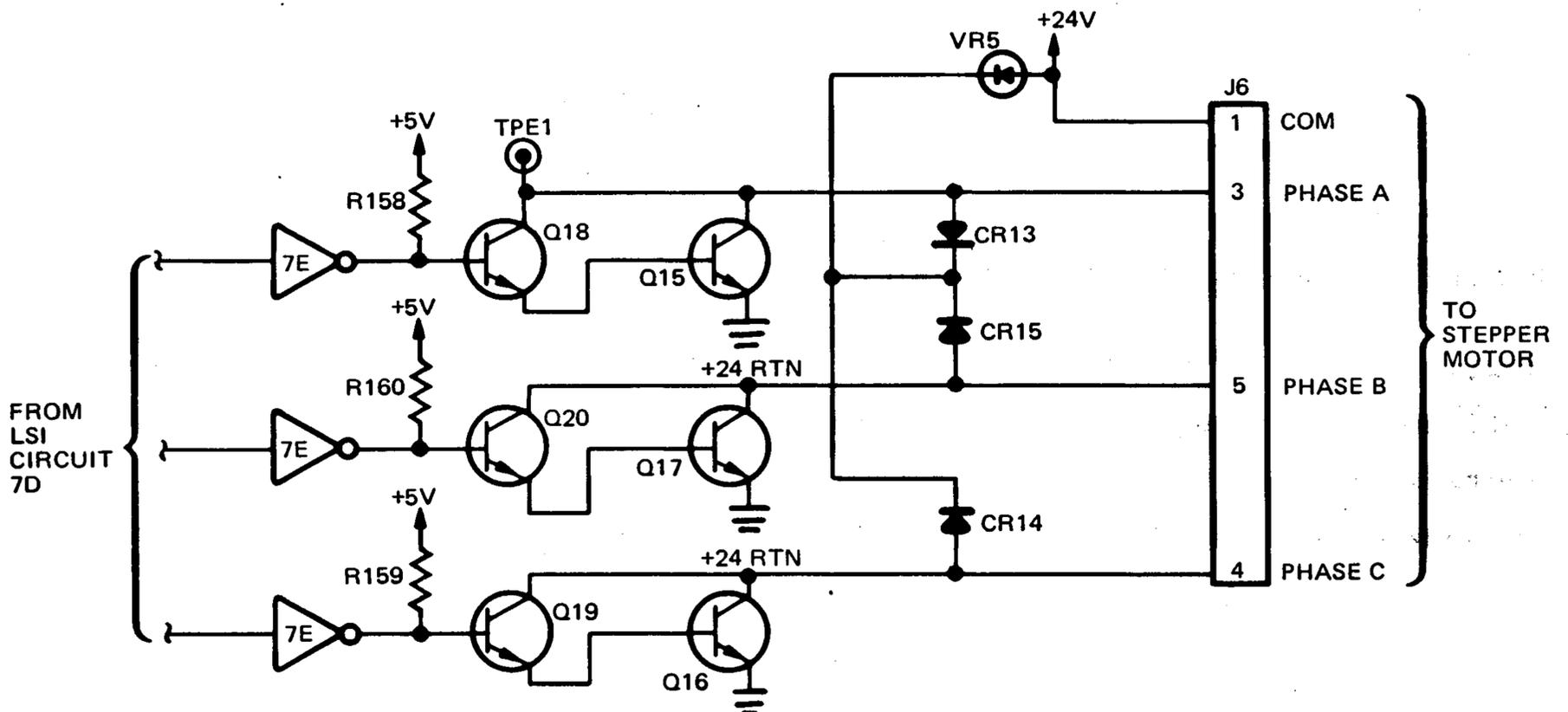
Figure 3-20. Stepper Motor Driver Circuit
