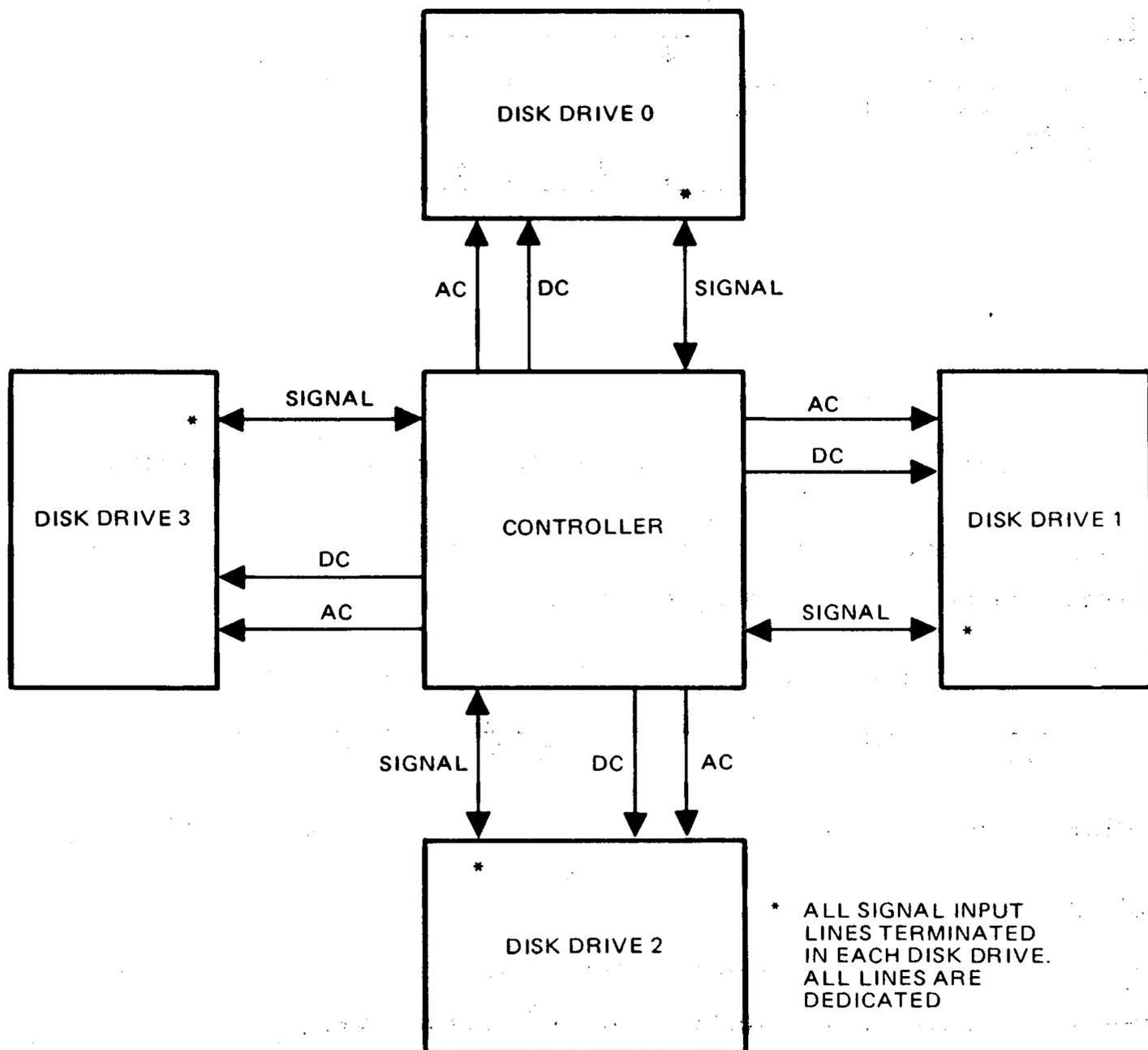
Figure 4-6. Radial Select Configuration
