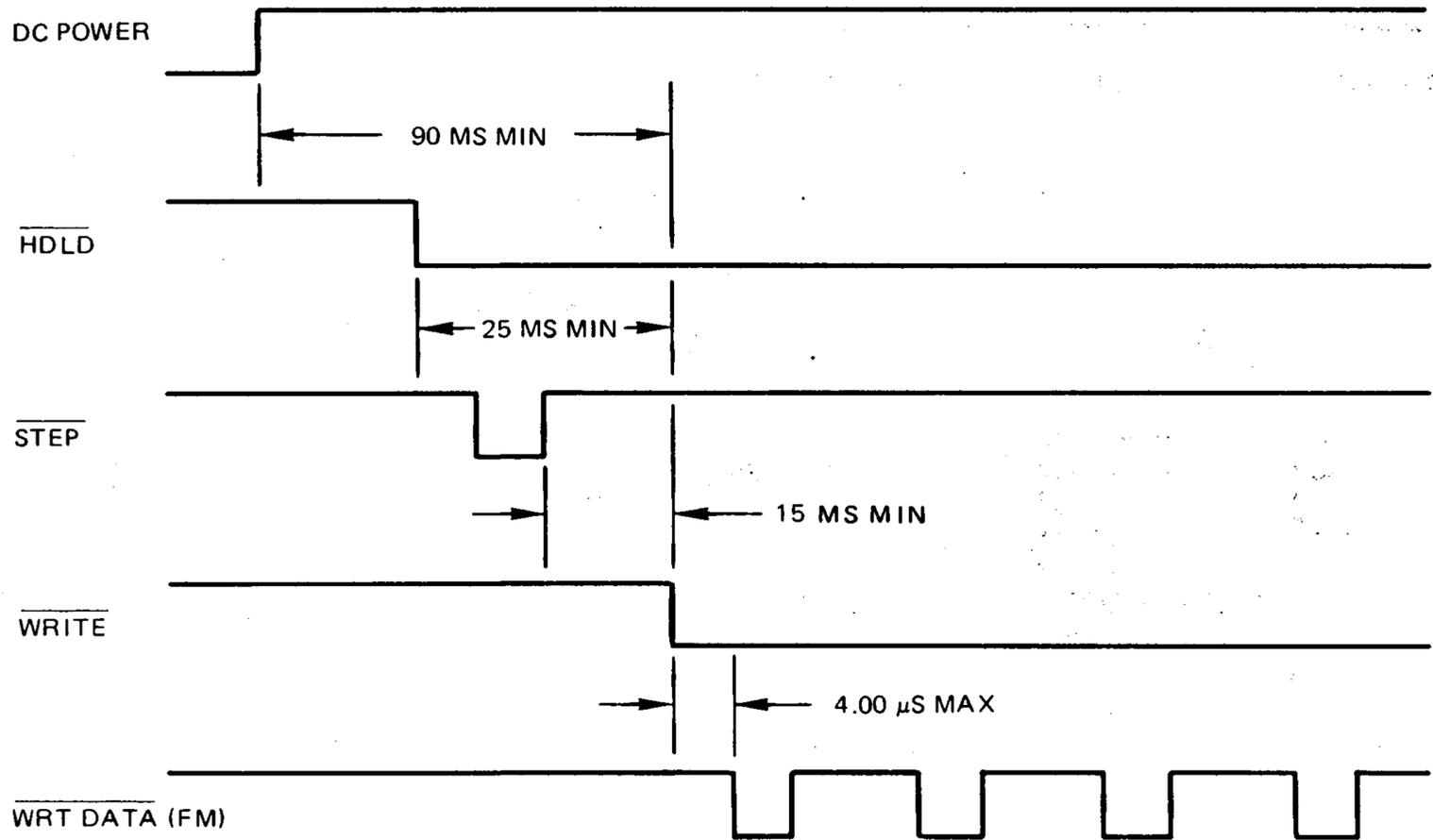
Figure 3-21. Write Initiate Timing
