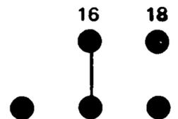
The IN USE latch can be disabled by removing the wire jumper from the vertical 4 pads.
