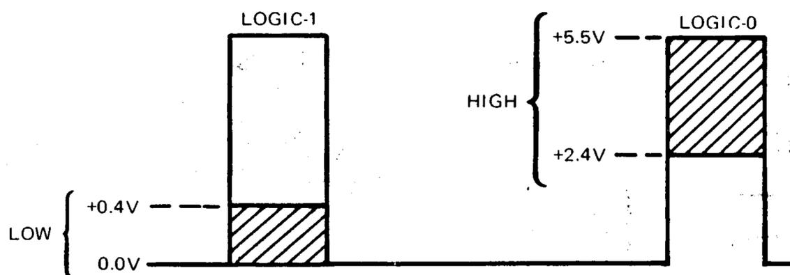
Figure 3-7. Interface Logic Levels
