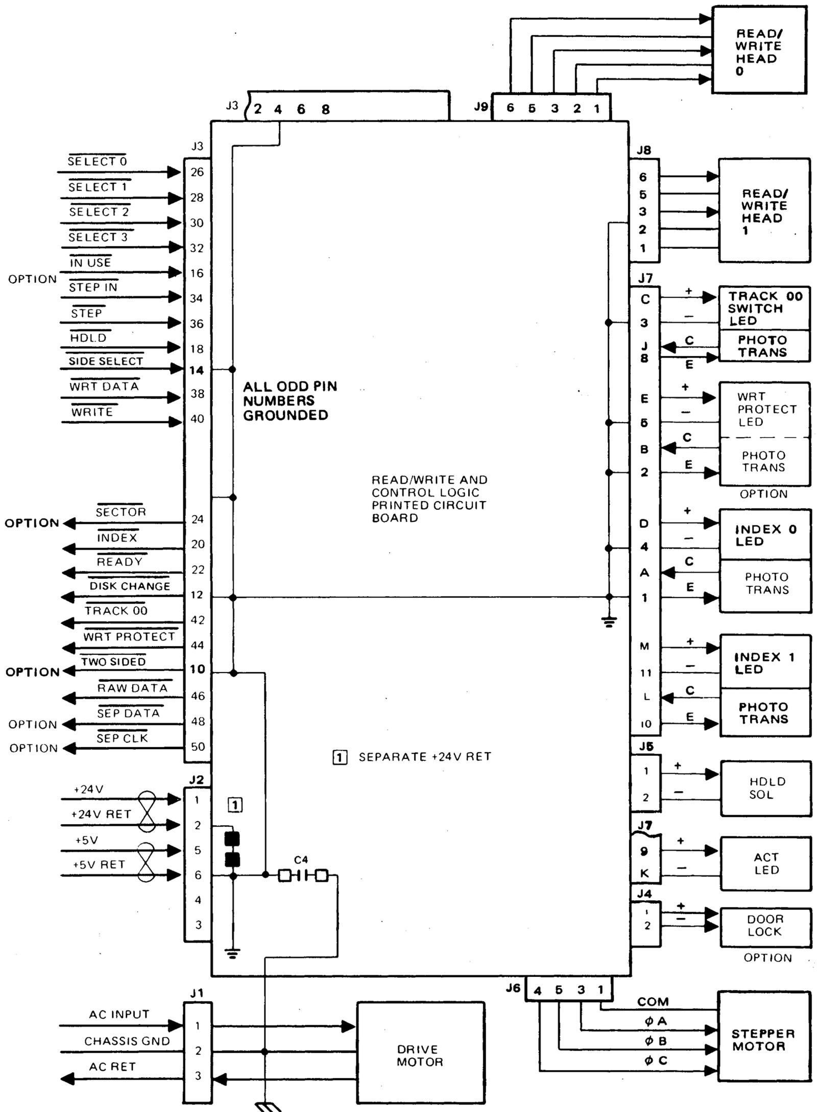
Figure 4-4. Interconnection Diagram
