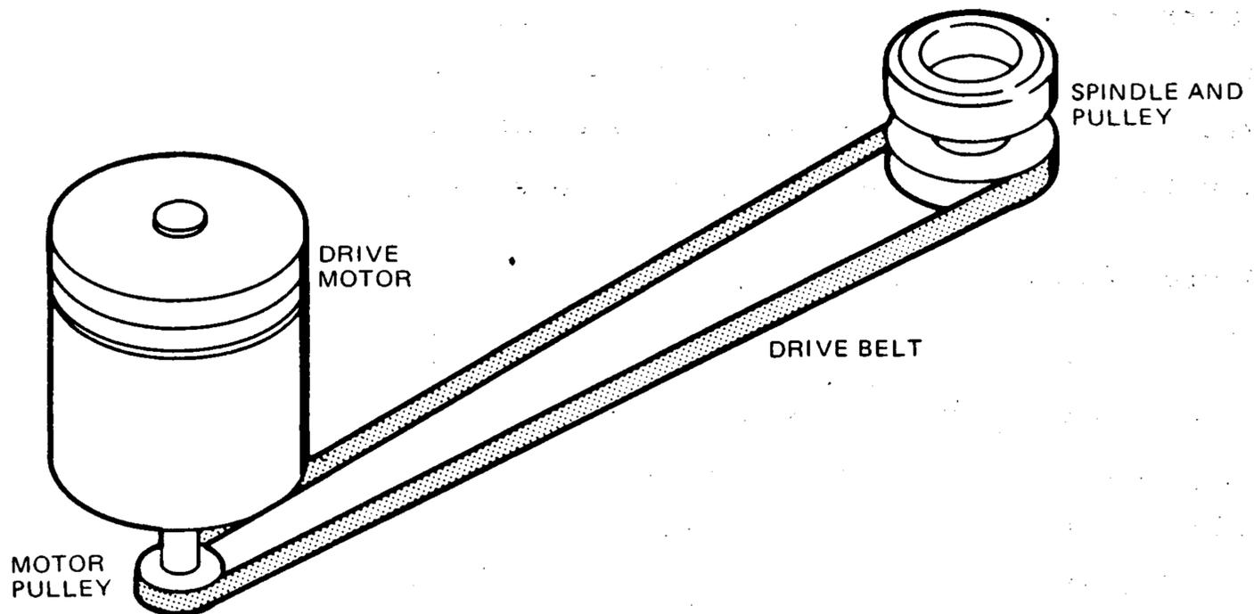
Figure 3-3. Spindle Drive System
