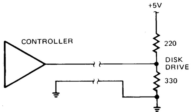
Figure 3-40. Terminating Resistor Network
