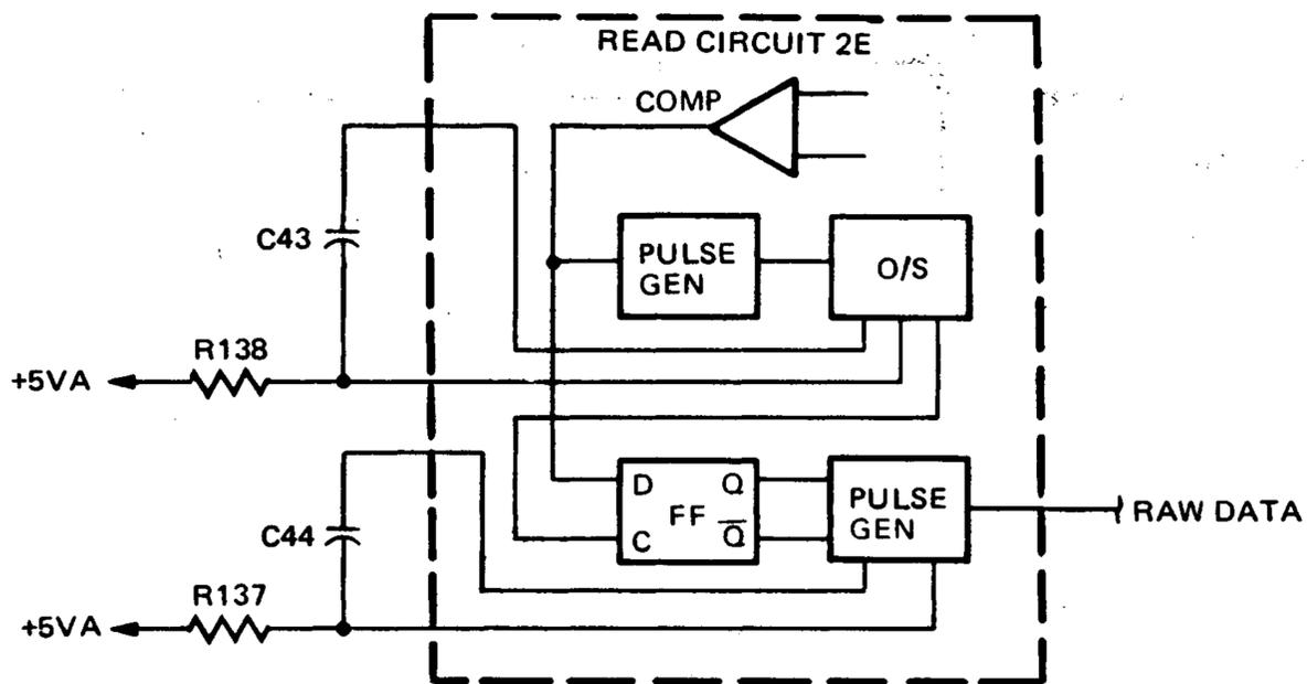
Figure 3-36. Time Domain Filter Logic
