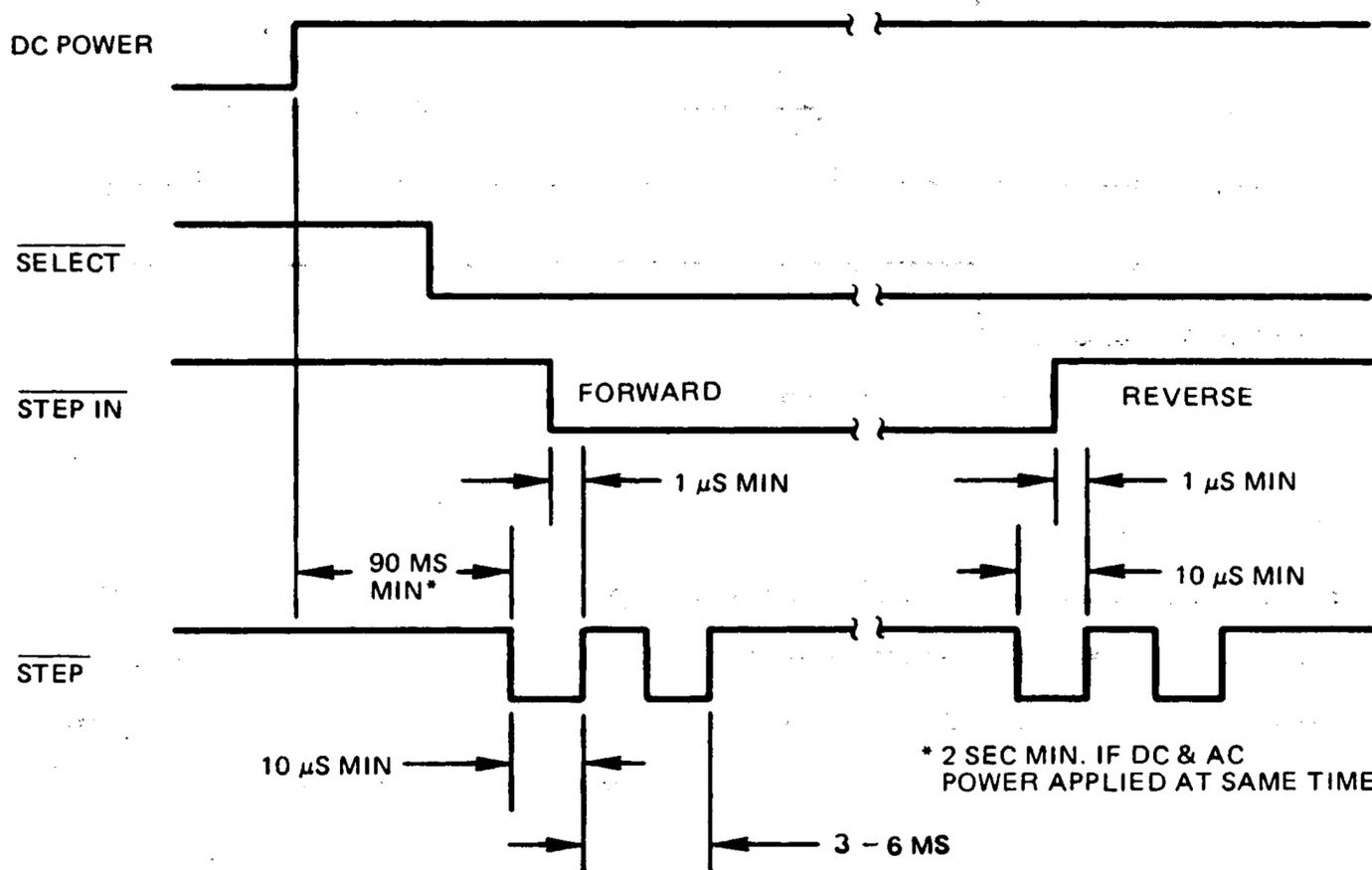
Figure 3-19. Stepper Motor Timing
