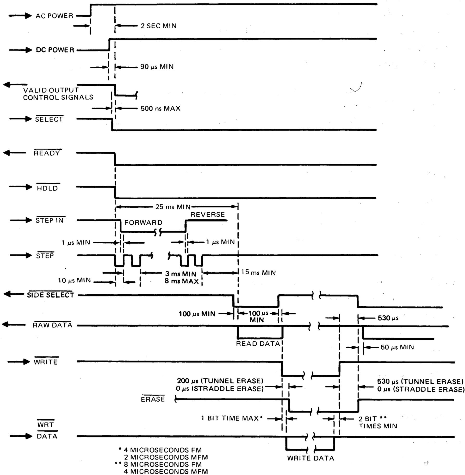
Figure 3-6. Control and Data Timing
