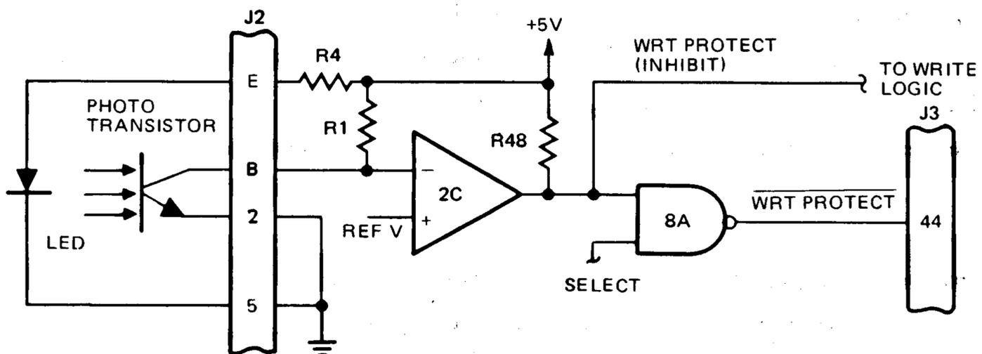
Figure 3-22. Write Protect Logic
