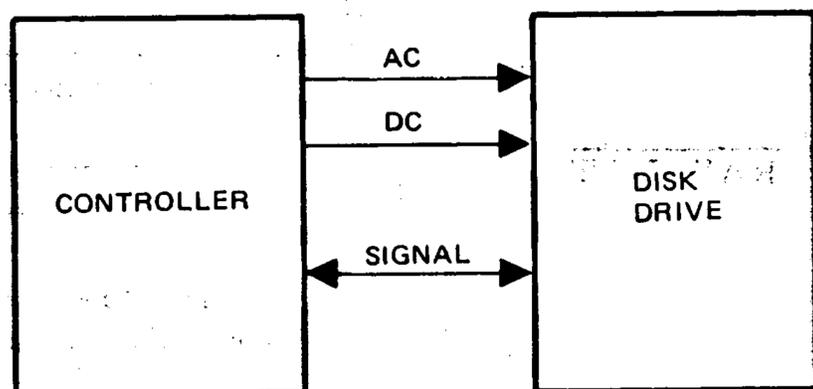
Figure 4-5. Single-Drive Configuration
