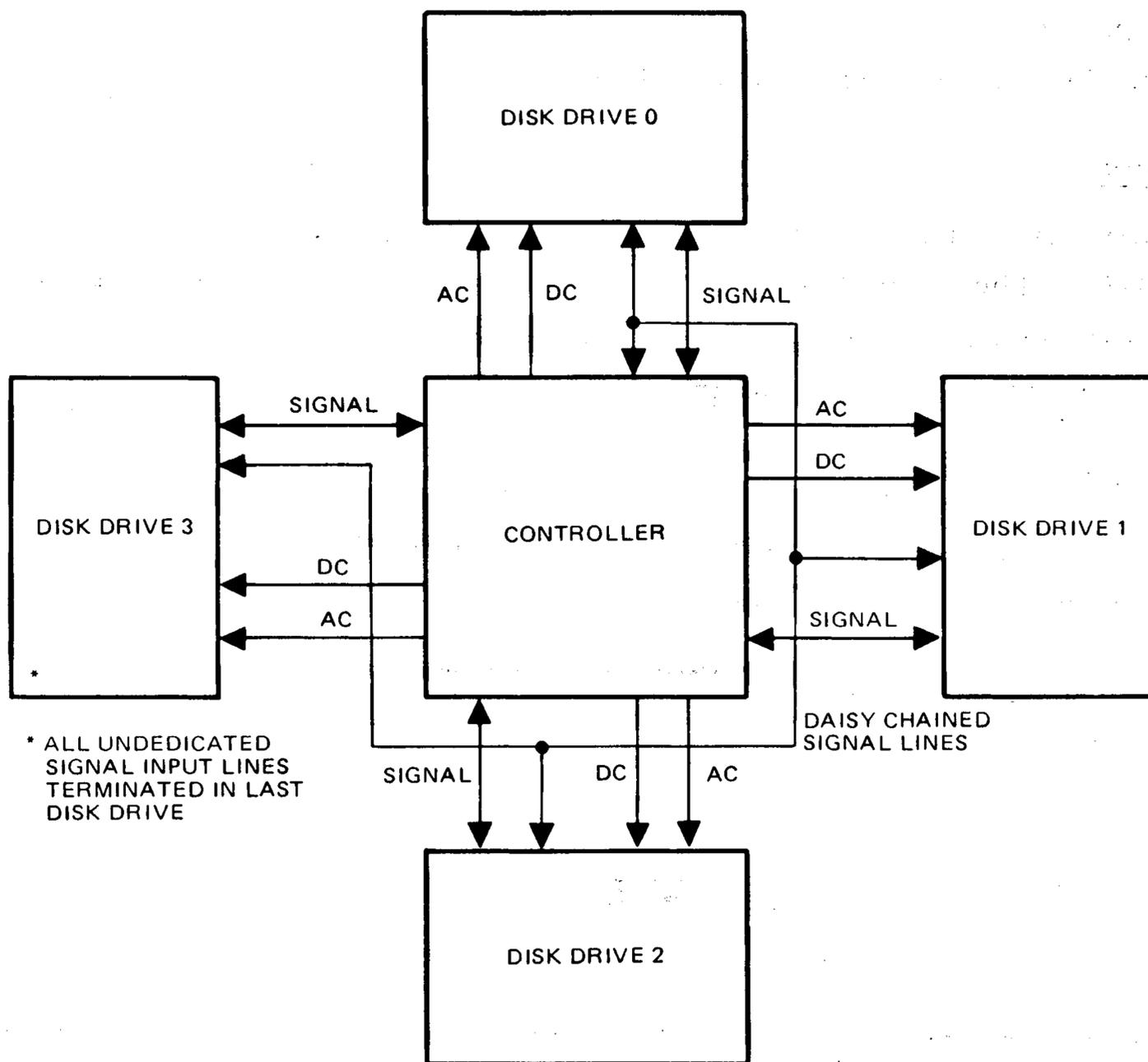
Figure 4-7. Daisy-Chained Radial Select Configuration
