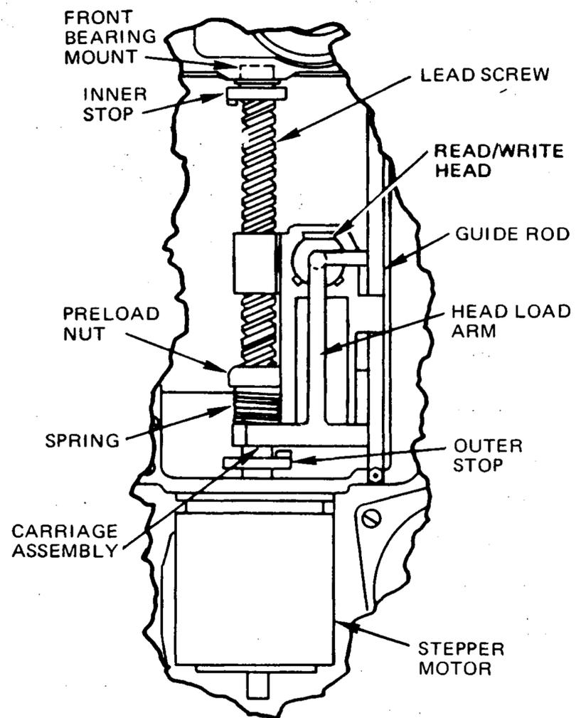
Figure 3-5. Read/Write Head Positioning System
