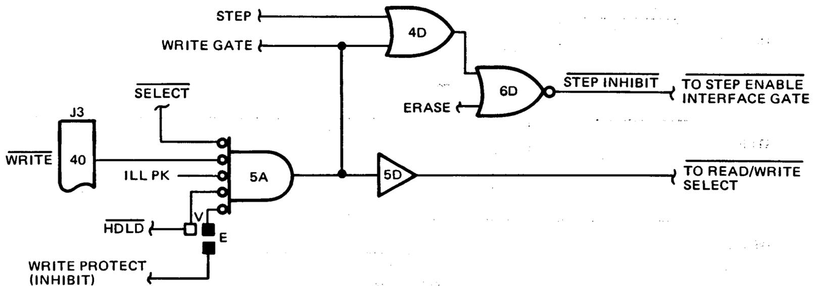
Figure 3-23. Write and Erase Gating Logic
