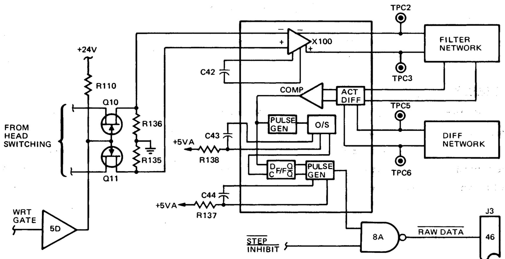
Figure 3-32. Read Logic, Simplified Diagram
