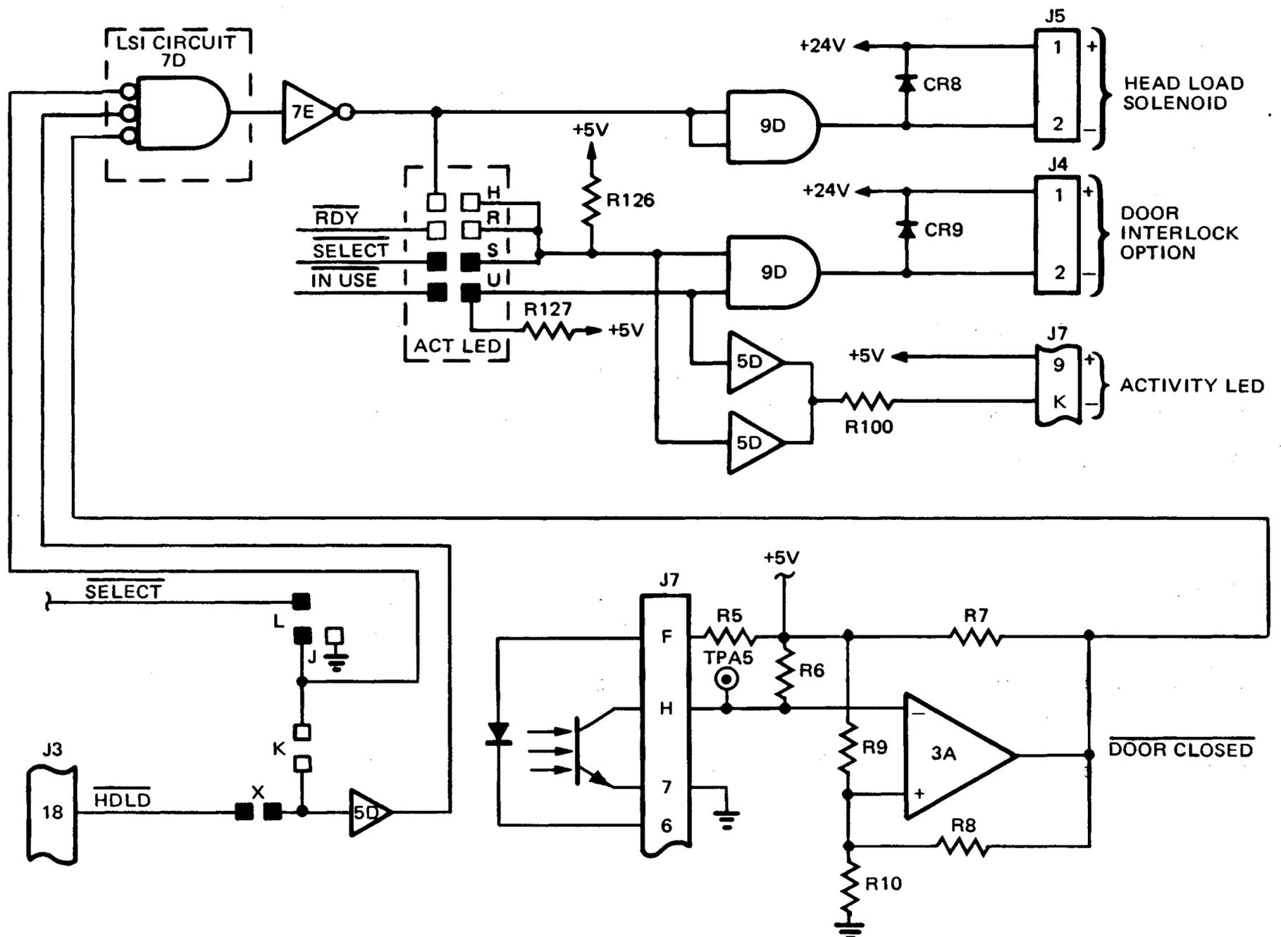
Figure 3-15. Head Load Logic
