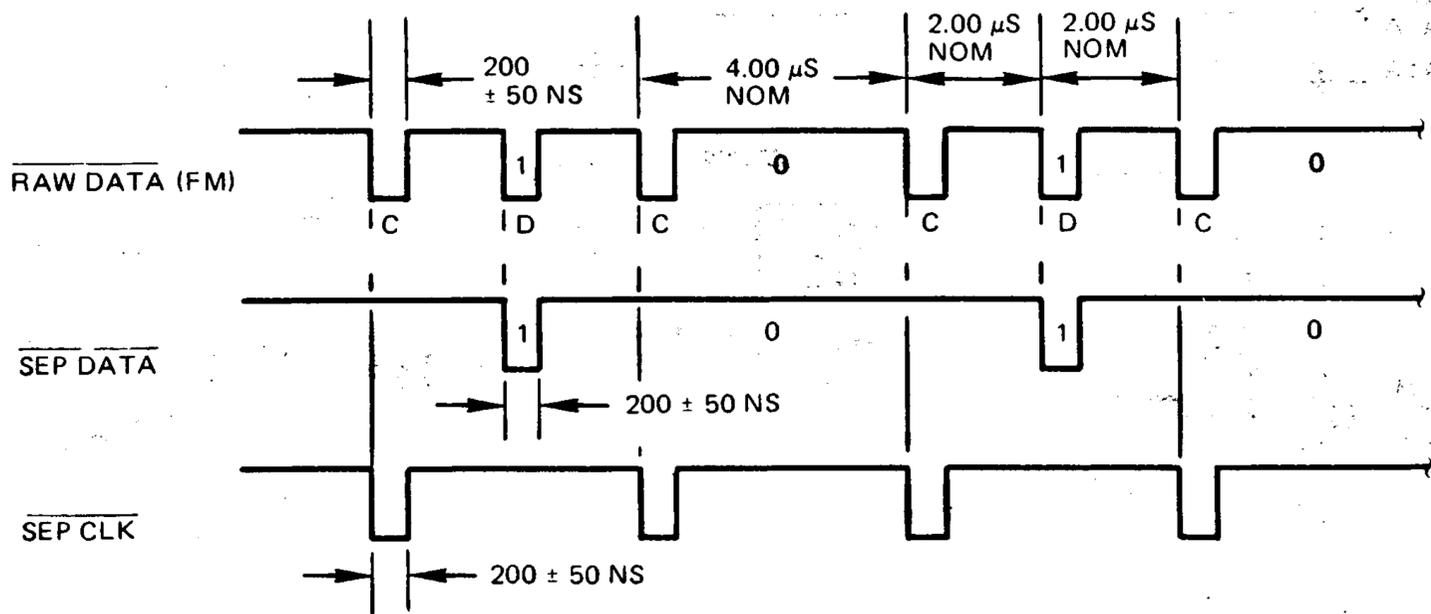
Figure 3-38. FM Data Separator Output Timing
