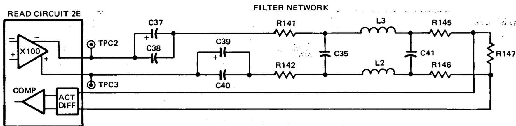
Figure 3-33. Read Preamplifier and Filter Circuit
