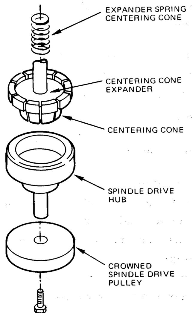
Figure 3-4. Spindle System
