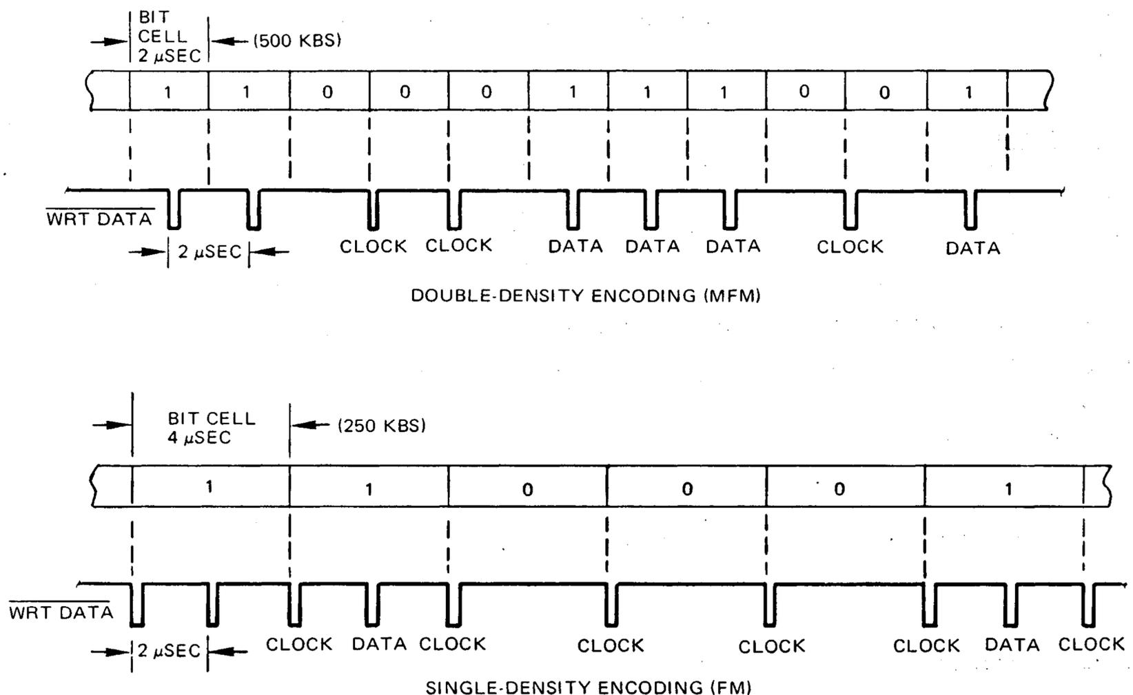
Figure 1-3. Single and Double Density Encoding
