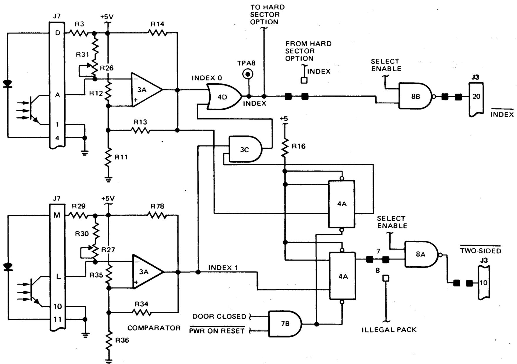
Figure 3-10. Index Detection Logic
