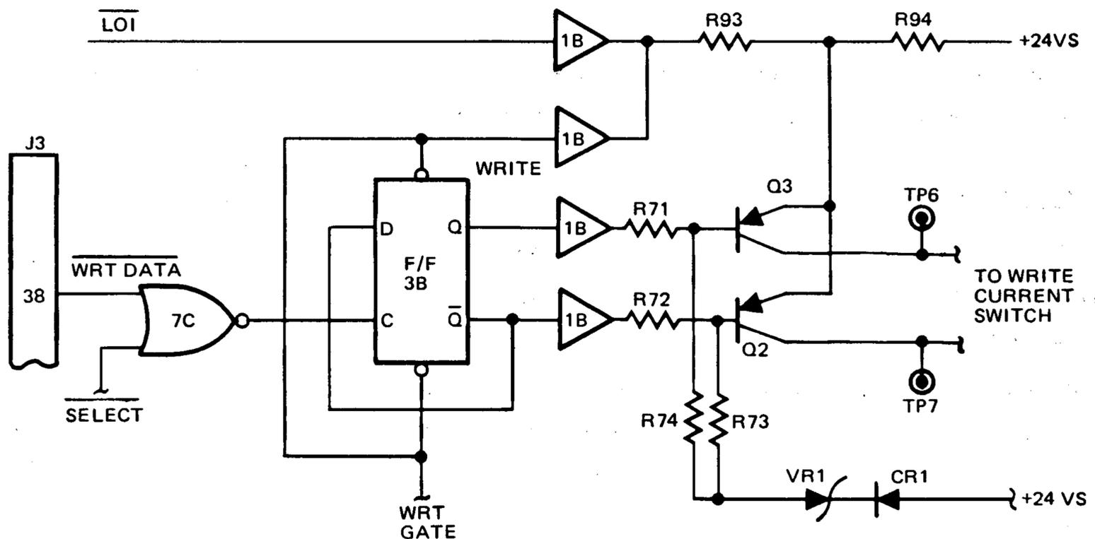
Figure 3-27. Write Current Control Logic
