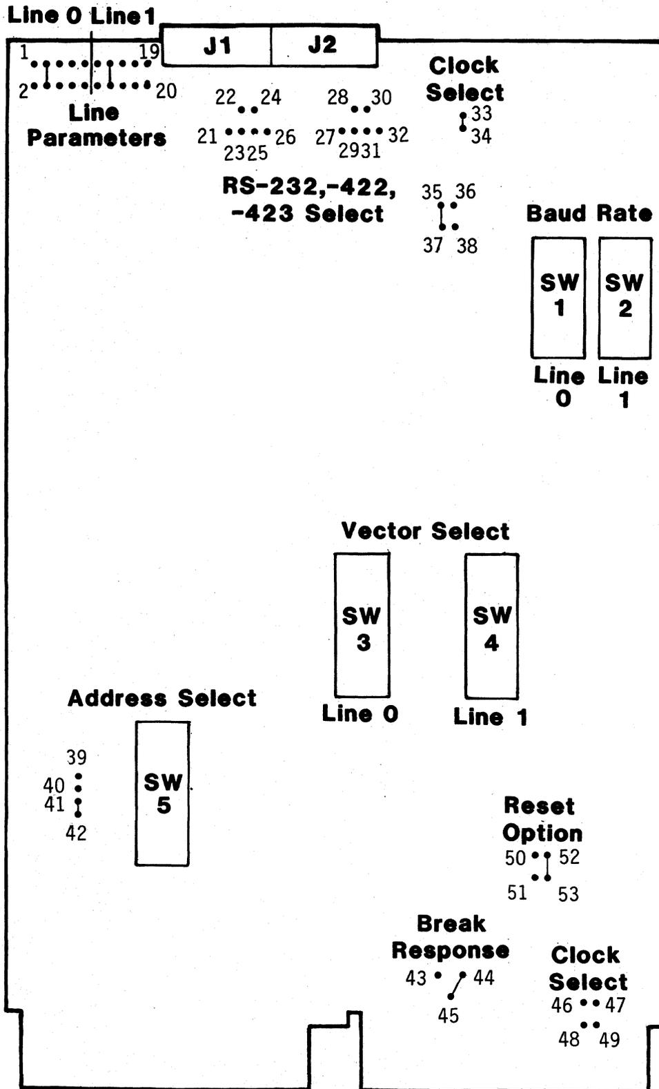
FIGURE 2-1: SWITCH AND JUMPER LOCATIONS
