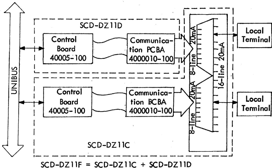
FIGURE 1-3: REQUIRED HARDWARE FOR EIA CONFIGURATIONS
