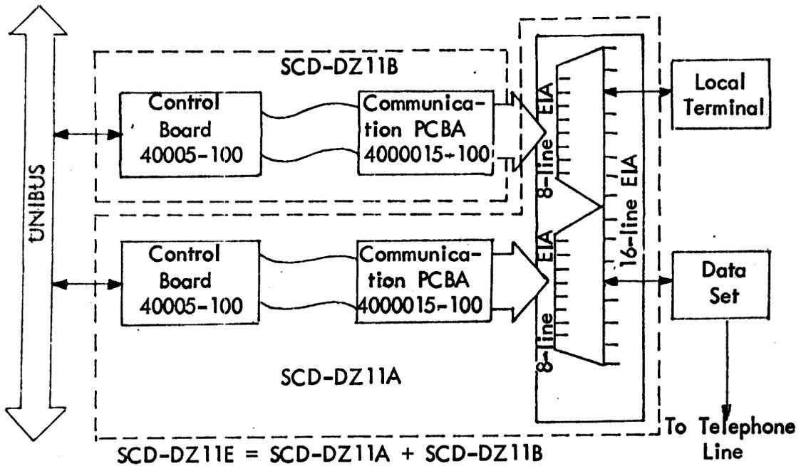
FIGURE 1-2: REQUIRED HARDWARE FOR EIA CONFIGURATIONS
