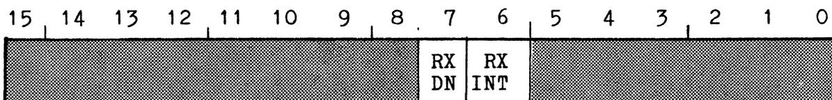
**RX DN** RECEIVER DONE. Set when an entire character has been received and is ready for input to the CPU. Cleared when RBUF is read or BINIT L signal goes true. If RX INT (bit 6) is set, setting RX DN starts an interrupt sequence. Read only.
