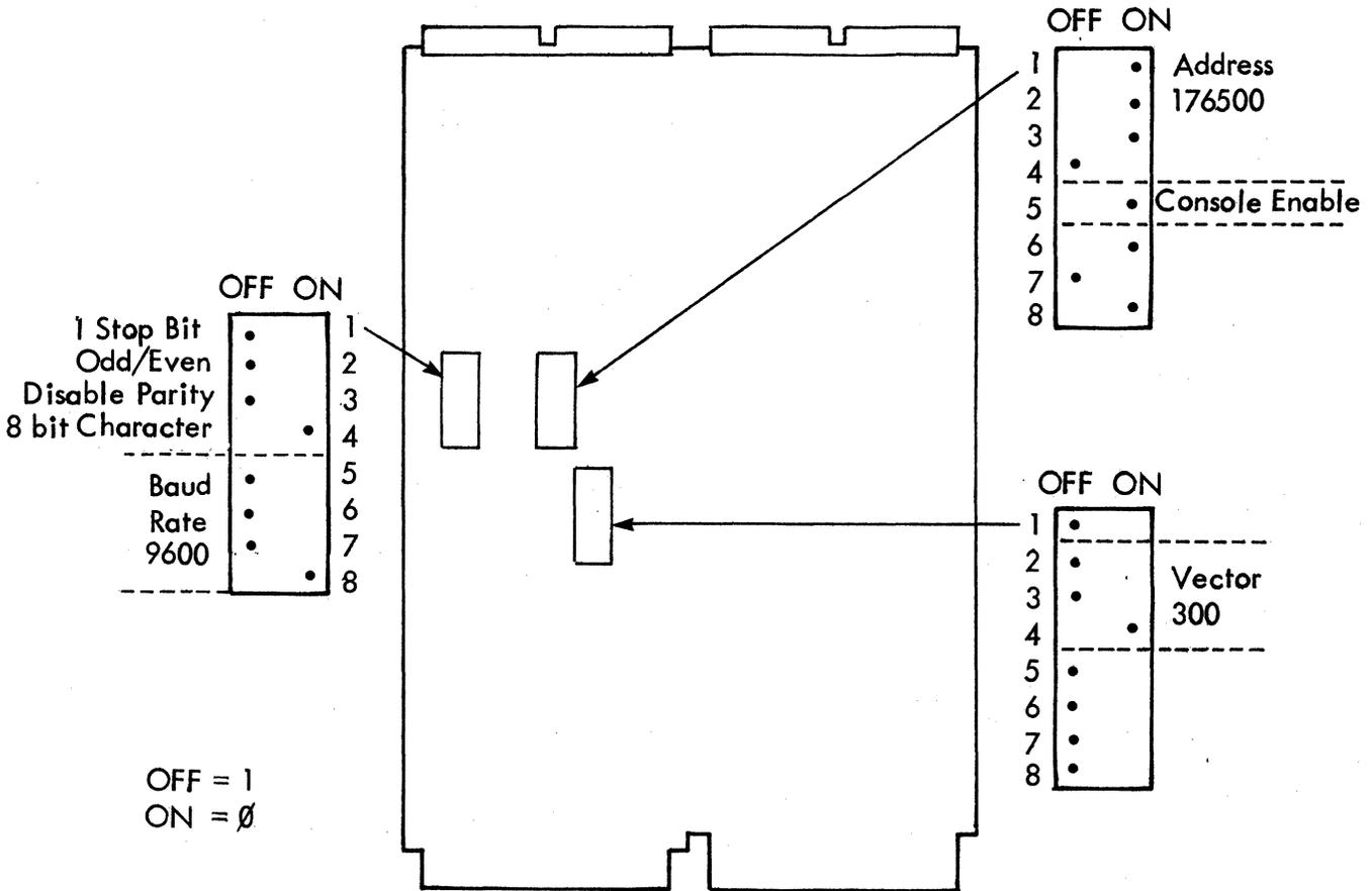
FIGURE 2-1: COMPONENT LOCATIONS SHOWING FACTORY CONFIGURATIONS
