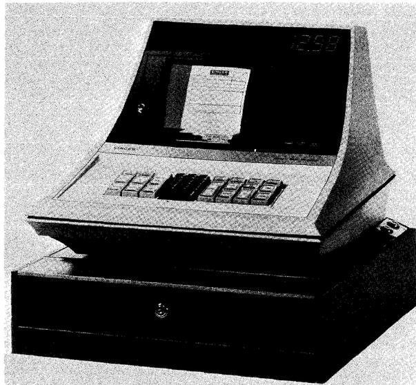
*Singer's MDTs Data Terminal, the key component of the Modular Data Transaction System, is a "computerized cash register" that can be used effectively with the System Ten in either an on-line or off-line mode.*
