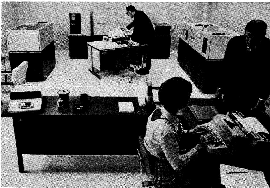
*Designed to show how the compact System Ten components fit into a normal office environment, this photo shows (from left to right) a printer, magnetic tape drive, processor, disc drive, card punch, and card reader, all clustered around a Model 70 Workstation.*
